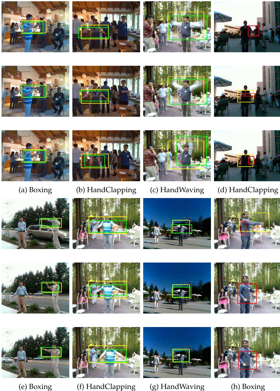
Figure 6.10: Localization results shown as a sequence of bounding boxes (MSR-II): Groundtruth is shown in yellow, correctly localized tubelets in green and false positives, missed detections (or poorly localized ones) in red. Caption below each sequence reports the class detected.
