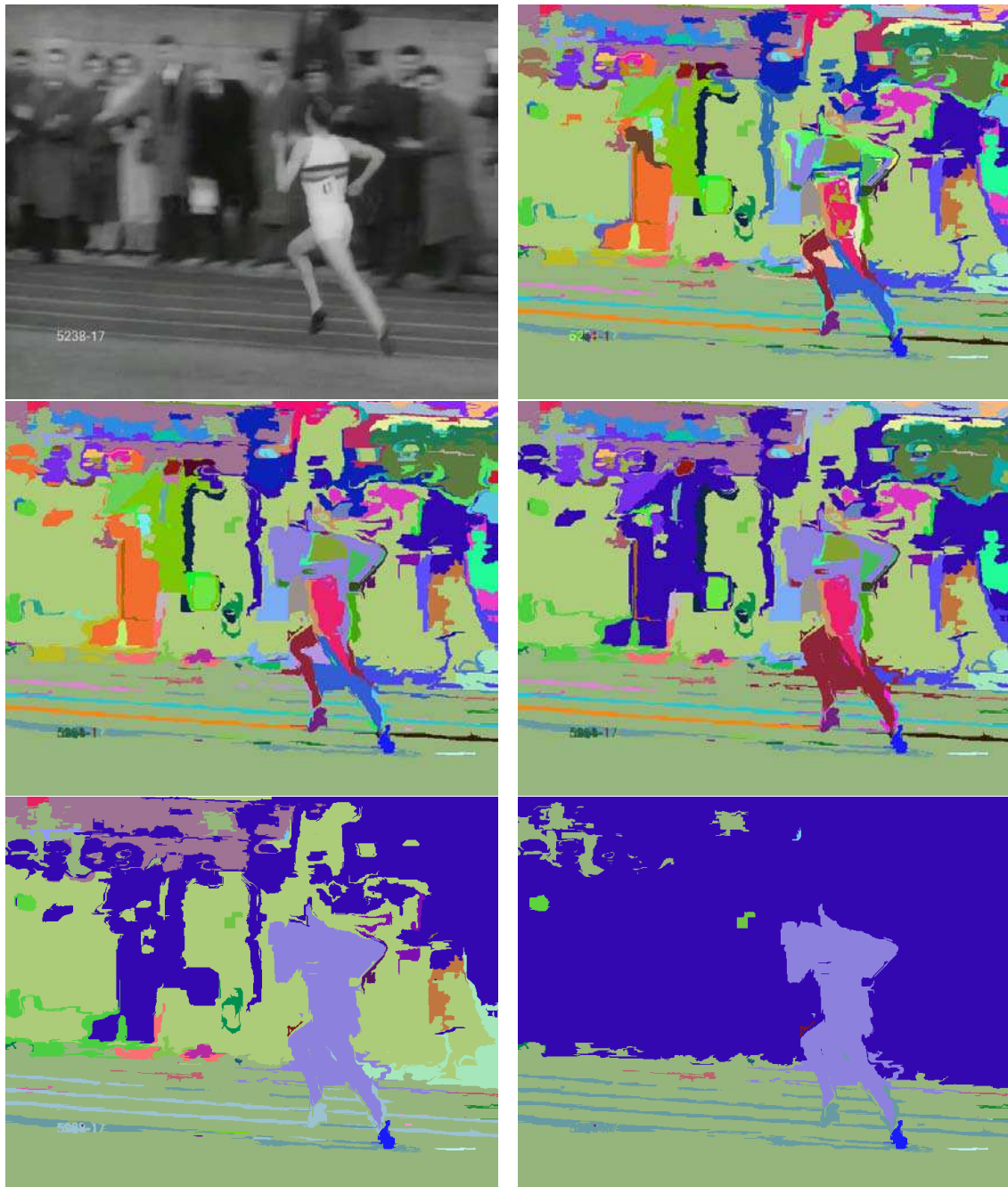
Figure 6.3: Example from action ‘Running’: The two images on the top depict a video frame and the initial super-voxel segmentation used as input of our approach. The next four images represent the segmentation after a varying number of merge operations.
