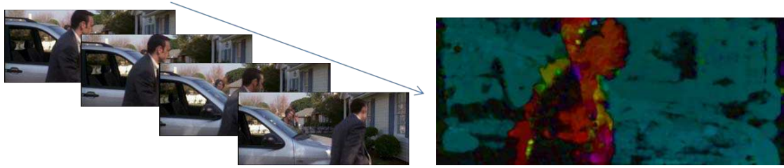
(a) Camera motion: Only person is moving but there is motion induced due to camera motion, which can be seen as optical flow in the background.
