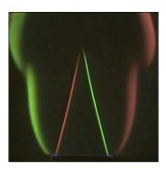
**Figure 1.12 :** Color Schlieren image of a conical methane-air premixed flame  $(\phi = 0.90, v_u = 1.50 \text{ m} \cdot \text{s}^{-1}).$
