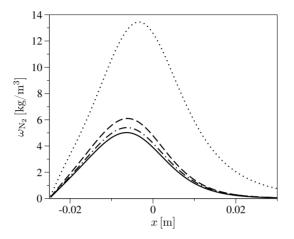
**Figure 5.9:** RVC, BRVC(50), VC and MTP model comparison. N<sub>2</sub> mass production term evolution along the axis of the EAST facility nozzle (unbroken line RVC, dashed line BRVC(50), dotted-dashed line VC, dotted line MTP).
