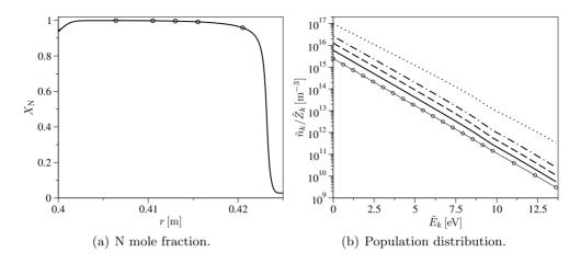
**Figure 5.22:** BRVC(20) model. Comparative evolution of the N mole fraction and the energy bin population distribution in the post-shock equilibrium area. The circles in (a) indicate the locations at which the population distributions, plotted in (b), are extracted (in (b) line with circles r = 0.421 m, unbroken line r = 0.416 m, dashed line r = 0.413 m, dotted-dashed line r = 0.411 m, dotted line r = 0.406 m).
