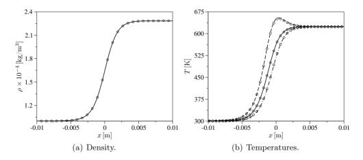
**Figure 7.15:** Flow across a normal shock wave in a Ne-Ar gas. Evolution of the gas density, temperature and related parallel and transverse components  $(M_{\infty} = 2;$  lines BEST, symbols DMSC(Torres); in (b) unbroken line T, dashed line  $T_x$ , dotted-dashed line  $T_y$ ).
