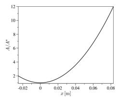
**Figure 5.2:** Normalized area distribution of the EAST facility nozzle (inlet x = -0.025 m, throat x = 0 m, outlet x = 0.083 m).
