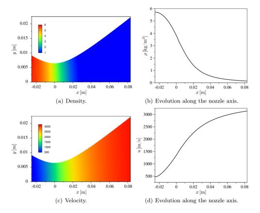
**Figure 5.29:** VC model. Density and velocity distributions within the EAST facility nozzle.
