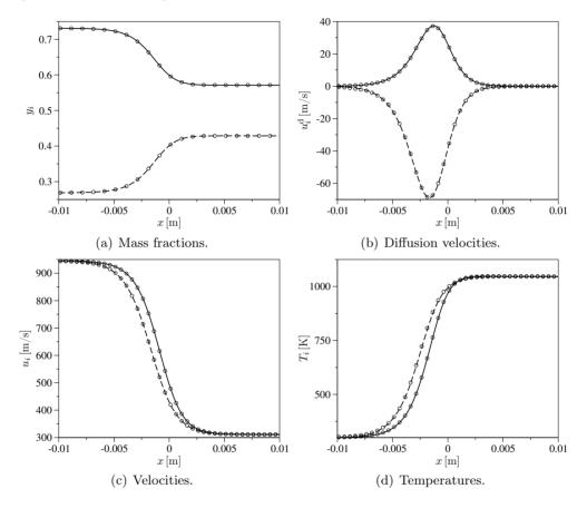
**Figure 7.18:** Flow across a normal shock wave in a multi-energy level gas. Evolution of the level mass fractions, diffusion velocities, velocities and temperatures  $(M_{\infty} = 3;$  unbroken lines level 1 BEST, dashed lines level 2 BEST, symbols DSMC(Torres)).
