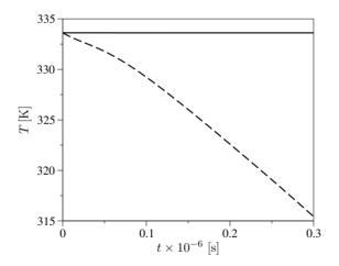
**Figure 7.13:** Isochoric equilibrium relaxation of a Ne-Ar gas. Time-evolution of the gas temperature with and without conservation constraint ( $N_c = 16$ ; unbroken line with conservation, dashed line without conservation).
