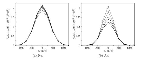
**Figure 7.11:** Isochoric equilibrium relaxation of a Ne-Ar gas. Time-evolution of the  $c_x$  axis component of the species velocity distribution functions (unbroken lines  $t = 5 \times 10^{-9}$  s, dashed lines  $t = 1.4 \times 10^{-8}$  s, dotted-dashed lines  $t = 2.4 \times 10^{-8}$  s, lines with circles  $t = 5.0 \times 10^{-8}$  s, lines with squares  $t = 1.5 \times 10^{-7}$  s).
