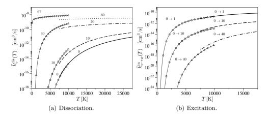
**Figure 3.7:** Comparison between the NASA ARC and U Bari databases for the vibrational dissociation and inelastic collisional excitation rate coefficients (lines NASA ARC, lines with symbols U Bari; numbers indicate the vibrational levels involved in the transitions).
