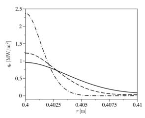
**Figure 5.19:** BRVC(20) model. Heat flux evolution along the stagnation-line for different values of the free-stream pressure (unbroken line  $p_{\infty} = 0.05$  torr, dashed line  $p_{\infty} = 0.1$  torr, dotted-dashed line  $p_{\infty} = 0.33$  torr).
