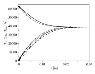
**Figure 4.13:** RVC and MT model comparison. Temperature evolution behind the shock wave switching off dissociation ( $p_{\infty} = 0.1$  torr and  $u_{\infty} = 10$  km/s; unbroken line T RVC, dashed line  $T_{\rm vib}$  RVC, dotted-dashed line  $T_{\rm rot}$  RVC, line with circles T MT, line with squares  $T_{\rm vib}$  MT, line with triangles  $T_{\rm rot}$  MT).
