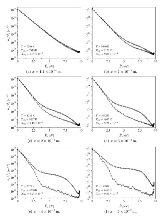
**Figure 5.11:** RVC and VC model comparison. Vibrational specific population distributions along the axis of the EAST facility nozzle (lines with circles RVC, lines with squares VC; the reported values for the  $N_2$  mole fraction, translational and vibrational temperatures refer to the RVC model solution).
