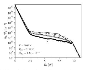
**Figure 5.17:** BRVC model. Energy bin population distribution at the location  $x = 2.85 \times 10^{-1}$  m along the axis of the Scirocco nozzle for different numbers of energy bins (unbroken line BRVC(5), dashed line BRVC(10), dotted line BRVC(20), dotted-dashed line BVVC(50), circles BRVC(100), triangles BRVC(500); the reported values for the N<sub>2</sub> mole fraction, translational and internal temperatures refer to the BRVC(50) model solution).
