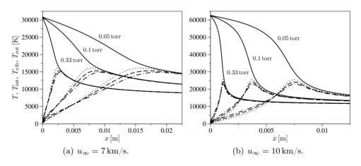
**Figure 4.1:** *RVC* model. Temperature evolution behind the shock wave for different values of the free-stream pressure (unbroken lines T, dashed lines  $T_{int}$ , dotted-dashed lines  $T_{vib}$ , dotted lines  $T_{rot}$ ).
