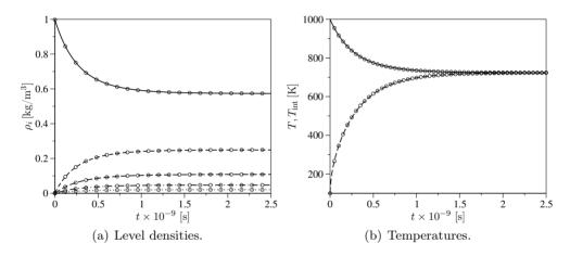
**Figure 7.17:** Isochoric equilibrium relaxation of a multi-energy level gas. Timeevolution of the level densities and temperatures (lines BEST, symbols DSMC(Torres); in (a) unbroken line  $\rho_1$ , short dashed line  $\rho_2$ , long dashed line  $\rho_3$ , dotted-dashed dashed line  $\rho_4$ , dotted line  $\rho_5$ ; in (b) unbroken line T, dashed line  $T_{int}$ ).
