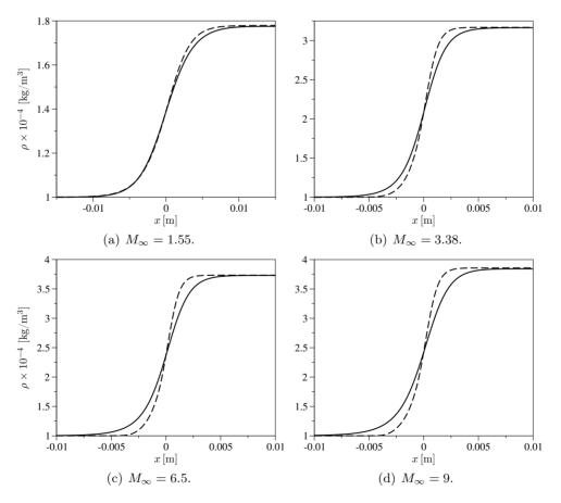
**Figure 7.9:** Flow across a normal shock wave in Ar. Comparison of the density profiles obtained by solving the Boltzmann and the Navier-Stokes equations for different values of the free-stream Mach number (unbroken lines BEST, dashed lines NS).
