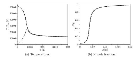
**Figure 4.5:** RVC model. Temperature and N mole fraction evolution behind the shock wave with/without predissociation ( $p_{\infty} = 0.1$  torr and  $u_{\infty} = 10$  km/s; in (a) unbroken line T with predissociation, dashed line  $T_{\text{int}}$  with predissociation, dotted-dashed line T without predissociation, dotted line  $T_{\text{int}}$  without predissociation; in (b) unbroken line with predissociation, dashed line without predissociation).
