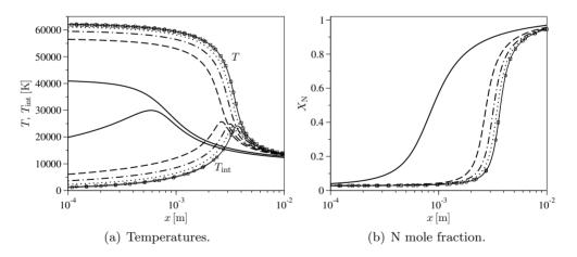
**Figure 4.17:** BRVC model. Bin number convergence study on the temperatures and the N mole fraction for the flow behind a normal shock wave ( $p_{\infty} = 0.1$  torr and  $u_{\infty} = 10$  km/s; unbroken lines BRVC(2), dashed lines BRVC(5), dotted-dashed lines BRVC(10), dotted lines BVRC(20), lines with circles BRVC(50), lines with squares BRVC(100)).
