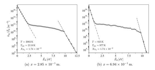
**Figure 5.15:** BRVC(50) model. Energy bin population distributions at the locations  $x = 2.85 \times 10^{-1}$  m and  $x = 6.94 \times 10^{-1}$  m along the axis of the Scirocco nozzle (the dashed and the dotted-dashed lines indicate the Boltzmann distributions at the translational and internal temperature, respectively).
