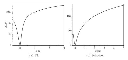
**Figure 5.12:** Normalized area distributions of the F4 and Scirocco nozzles (in (a) inlet x = -0.5 m, throat x = 0 m, outlet x = 3 m; in (b) inlet x = -0.28 m, throat x = 0 m, outlet x = 5 m).
