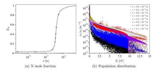
**Figure 4.6:** RVC model. Comparative evolution of the N mole fraction and rovibrational energy level distribution behind the shock wave  $(p_{\infty} = 0.1 \text{ torr } and u_{\infty} = 10 \text{ km/s};$  the symbols in (a) highlight the locations at which the population distributions, plotted in (b), are extracted).
