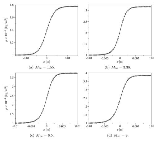
**Figure 7.1:** Flow across a normal shock wave in Ar. Density evolution for different values of the free-stream Mach number (lines BEST, symbols DSMC(Torres)).
