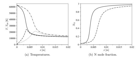
**Figure 4.4:** RVC model. Temperature and N mole fraction evolution behind the shock wave with/without exchange processes ( $p_{\infty} = 0.1$  torr and  $u_{\infty} = 10$  km/s; in (a) unbroken line T with exchange, dashed line  $T_{\text{int}}$  with exchange, dotted-dashed line T without exchange; in (b) unbroken line with exchange, dashed line without exchange.
