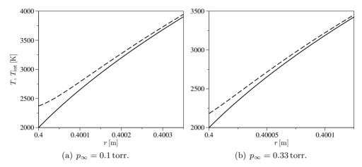
**Figure 5.20:** BRVC(20) model. Translational and internal temperature profiles within the boundary layer for different values of the free-stream pressure (unbroken lines T, dashed lines  $T_{int}$ ).
