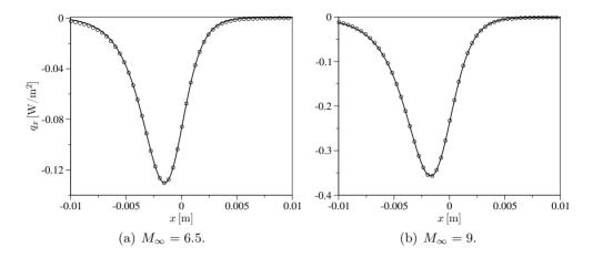
**Figure 7.3:** Flow across a normal shock wave in Ar. Heat flux evolution for different values of the free-stream Mach number (lines BEST, symbols DSMC(Torres)).
