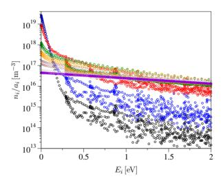
**Figure 4.7:** RVC model. Evolution behind the shock wave of the population of the rovibrational energy levels lying close to the ground-state ( $p_{\infty} = 0.1$  torr and  $u_{\infty} = 10 \text{ km/s}$ ; the locations at which the distributions are plotted are the same as those of fig. 4.6).
