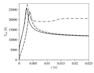
**Figure 4.18:** BRVC and URVC models. Internal temperature evolution behind the shock wave for different numbers of energy bins ( $p_{\infty} = 0.1$  torr and  $u_{\infty} = 10$  km/s; unbroken line BRVC(5), dashed line BRVC(50), dotted-dashed line URVC(5), dotted line URVC(50)).
