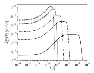
**Figure 4.14:** *RVC model. Time evolution of the macroscopic dissociation rate coefficient (unbroken line*  $T = 10\,000\,\text{K}$ *, dashed line*  $T = 15\,000\,\text{K}$ *, dotted-dashed line*  $T = 20\,000\,\text{K}$ *, line with circles*  $T = 30\,000\,\text{K}$ *, line with squares*  $T = 40\,000\,\text{K}$ *).*
