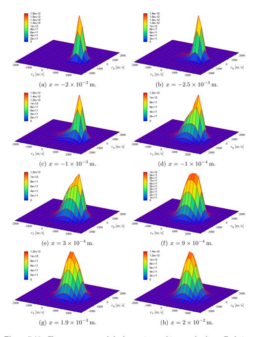
**Figure 7.22:** Flow across a normal shock wave in a multi-energy level gas. Evolution of the projection on the  $(c_x, c_y)$  plane of the velocity distribution function of level 2  $(M_{\infty} = 3)$ .
