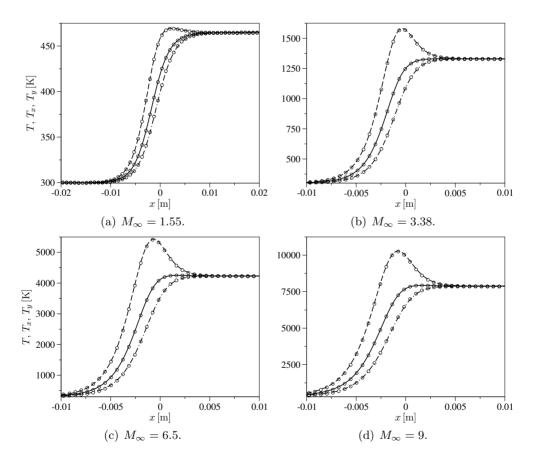
Figure 7.2: Flow across a normal shock wave in Ar. Temperature evolution for different values of the free-stream Mach number (unbroken lines T BEST, dashed lines  $T_x$  BEST, dotted-dashed lines  $T_y$  BEST, symbols DSMC(Torres)).
