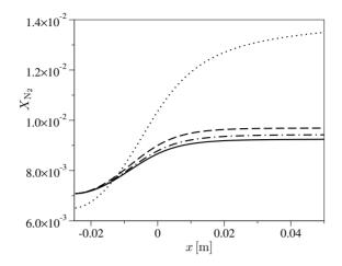
**Figure 5.8:** RVC, BRVC(50), VC and MTP model comparison. N<sub>2</sub> mole fraction evolution along the axis of the EAST facility nozzle (unbroken line RVC, dashed line BRVC(50), dotted-dashed line VC, dotted line MTP).
