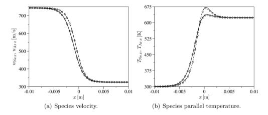
**Figure 7.14:** Flow across a normal shock wave in a Ne-Ar gas. Evolution of the species hydrodynamic velocity and parallel temperature  $(M_{\infty} = 2; unbroken lines Ne BEST, dashed line Ar BEST, symbols DSMC(Torres)).$
