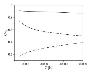
**Figure 3.6:** Chemistry coupling factors (unbroken line  $C_{N_2}^{dis-int}$ , dashed line  $C_{N_2}^{dis-vib}$ , dotted-dashed line  $C_{N_2}^{dis-vic}$ ).
