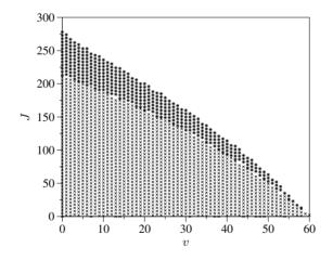
**Figure 3.1:** Rotational structure of the vibrational levels of  $N_2(^{1}\Sigma_g^{+})$  (one level over four is plotted; crosses bound levels, stars predissociated levels).
