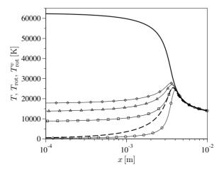
**Figure 4.9:** RVC model. Translational and rotational temperature evolution behind the shock wave ( $p_{\infty} = 0.1$  torr and  $u_{\infty} = 10$  km/s; unbroken line T, dashed line  $T_{rot}$ , line with circles  $T_{rot}^{0}$ , line with squares  $T_{rot}^{1}$ , line with triangles  $T_{rot}^{2}$ , line with diamonds  $T_{rot}^{3}$ ).
