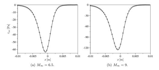
Figure 7.4: Flow across a normal shock wave in Ar. Normal viscous stress evolution for different values of the free-stream Mach number (lines BEST, symbols DSMC(Torres)).
