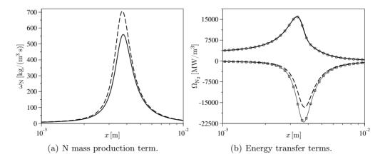
**Figure 4.16:** RVC and BRVC(50) model comparison. Mass production and energy transfer term evolution behind the shock wave ( $p_{\infty} = 0.1$  torr and  $u_{\infty} = 10$  km/s; in (a) unbroken line RVC, dashed line BRVC(50); in (b) unbroken line  $\Omega_{N_2}^{\text{tra-int}}$  RVC, dashed line  $\Omega_{N_2}^{\text{tra-int}}$  RVC, line with circles  $\Omega_{N_2}^{\text{tra-int}}$  BRVC(50), line with squares  $\Omega_{N_2}^{\text{dis-int}}$  BRVC(50)).
