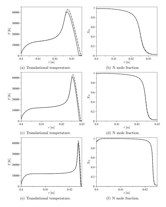
**Figure 5.27:** BRVC model. Translational temperature and N mole fraction evolution along the stagnation-line for different numbers of energy bins ((a)-(b)  $p_{\infty} = 0.05$  torr , (c)-(d)  $p_{\infty} = 0.1$  torr, (e)-(f)  $p_{\infty} = 0.33$  torr; unbroken lines BRVC(10), dotted lines BRVC(20), dashed lines BRVC(100)).
