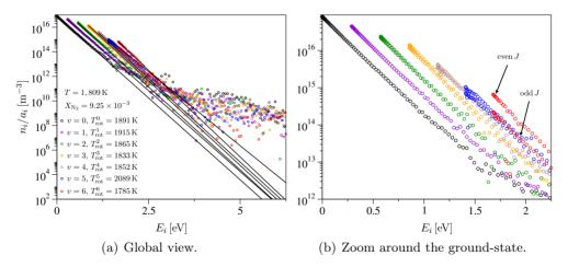
**Figure 5.6:** RVC model. Rotational energy level distribution for the ground and the first five excited vibrational states at the location  $x = 5 \times 10^{-2}$  m along the axis of the EAST facility nozzle (the unbroken lines in (a) represent the Boltzmann distributions at the rotational temperatures  $T_{\text{rot}}^v$ ).
