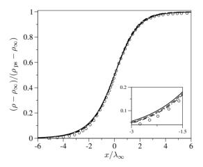
Figure 7.8: Flow across a normal shock wave in Ar. Comparison between the computed and experimental density profiles for different cross-section models ( $M_{\infty} = 3.38$ ; unbroken line VHS, dashed line LJ, dotted-dashed line PL, symbols experiments).
