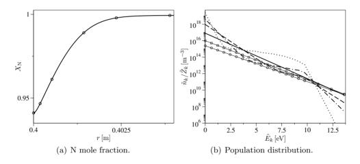
**Figure 5.23:** BRVC(20) model. Comparative evolution of the N mole fraction and the energy bin population distribution in the boundary layer. The circles in (a) indicate the locations at which the population distributions, plotted in (b), are extracted (in (b) line with circles r = 0.404 m, line with squares r = 0.402 m, unbroken line r = 0.401 m, dashed line r = 0.4005 m, dotted-dashed line r = 0.4002 m, dotted line r = 0.4 m)
