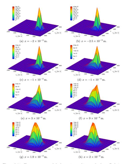
**Figure 7.21:** Flow across a normal shock wave in a multi-energy level gas. Evolution of the projection on the  $(c_x, c_y)$  plane of the velocity distribution function of level 1  $(M_{\infty} = 3)$ .
