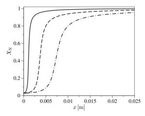
**Figure 4.2:** *RVC model.* N mole fraction evolution behind the shock wave for different values of the free-stream pressure ( $u_{\infty} = 10 \text{ km/s}$ ; unbroken lines  $p_{\infty} = 0.33 \text{ torr}$ , dashed lines  $p_{\infty} = 0.1 \text{ torr}$ , dotted-dashed lines  $p_{\infty} = 0.05 \text{ torr}$ ).
