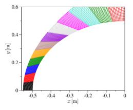
**Figure 5.33:** VC model. Mesh used for the flow over a sphere (12 blocks,  $90 \times 360$  cells; one node over three is plotted along both the axial and radial directions).
