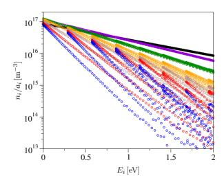
**Figure 5.5:** *RVC* model. Evolution along the axis of the EAST facility nozzle of the population of the rovibrational energy levels lying close to the ground-state (the locations at which the distributions are plotted are the same as those of fig. 5.4).
