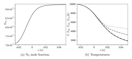
**Figure 5.3:** RVC Model. N<sub>2</sub> mole fraction and temperature evolution along the axis of the EAST facility nozzle (in (b) unbroken line T, dashed line  $T_{int}$ , dotted line  $T_{vib}$ , dotted-dashed line  $T_{rot}$ ).
