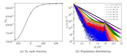
**Figure 5.4:** *RVC* model. Comparative evolution of the  $N_2$  mole fraction and the rovibrational energy level distribution along the axis of the EAST facility nozzle (the symbols in (a) highlight the locations at which the population distributions, plotted in (b), are extracted).
