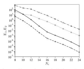
**Figure 7.12:** Isochoric equilibrium relaxation of a Ne-Ar gas.  $L_1$  and  $L_2$  norms of the error on the gas temperature with and without conservation constraint (unbroken line  $E_1$  with conservation, dashed line  $E_2$  with conservation, dotted-dashed line  $E_1$  without conservation, dotted line  $E_2$  without conservation; circles are added to highlight the number of velocity nodes used).
