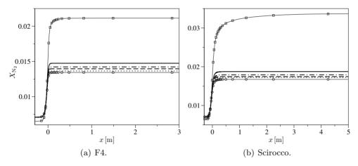
**Figure 5.16:** BRVC model. Influence of the number of energy bins on the  $N_2$  mole fraction evolution along the axis of the F4 and Scirocco nozzles (unbroken lines BRVC(2), dotted-broken lines BRVC(10), dashed lines BRVC(50), dotted lines BRVC(500), lines with circles VC, lines with squares MTP).
