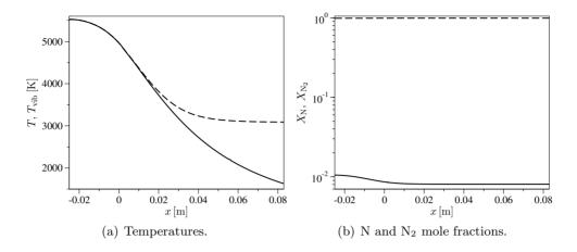
**Figure 5.30:** VC model. Temperature and mole fraction evolution along the axis of the EAST facility nozzle (in (a) unbroken line T, dashed line  $T_{vib}$ ; in (b) unbroken line N, dashed line  $N_2$ ).
