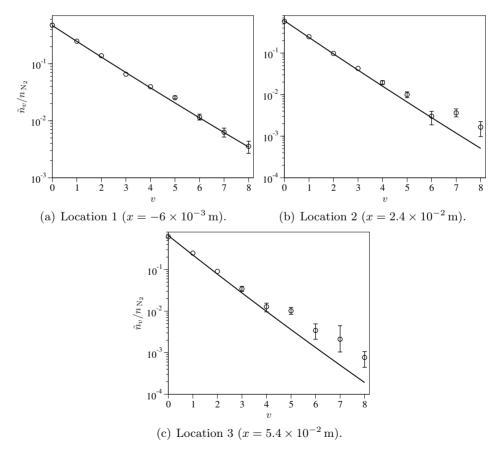
**Figure 5.32:** VC model. Comparison between the computed and experimental normalized vibrational population distributions for the EAST facility nozzle (unbroken lines calculations, circles experiments).
