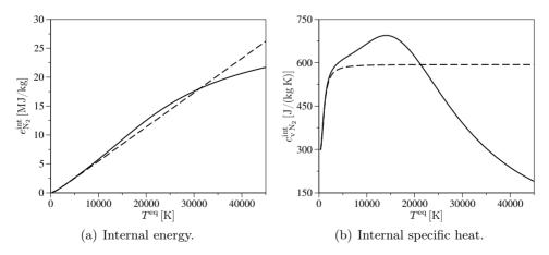
**Figure 3.3:** Internal energy and specific heat of  $N_2(^{1}\Sigma_g^{+})$  (unbroken lines NASA ARC, dashed lines RR-HO).
