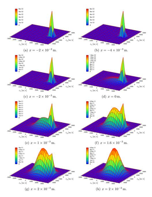
**Figure 7.6:** Flow across a normal shock wave in Ar. Evolution of the projection on the  $(c_x, c_y)$  plane of the velocity distribution function  $(M_{\infty} = 6.5)$ .
