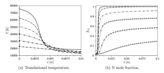
**Figure 4.3:** RVC model. Translational temperature and N mole fraction evolution behind the shock wave for different values of the free-stream velocity ( $p_{\infty} = 0.1 \text{ torr}$ ; unbroken lines  $u_{\infty} = 11 \text{ km/s}$ , dashed lines  $u_{\infty} = 10 \text{ km/s}$ , dotted-dashed lines  $u_{\infty} = 9 \text{ km/s}$ , lines with circles  $u_{\infty} = 8 \text{ km/s}$ , lines with squares  $u_{\infty} = 7 \text{ km/s}$ , lines with triangles  $u_{\infty} = 6 \text{ km/s}$ ).
