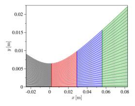
**Figure 5.28:** VC model. Mesh used for the EAST facility nozzle (4 blocks,  $200 \times 50$  cells; one node over two is plotted along both the axial and radial directions).
