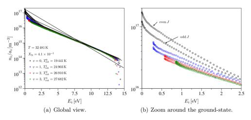
**Figure 4.8:** RVC model. Rotational energy level distribution for the ground and the first three excited vibrational states at  $x = 3.6 \times 10^{-3}$  m ( $p_{\infty} = 0.1$  torr and  $u_{\infty} = 10$  km/s; in (a) the unbroken lines represent the Boltzmann distributions at the rotational temperatures  $T_{\rm rot}^{v}$ ).
