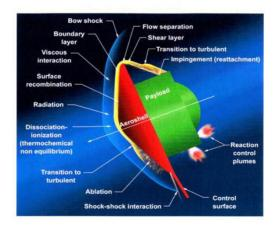
**Figure 1:** Relevant physico-chemical phenomena occurring during a planetary descent of a space vehicle (credits NASA Ames Research Center).
