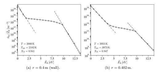
**Figure 5.24:** BRVC(20) model. Energy bin population distributions at the locations r = 0.4 m (wall) and r = 0.402 m in the boundary layer (the dashed and the dotted-dashed lines indicate the Boltzmann distributions at the translational and internal temperature, respectively).
