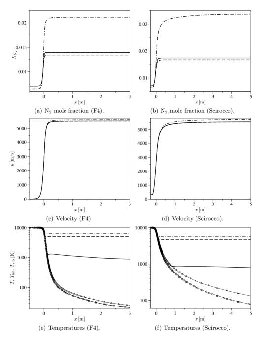
**Figure 5.13:** BRVC(50), VC and MTP model comparison. N<sub>2</sub> mole fraction, velocity and temperature evolution along the axis of the F4 and Scirocco nozzles (in (a)-(d) unbroken lines BRVC(50), dashed lines VC, dotted-dashed lines MTP; in (e)-(f) lines with circles T BRVC(50), lines with squares T VC, lines with triangles T MTP, unbroken lines  $T_{\rm int} BRVC(50)$ , dashed lines  $T_{\rm vib}$  VC, dotted-dashed lines  $T_{\rm vib}$  MTP).
