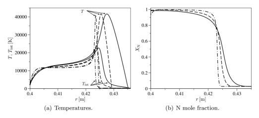
**Figure 5.18:** BRVC(20) model. Temperature and N mole fraction evolution along the stagnation-line for different values of the free-stream pressure (unbroken lines  $p_{\infty} = 0.05$  torr, dashed lines  $p_{\infty} = 0.1$  torr, dotted-dashed lines  $p_{\infty} = 0.33$  torr).
