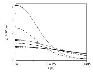
**Figure 5.26:** BRVC(20) and MTP model comparison. Heat flux evolution along the stagnation-line for different values of the free-stream pressure (unbroken line BRVC(20)  $p_{\infty} = 0.05$  torr, dashed line BRVC(20)  $p_{\infty} = 0.1$  torr, dotted-dashed line BRVC(20)  $p_{\infty} = 0.33$  torr, line with circles MTP  $p_{\infty} = 0.05$  torr, line with squares MTP  $p_{\infty} = 0.1$  torr, line with diamonds MTP  $p_{\infty} = 0.33$  torr).
