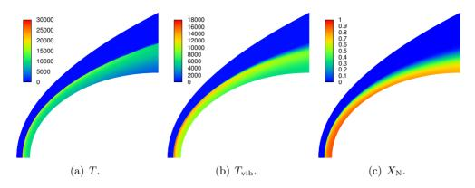
**Figure 5.34:** *VC model. Temperature and* N *mole fraction distributions around the sphere.*
