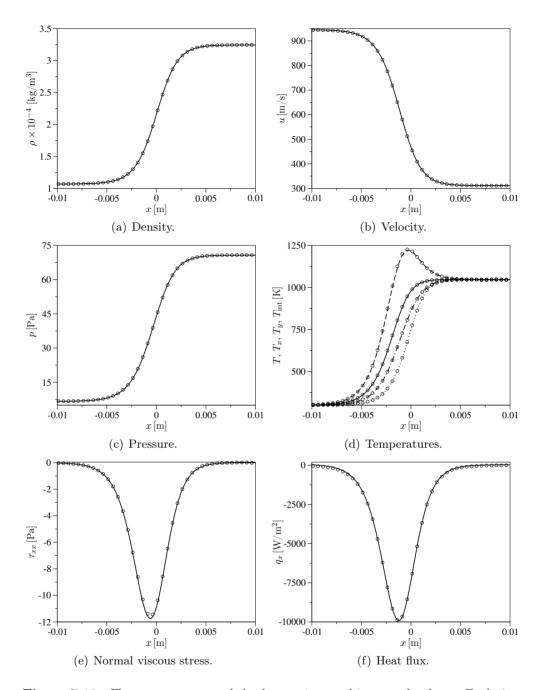
Figure 7.19: Flow across a normal shock wave in a multi-energy level gas. Evolution of the gas density, pressure, velocity, translational temperature and related parallel and transverse components, internal temperature, normal viscous stress and heat flux  $(M_{\infty} = 3; \text{ lines BEST, symbols } DSMC(Torres); \text{ in } (d) \text{ unbroken line } T, \text{ dashed line } T_x, \text{ dotted-dashed line } T_y, \text{ dotted line } T_{\text{int}}).$
