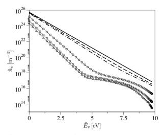
**Figure 5.31:** VC model. Evolution of the vibrational population distribution along the axis of the EAST facility nozzle (unbroken line  $x = -2.5 \times 10^{-2}$  m, dashed line  $x = -6 \times 10^{-3}$  m, dotted-dashed line x = 0 m, line with circles  $x = 2.4 \times 10^{-2}$  m, line with squares  $x = 5.4 \times 10^{-2}$  m, line with triangles  $x = 8.3 \times 10^{-2}$  m).
