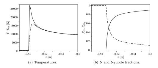
**Figure 5.35:** VC model. Temperature and N mole fraction evolution along the stagnation-line (in (a) unbroken line T, dashed line  $T_{vib}$ ; in (b) unbroken line N, dashed line  $N_2$ ).
