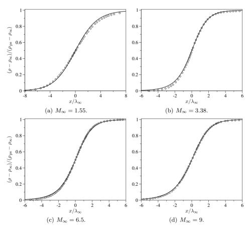
Figure 7.7: Flow across a normal shock wave in Ar. Comparison between the computed and experimental density profiles for different values of the free-stream Mach number (unbroken lines BEST, symbols experiments).
