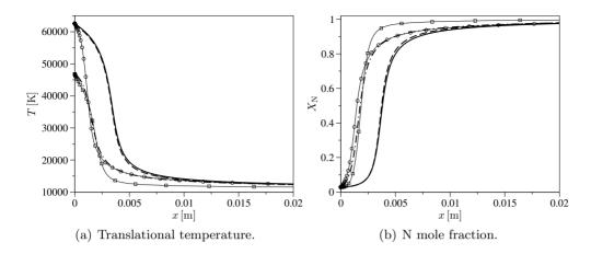
**Figure 4.15:** RVC, BRVC(50), VC, MT and MTP model comparison. Translational temperature and N mole fraction evolution behind the shock wave ( $p_{\infty} = 0.1$  torr and  $u_{\infty} = 10$  km/s; unbroken lines RVC, dashed lines BRVC(50), dotted-dashed lines VC, lines with circles MT, lines with squares MTP).
