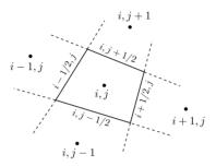
Figure 5.1: Node and cell ordering convention in the 2D structured grid code in use.
