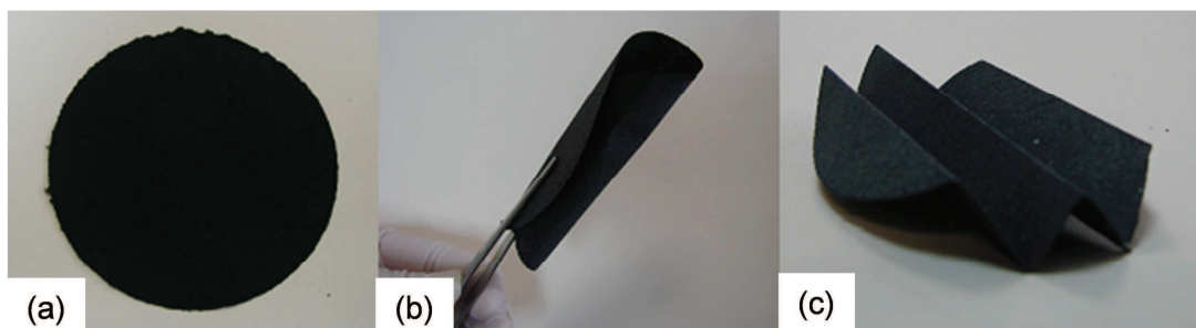
Figure III. 18 LiFePO 4 /CB/FB paper-cathode. (a) Unbent, (b) rolled-up and (c) folded.
