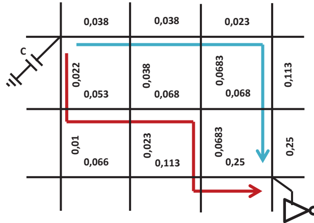
Figure 4.20: Equivalent resistor calculation example
