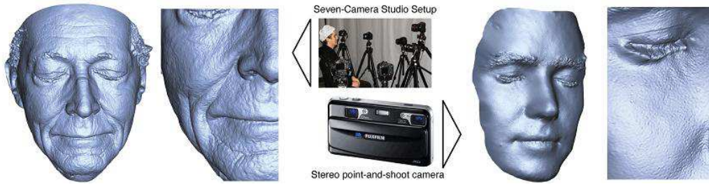
Figure 1.17: Left: Face model captured using a seven camera studio setup; Center: capture systems; Right: Face model captured using consumer binocular stereo camera. Figure is collected from [Beeler et al. 2010]
