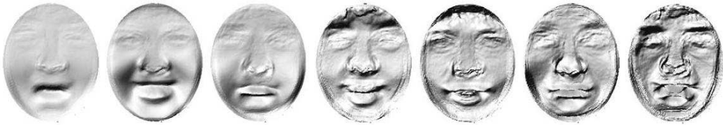
Figure 2.8: Some eigenvectors which span the shape residue PCA subspace (expression deformation model). the images from left to right are the 1st, 2nd, 3rd, 9th, 10th, 11th and 25th.eigenvectors, respectively. Notice that the eigenvectors with the higher eigenvalues are more relevant to the largely deformable regions (e.g. the mouth) and the other regions (e.g. eyebrows, eyes) gradually appear in the lower eigenvectors.[Al-Osaimi et al. 2009]
