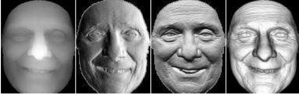
Figure G.2: From left to right: the original range image, and its normal images of component x , y and z .
