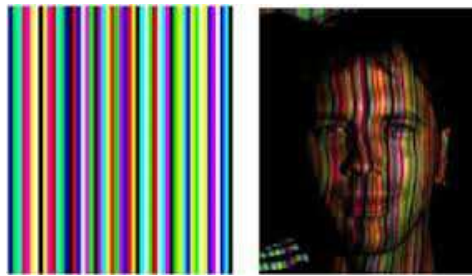
Figure 1.16: An example of structured light. A structured light (left), and its projection on to a face. Figure is collected from [Tsalakanidou et al. 2005]
