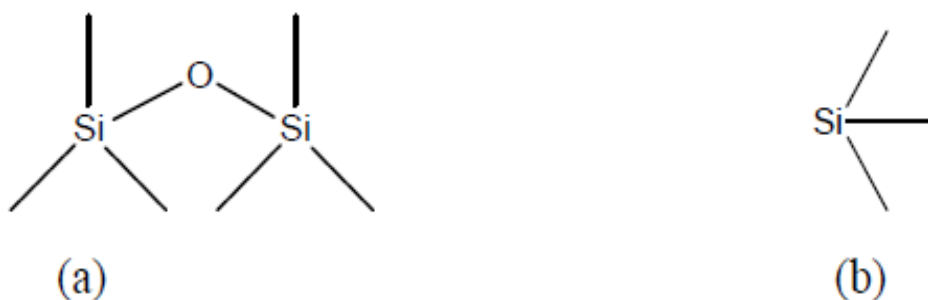
Figure 4-2. (a) Structural formula corresponding to the ratio of m/z = 147 fragments and its presence is due to the parasitic reaction occurring between an agent MTBSTFA derivatizing molecule and a water molecule. The hydrolysis and derivatization protocol includes a drying step to remove most of the water present, it can, however, never be complete. (b) Structural formula corresponding to the ratio of m/z = 73 fragment, it is the recombination of a silicon with three methyl groups (Mai-Julie NGUYEN, 2007).
