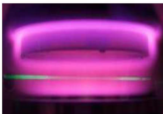
Figure 1-13. Picture for the \text{CH}_4\text{-N}_2 plasma in the PAMPRE reactor, the green trace corresponds to the diffusion of powders suspended at 532 nm green laser.
