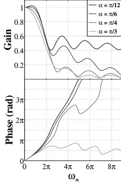
**Figure 4.5:** FTF component  $F_A$  gain (top) and phase lag (bottom) evolution as a function of the reduced frequency  $\omega_*$  for different values of the flame angle  $\alpha = \pi/3$ ,  $\pi/4$ ,  $\pi/6$  and  $\pi/12$  with respect to the flow direction. The darkness is associated to decreasing values of  $\alpha$ :  $\alpha = \pi/12$  (black).  $\alpha = \pi/3$  (light gray).
