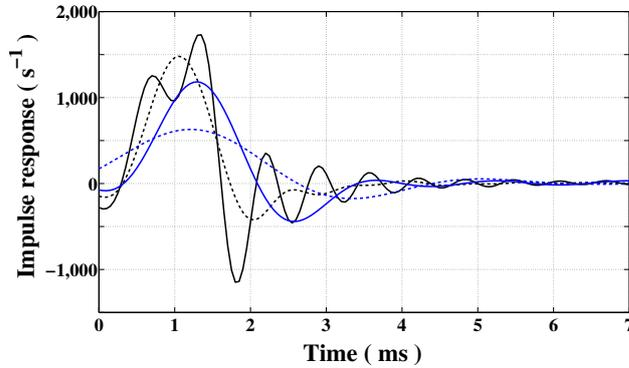
**Figure B.7:** Impulse response of a collection of small premixed laminar conical flames. These data are determined from FDF measurements where  $v_1^{\text{rms}}/U_b = 0.06$  (black solid line), 0.26 (black dashed line), 0.46 (blue solid line) and 0.66 (blue dashed line).
