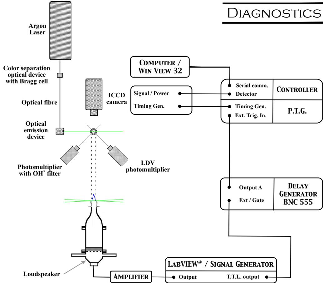
**Figure 2.2:** Setup with diagnostics. A signal is generated to trigger the ICCD camera and to drive the loudspeaker. The loudspeaker generates acoustic velocity perturbations measured with a LDV system at the burner outlet. These perturbations produce flame front wrinkles that are captured by the camera and heat release rate perturbations that are recorded by a photomultiplier equipped with an  $OH^*$  filter.
