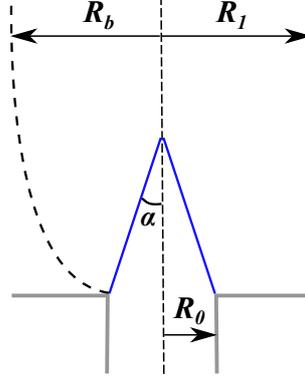
**Figure 6.1:** Scheme of a conical flame showing the different notations needed in this study. The injection unit radius  $R_0$  has to be compared to the burnt gas plume radius  $R_b$  occupied by the flame if it would be unconfined (left side of the figure) and to the radius of the flame tube  $R_1$  confining the burnt gases (right side of the figure). The flame tip half-angle  $\alpha$  is also indicated in this figure.
