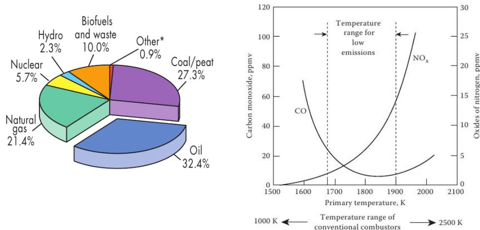
**Figure 1:** (left) World total primary energy supply in 2010 from the International Energy Agency. “Other\*” includes geothermal, solar and wind. (right) CO and NO<sub>x</sub> concentrations as a function of the combustion zone temperature, from Lefebvre and Ballal (2010).
