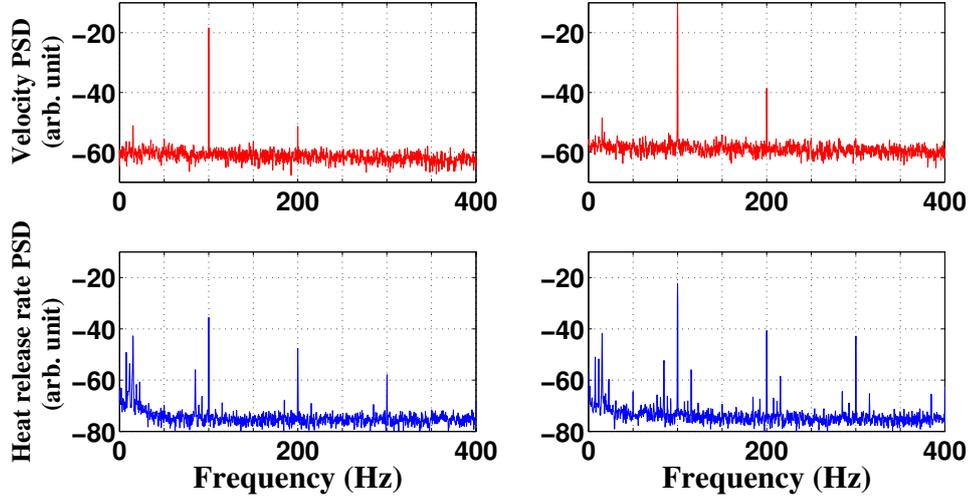
**Figure 2.5:** Power spectral density of the velocity signal (red line) and the heat release rate signal (blue line) for a forcing frequency  $f = 100$  Hz and perturbation levels of  $|v_1/v_0| = 0.1$  (left) and  $0.3$  (right).
