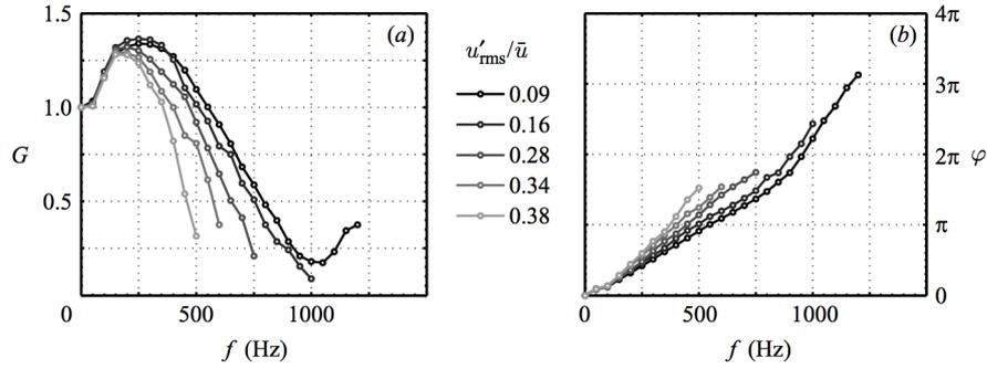
**Figure 7.1:** Flame Describing Function gain  $G$  and phase  $\varphi$  as a function of frequency  $f$  and perturbation level  $u'_{\text{rms}}/\bar{u}$ . Reproduced from *Noiray et al. (2008)*.
