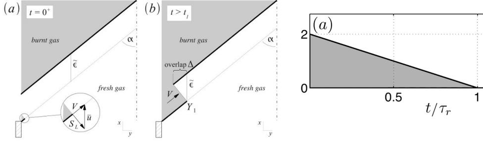
**Figure 1.9:** Flame response (left) and dimensionless impulse response of a conical flame  $h_U(t)\tau_r$  (right) in the case of a uniform velocity perturbation. Reproduced from [Blumenthal et al. (2013)].
