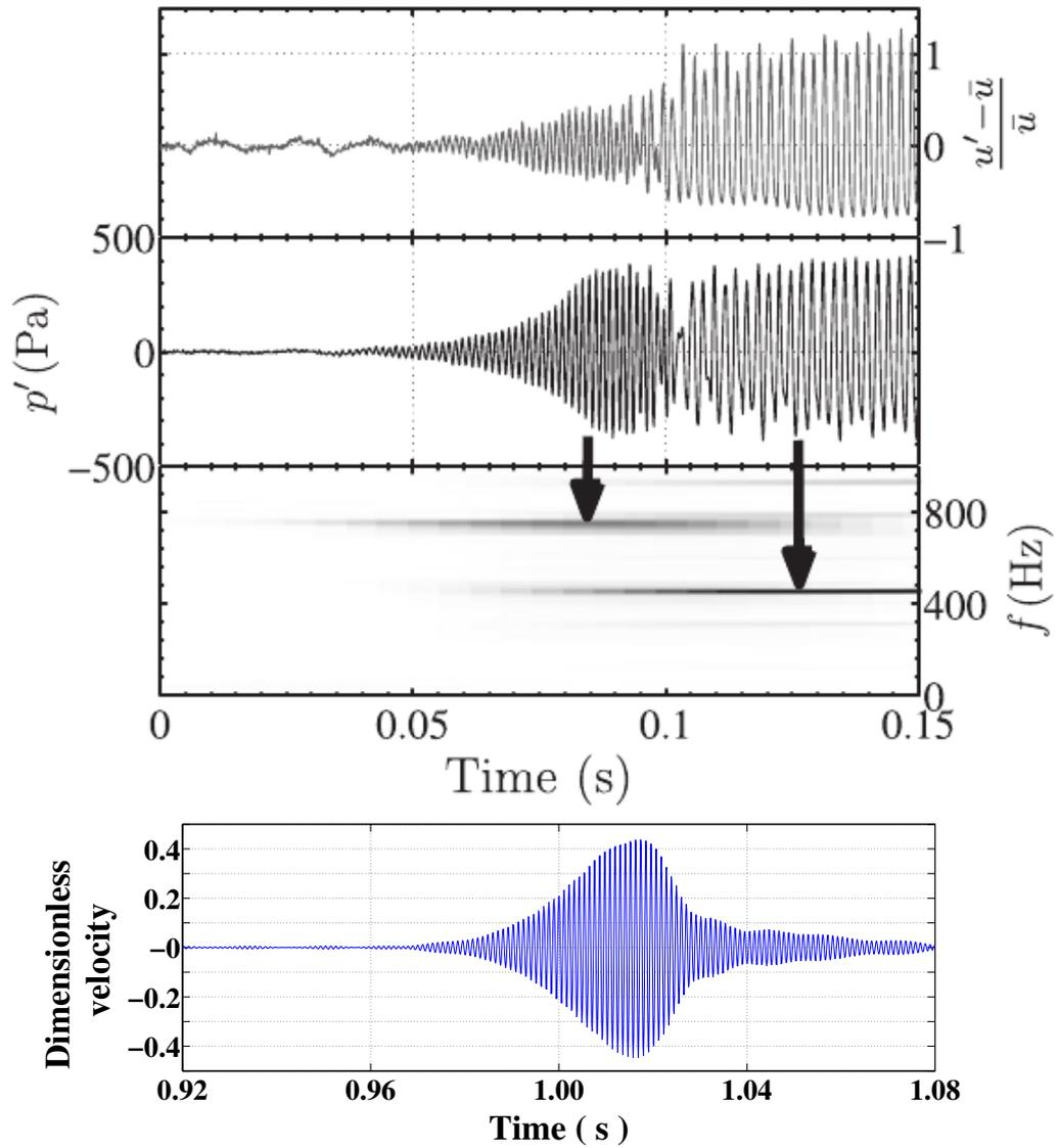
**Figure 8.11: Top:** Temporal signals of the self-sustained instability. The two upper plots show the normalized velocity and the pressure oscillations in the plenum. The lower plot corresponds to the short-time Fourier spectral density of the pressure signal. Reproduced from *Boudy et al. (2011)*. **Bottom:** Dimensionless velocity perturbation signal filtered around the high frequency of the instability.  $L_1 = 0.54$  m.  $l = 0.003$  m.
