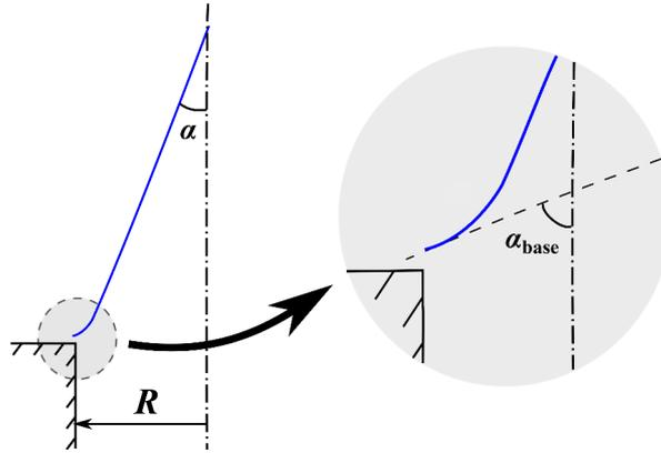
**Figure 5.6:** Scheme of a conical flame with a zoom on the flame base showing the difference between the flame tip half-angle  $\alpha$  and the flame base angle  $\alpha_{\text{base}}$ .
