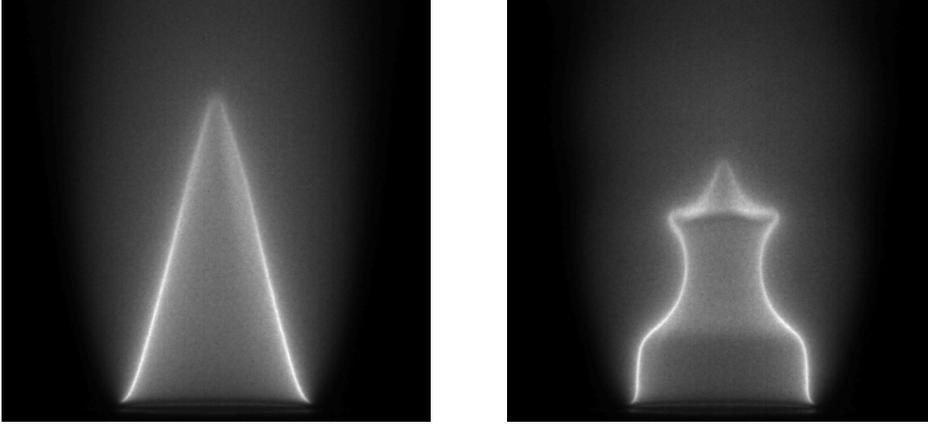
**Figure 2.6:** *Images of a steady (left) and acoustically perturbed (right) conical flame.  $\phi = 1.03$ .  $v_0 = 1.56 \text{ m.s}^{-1}$ . Right figure:  $f = 100 \text{ Hz}$ .*
