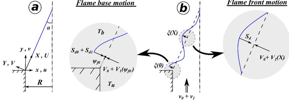
**Figure 1.3:** Schematic of the configuration investigated. (a) Steady conical flame along with the different frames used in this chapter. (b) Acoustically perturbed conical flame, with a focus on the flame base region and the flame front displacement far from the burner lip.
