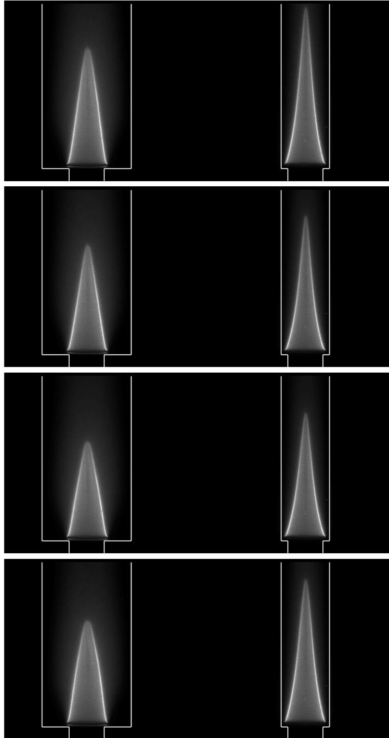
**Figure 6.9:** Images of acoustically perturbed confined conical flames for four equidistant phases during the forcing period. Left column:  $C_r = 0.44$ . Right column:  $C_r = 0.81$ .  $f = 10$  Hz.  $\dot{m} = 0.792$  g.s<sup>-1</sup>.  $|v_1/v_0| = 0.1$ .  $\phi = 0.86$ .
