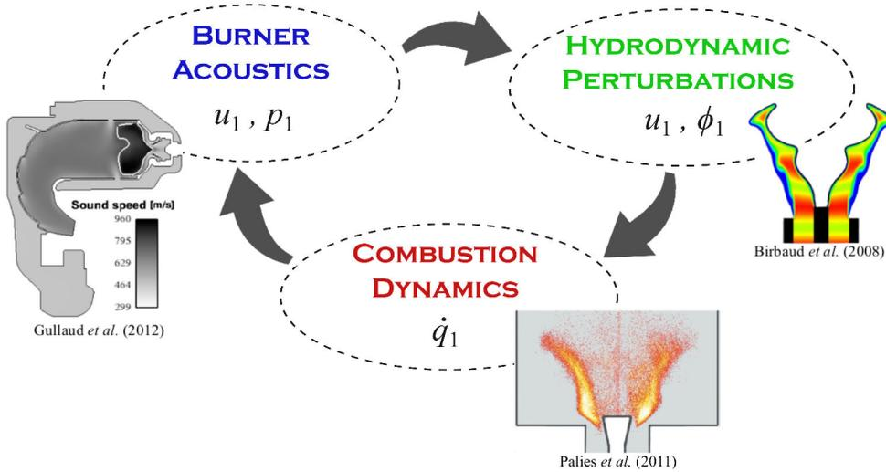
**Figure 4:** Representation of the resonant coupling leading to thermo-acoustic instabilities. The acoustic waves are characterized by their velocity and pressure perturbations  $u_1, p_1$  that satisfy the wave equation. Acoustic perturbations produce hydrodynamic perturbations  $u_1, \phi_1$ . The unsteady combustion leads to delayed heat release rate perturbations  $\dot{q}_1$  that act as a source term in the wave equation.
