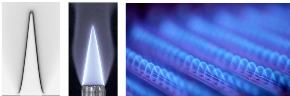
**Figure 3:** (left) *2D premixed laminar conical flame. Reproduced from Selle et al. (2011).* (center) *Axisymmetric laminar premixed conical flame. Reproduced from Durox et al. (2004).* (right) *Premixed laminar conical flames of a burner placed inside a domestic boiler. Reproduced from www.lovekin.co.uk.*
