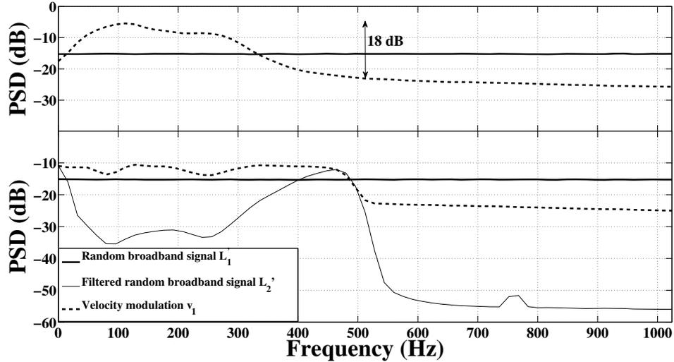
**Figure 3.5:** Power spectral densities of (top figure) (—) the random broadband signal  $L_1$  and (- - -) the uncontrolled velocity perturbations  $v_1$  (bottom figure) (—) the random broadband signal  $L_1$ , (...) the broadband signal  $L_2$  resulting from the filtering of  $L_1$  by  $\mathcal{H}_{mp}^{-1}(\omega)$  and (- - -) the resulting controlled velocity perturbations  $v_1$ .
