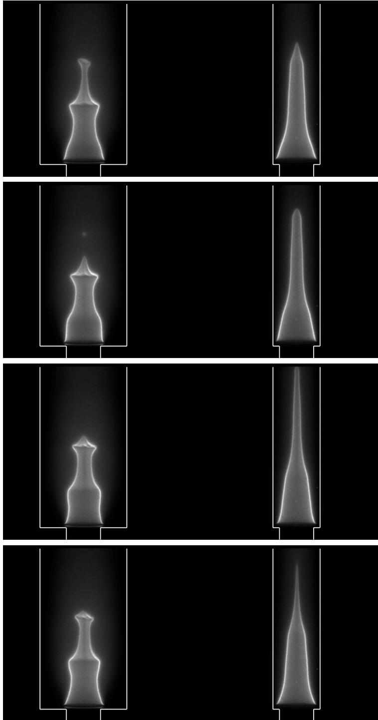
**Figure 6.10:** Images of acoustically perturbed confined conical flames for four equidistant phases during the forcing period. Left column:  $C_r = 0.44$ . Right column:  $C_r = 0.81$ .  $f = 80$  Hz.  $\dot{m} = 0.792$  g.s<sup>-1</sup>.  $|v_1/v_0| = 0.1$ .  $\phi = 0.86$ .
