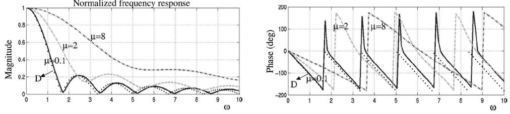
**Figure 1.6:** Exothermicity effects on the FTF gain (left) and phase lag (right) of a ducted V-flame. The different curves are a function of the parameter  $\mu = \rho_u/\rho_b - 1$ . Reproduced from [Mehta et al. \(2005\)](#). The FTF phase decreases at low frequencies because the “ $\exp(i\omega t)$ ” convention was adopted in this article.
