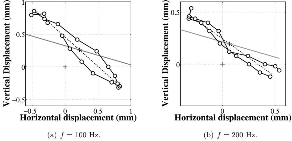
**Figure 5.4:** Flame base motion for a modulation amplitude of  $v_1^{\text{rms}}/v_0 = 0.1$  (grey +) Steady flame base location. (black +) Mean location of the flame base displacement. (black line) Flame base motion determined experimentally. (black dashed line) Measured direction normal to the flame front at the flame base, defined by  $\alpha_{\text{base}}$ . (grey solid line) Theoretical direction normal to the flame front, defined by  $\alpha = \arcsin(S_{a0}/v_0)$ .
