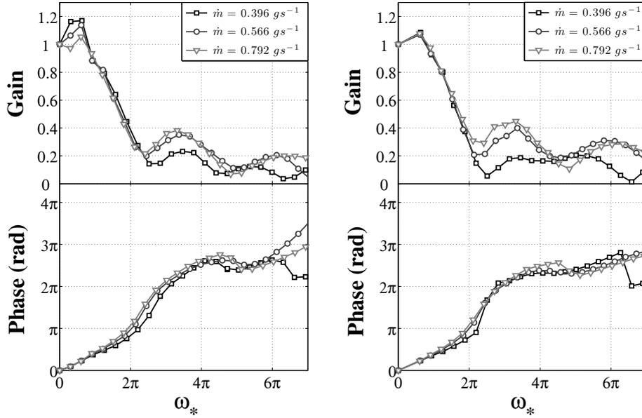
**Figure 6.12:** FTF gain (top) and phase (bottom) as a function of the reduced frequency  $\omega_*$ , for three different inlet mass flow rates and for two confinement ratios:  $C_r = 0$  (left) and  $C_r = 0.44$  (right).
