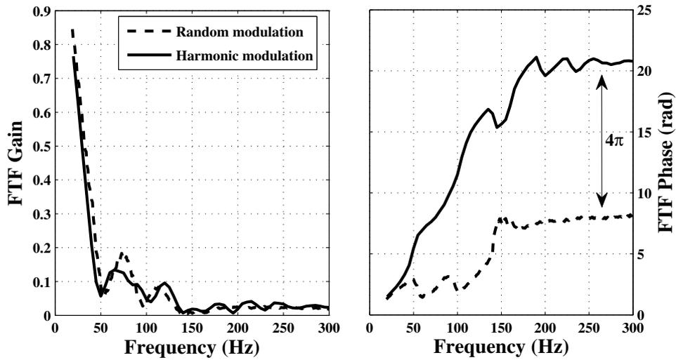
Figure 3.9: *FTF* obtained with harmonic and random velocity modulation and cross-correlation techniques, for a relative rms velocity perturbation of  $v_1^{\text{rms}}/v_0 = 0.12$ .
