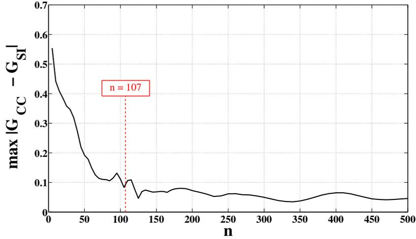
**Figure 3.12:** Convergence of the SI method. The gain difference  $|G_{CC} - G_{SI}|$  is plotted as a function of the number of coefficients  $n = n_a = n_b$  used to model the IIR flame response.  $v_1^{\text{rms}}/v_0 = 0.04$ .
