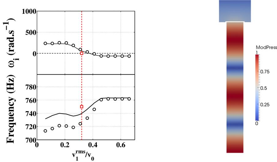
**Figure 8.12:** **Left:** Oscillation frequency  $f$  and growth rate  $\omega_i$  of the third eigenmode are plotted as a function of the perturbation level  $v_1^{\text{rms}}/v_0$ . Numerical results from AVSP ( $\circ$ ) and from LOM (-) are compared to experimental data ( $\square$ ) from [Boudy et al. \(2011\)](#). **Right:** Pressure modulus distribution calculated by AVSP indicating the structure of the third eigenmode at limit cycle.  $L_1 = 0.54$  m and  $l = 0.003$  m.
