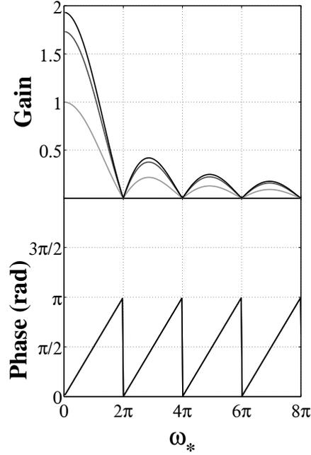
**Figure 5.1:** Transfer function  $F_C(\omega_*, \alpha)$  plotted as a function of reduced frequency  $\omega_*$  for different angles  $\alpha = \pi/12$  (black),  $\pi/6$  (dark grey), and  $\pi/3$  (light grey).
