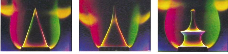
**Figure 1.1:** Three color Schlieren images of  $\text{CH}_4/\text{air}$  conical flames. **(left)** Steady flame for  $v_0 = 0.96 \text{ m.s}^{-1}$  and  $\phi = 0.95$ . **(center)** Perturbed flame at  $f = 25 \text{ Hz}$ . **(right)** Perturbed flame at  $f = 75 \text{ Hz}$ . Reproduced from *Ducruix et al. (2000)*.
