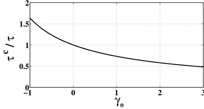
**Figure 6.15:** Evolution of the ratio of the time lag derived for elongated confined conical flames (Eq. 6.32) divided by the time lag  $\tau = (1/3)H_0/v_0$  of an elongated unconfined conical flame as a function of the parameter  $\gamma_*$ .
