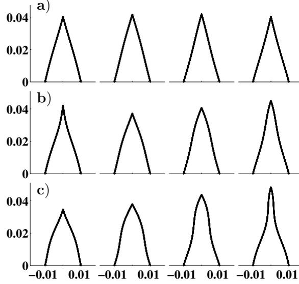
**Figure 4.2:** Flame shapes predicted with (a) a uniform velocity perturbation [Ducruix et al. (2000)]; (b) a convected velocity disturbance [Schuller et al. (2003a)]; (c) the model derived in the present chapter. The flame is presented for four different phases of the acoustic period, namely  $0$ ,  $\pi/2$ ,  $\pi$  and  $3\pi/2$ . Flame motions are calculated for  $\alpha = \pi/12$ ,  $|v_1/v_0| = 0.1$  and  $\omega_* = 5$ .
