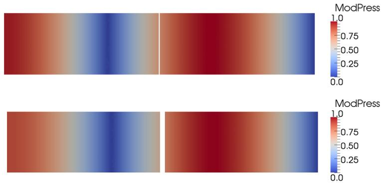
**Figure C.5:** *Pressure modulus distribution of the second acoustic eigenmode of the system. Top figure:  $h = 3$  mm. Bottom figure:  $h = 15$  mm.*
