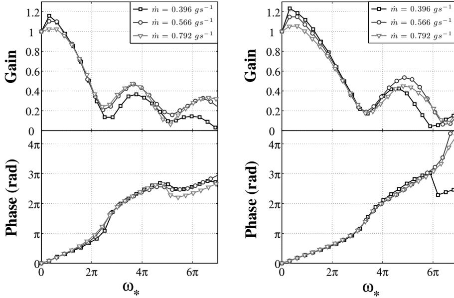
**Figure 6.13:** FTF gain (top) and phase (bottom) as a function of the reduced frequency  $\omega_*$ , for three different inlet mass flow rates and for two confinement ratios:  $C_r = 0.60$  (left) and  $C_r = 0.81$  (right).
