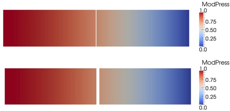
**Figure C.4:** *Pressure modulus distribution of the first acoustic eigenmode of the system. Top figure:  $h = 3$  mm. Bottom figure:  $h = 15$  mm.*
