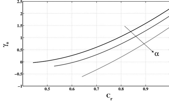
**Figure 6.7:** Evolution of  $\gamma_*$  as a function of the confinement ratio  $C_r$  for values of  $C_r$  satisfying Eq. (6.15). Different flame tip half-angles are considered:  $\alpha = \pi/12$  (black),  $\pi/6$  (dark grey) and  $\pi/4$  (light grey).  $E = 6$ .
