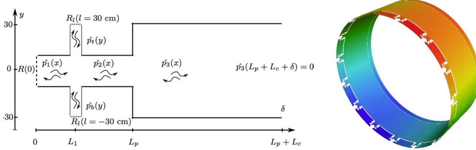
**Figure 5:** (left) *Acoustic network method applied to a two-cavity combustor with the feeding lines. Reproduced from Richecoeur et al. (2013).* (right) *First azimuthal mode in an annular chamber simulated with the Helmholtz solver AVSP. Reproduced from Sensiau (2008).*
