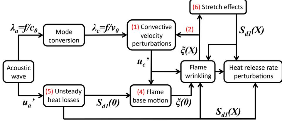
**Figure 1.4:** Mechanisms contributing to the conical flame dynamics when submitted to acoustic perturbations.  $u'_a$ : acoustic velocity perturbations of wavelength  $\lambda_a$ .  $u'_c$ : convective velocity perturbations of wavelength  $\lambda_c$ .  $S_{dl}(X)$ : flame speed disturbances.  $\xi(X)$ : flame front wrinkle.  $X = 0$ : flame base location. Red numbers in between parentheses refer to the mechanisms listed in Section 1.3 below.
