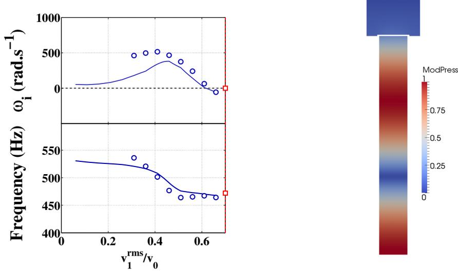
**Figure 8.13: Left:** Oscillation frequency  $f$  and growth rate  $\omega_i$  of the second eigenmode are plotted as a function of the perturbation level  $v_1^{\text{rms}}/v_0$ . Numerical results from AVSP ( $\circ$ ) and from LOM (-) are compared to experimental data ( $\square$ ) from Boudy et al. (2011). **Right:** Pressure modulus distribution calculated by AVSP indicating the structure of the second eigenmode at limit cycle.  $L_1 = 0.54$  m and  $l = 0.003$  m.
