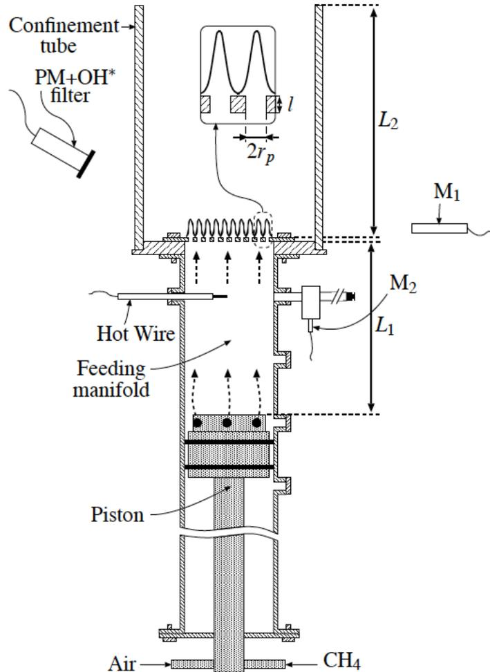
**Figure 8.1:** *Experimental setup used to characterize self-sustained thermo-acoustic oscillations involving combustion [Boudy (2012)]. Reactants are premixed upstream and a piston is used to modify the feeding manifold length  $L_1$ . A perforated plate of thickness  $l$  and hole radius  $r_p$  acts as an anchoring device for a collection of small laminar conical flames. The flame tube, made out of quartz and of length  $L_2 + l$ , allows the confinement of the combustion zone.*
