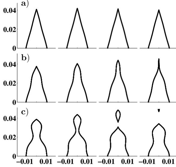
**Figure 4.3:** Flame shapes predicted with (a) a uniform velocity perturbation [Ducruix et al. (2000)], (b) a convected velocity disturbance [Schuller et al. (2003a)], and (c) the model derived in the present chapter. The flame is presented for four different phases of the acoustic period, namely  $0$ ,  $\pi/2$ ,  $\pi$  and  $3\pi/2$ . Flame motions are calculated for  $\alpha = \pi/12$ ,  $|v_1/v_0| = 0.1$  and  $\omega_* = 10$ .
