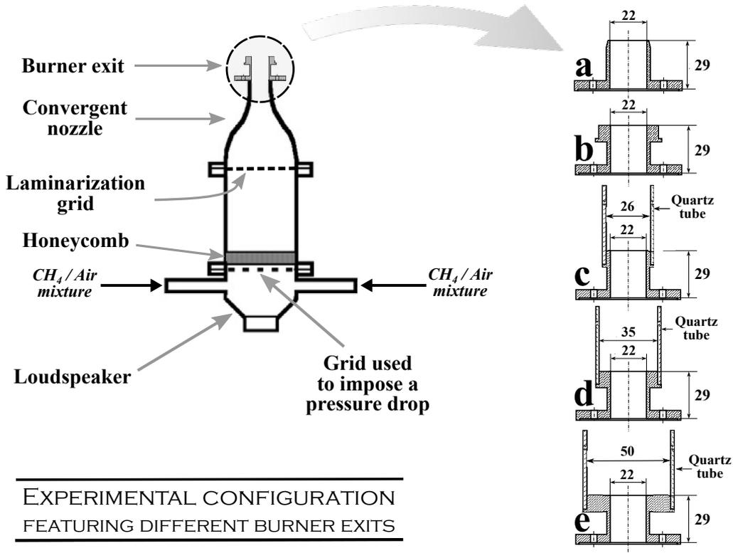
**Figure 2.1:** Burner geometry used for the experimental investigation. The reactive mixture is injected at the bottom and outflows the burner through a cylindrical exit. Three burner exit configurations were used: (a) a cylindrical piece with a beveled edge, (b) a cylindrical piece with a plateau and (c,d,e) a cylindrical piece with a plateau supporting a quartz tube.
