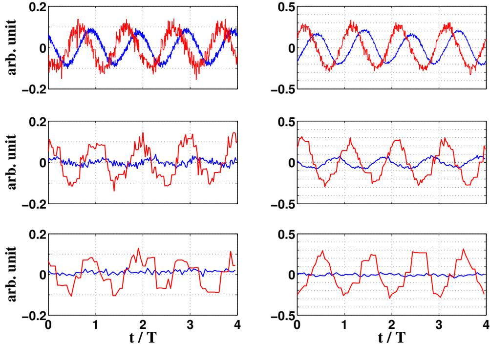
**Figure 2.3:** Dimensionless heat release rate perturbations  $\dot{Q}_1/Q_0$  (blue line) and velocity modulations  $v_1/v_0$  (red line) are plotted as a function of the time that is made dimensionless by the period  $T = 1/f$  associated to the forcing frequency. Upper row:  $f = 20$  Hz. Middle row:  $f = 100$  Hz. Lower row:  $f = 200$  Hz. Left column:  $|v_1/v_0| = 0.1$ . Right column:  $|v_1/v_0| = 0.3$ .
