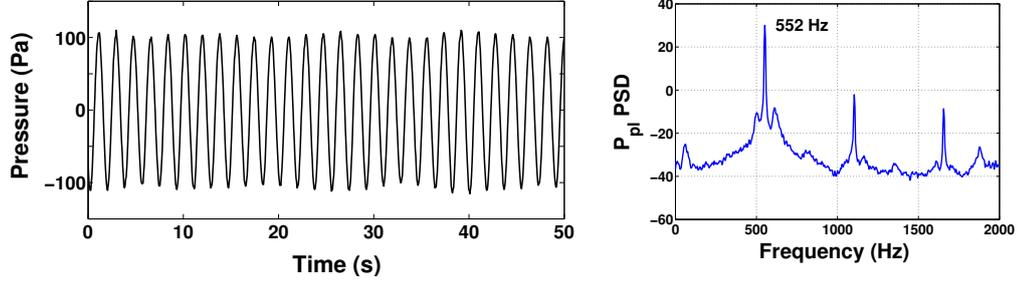
**Figure 8.6:** **Left:** Pressure evolution in the plenum at limit cycle. **Right:** Power spectral density of the pressure signal measured at limit cycle.  $L_1 = 0.12$  m and  $l = 0.003$  m.
