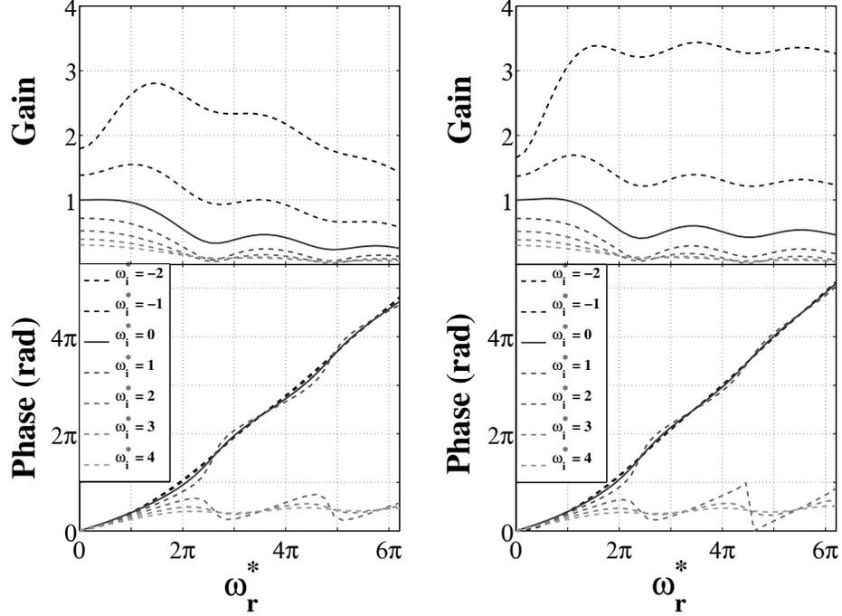
**Figure B.2:** Flame Transfer Function as a function of the reduced frequency  $\omega_r^*$  for different values of the dimensionless reduced growth rate  $\omega_i^*$ .  $\alpha = \pi/6$  (left figure) and  $\alpha = \pi/12$  (right figure).
