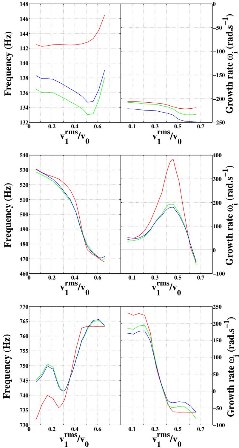
**Figure B.9:** Results from a nonlinear stability analysis combining a low-order acoustic network solver and the FDF methodology, for the first (top), second (center) and third (bottom) eigenmode. (red line) The flame frequency response and the inlet and outlet reflection coefficients are taken as  $F(\omega_r)$  and  $R(\omega_r)$ . (green line)  $F(\omega)$  and  $R(\omega_r)$ . (blue line)  $F(\omega)$  and  $R(\omega)$ .
