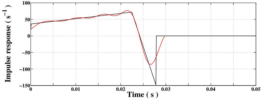
**Figure B.5:** *Impulse response of a single premixed laminar conical flame. (black line) Analytical model that considers incompressible convective perturbations. (red line) Impulse response determined from a discrete set of samples of an analytical FTF and the application of the reconstruction algorithm.*
