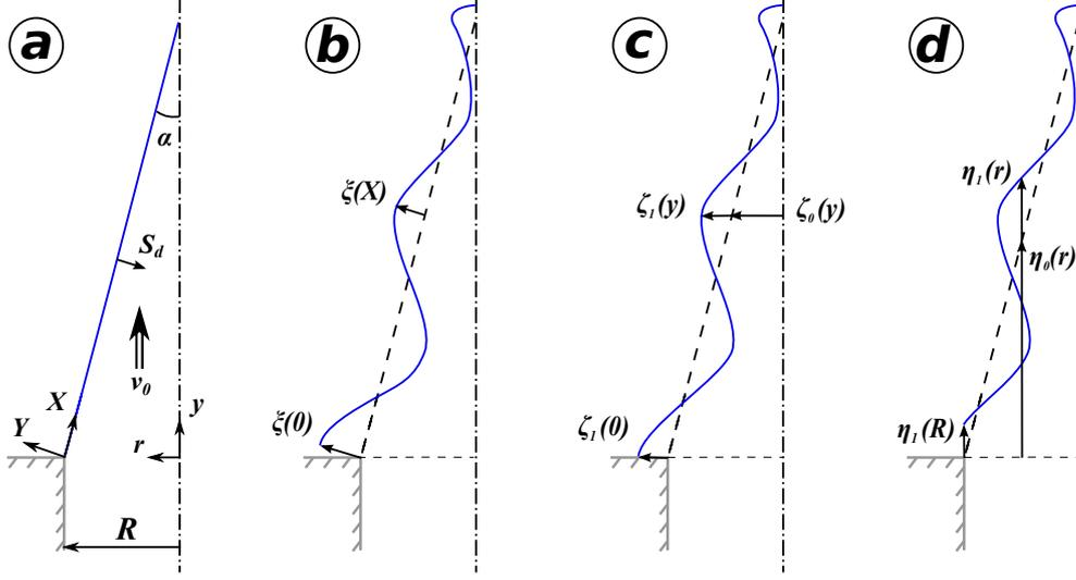
**Figure A.1:** Different configurations explored. (a) Steady laminar conical flame. (b) Unsteady flame perturbed by a flame base displacement along a direction normal to the steady flame front  $\xi(X=0)$ . (c) Unsteady flame perturbed by a horizontal flame base displacement  $\zeta_1(y=0)$ . (d) Unsteady flame perturbed by a vertical flame base displacement  $\eta_1(r=R)$ .
