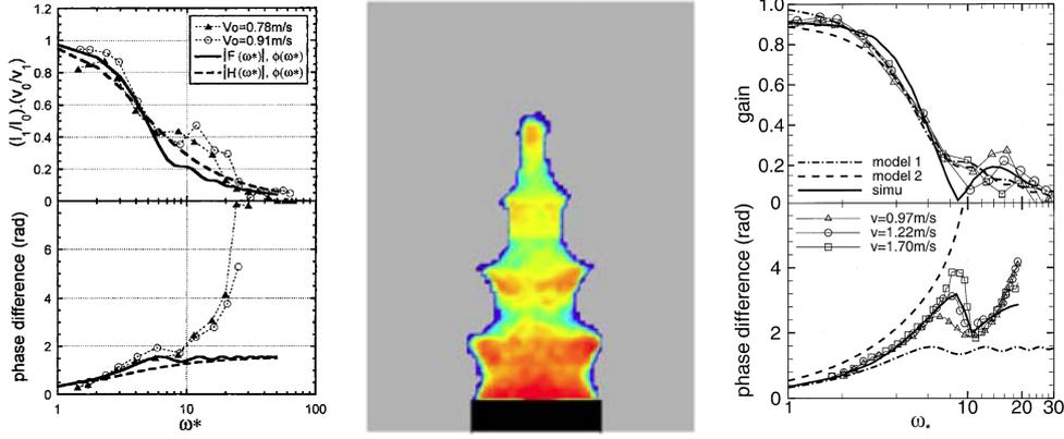
**Figure 1.5:** (center) PIV measurements of an acoustically perturbed conical flame, from *Birbaud et al. (2006)*. The fresh gas zone is colored with the axial velocity field. (left and right) Comparisons between experimentally determined FTF and the FTF component  $F_A$  gain (top) and phase (bottom) from the models derived by *Ducruix et al. (2000)* (left) and by *Schuller et al. (2003a)* (right). The FTF gain and phase lag are plotted as a function of the reduced frequency  $\omega_*$ .
