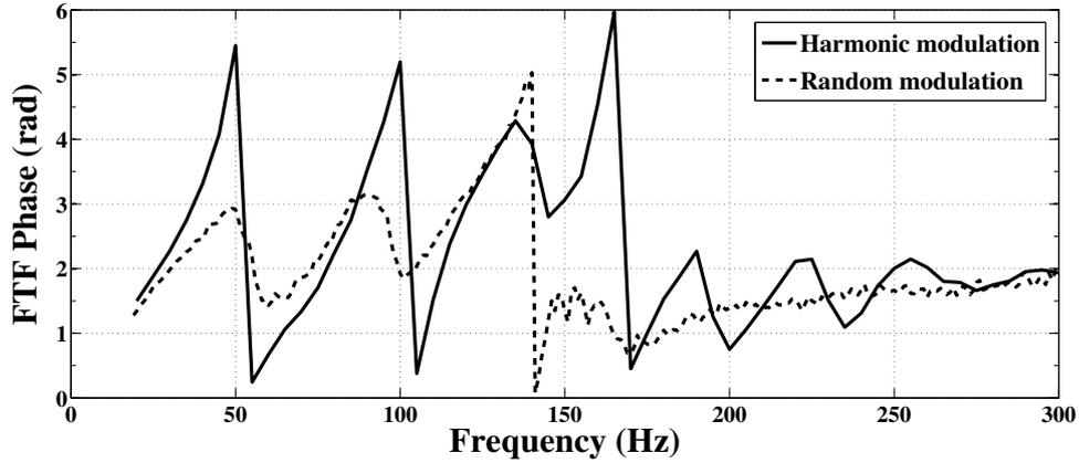
**Figure 3.10:** Phase lag of the FTF, wrapped between 0 and  $2\pi$ , for a relative rms velocity perturbation of  $v_1^{\text{rms}}/v_0 = 0.12$  when the flame is submitted to harmonic (-) or random (-) velocity disturbances.
