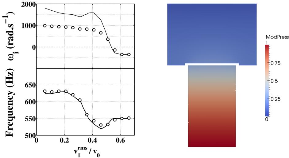
**Figure 8.7:** *Left:* Oscillation frequency  $f$  and growth rate  $\omega_i$  are plotted as a function of the perturbation level  $v_1^{\text{rms}}/v_0$ . Numerical results from AVSP ( $\circ$ ) are compared to results from LOM (-). *Right:* Pressure modulus distribution calculated by AVSP indicating the structure of the corresponding eigenmode at limit cycle.  $L_1 = 0.12$  m and  $l = 0.003$  m.
