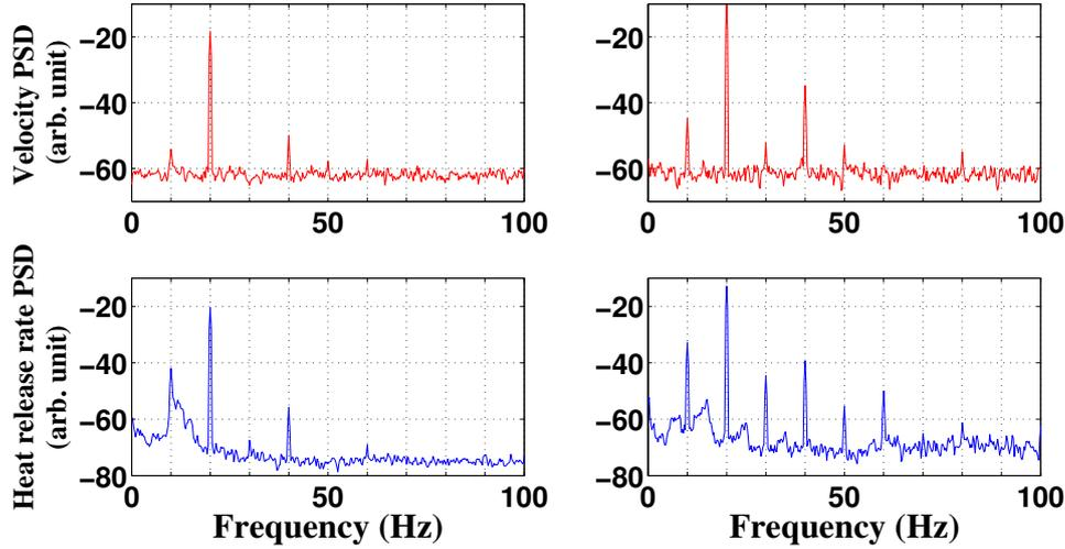
**Figure 2.4:** Power spectral density of the velocity signal (red line) and the heat release rate signal (blue line) for a forcing frequency  $f = 20$  Hz and perturbation levels of  $|v_1/v_0| = 0.1$  (left) and  $0.3$  (right).
