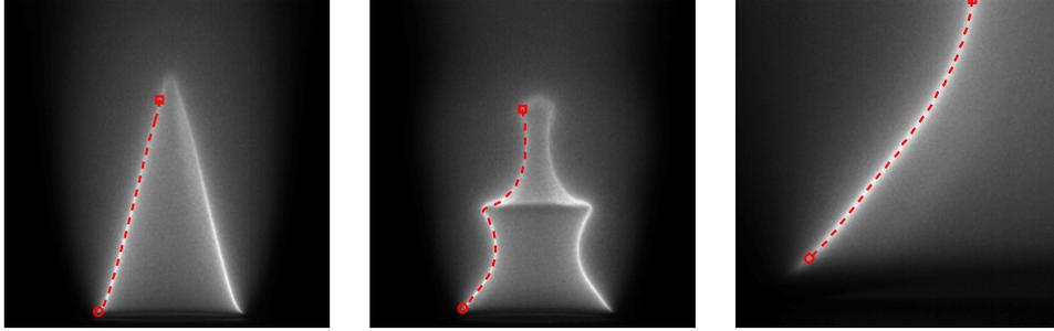
**Figure 2.7:** Images of a steady (left) and acoustically perturbed (center) conical flames. A zoomed image of the perturbed flame base is also shown (right). On each image, a dashed red line shows the result of the flame front detection algorithm, with a flame base and tip detection threshold of 60 % of the maximum value.  $\phi = 1.03$ .  $v_0 = 1.56 \text{ m.s}^{-1}$ .
