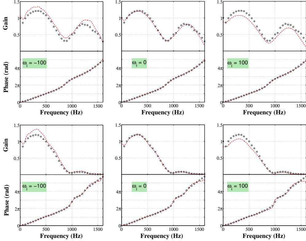
**Figure B.8:** *FTF as a function of the frequency. (black  $\circ$ ) Experimental FTF measured with constant amplitude harmonic signals for  $v_1^{\text{rms}}/U_b = 0.06$  (top row) and  $v_1^{\text{rms}}/U_b = 0.26$  (bottom row). (red line) FTF for different growth rates  $\omega_i = -100$  (left), 0 (center) and  $100 \text{ rad}\cdot\text{s}^{-1}$  (right), determined with the reconstruction based on the experimental data measured for  $\omega_i = 0$ .*
