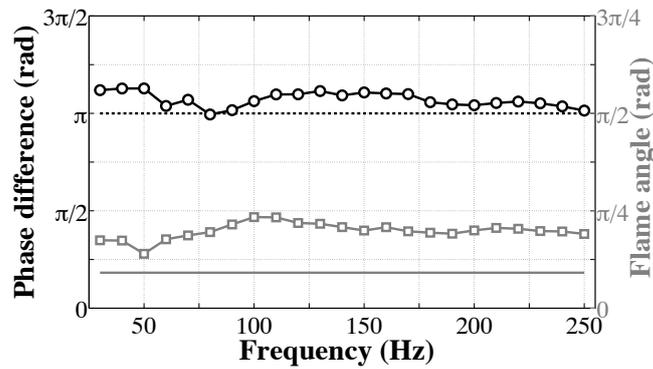
**Figure 5.7:** Evolutions of the (black curve and circles) phase difference between the horizontal and the vertical flame front displacement at its base, (grey line) flame tip half-angle defined by  $\alpha = \arcsin(S_d/v_0)$  and (grey circles) angle  $\alpha_{\text{base}}$  between the flame front at the flame base and the vertical axis. Perturbation level  $v_1^{\text{rms}}/v_0 = 0.1$ .
