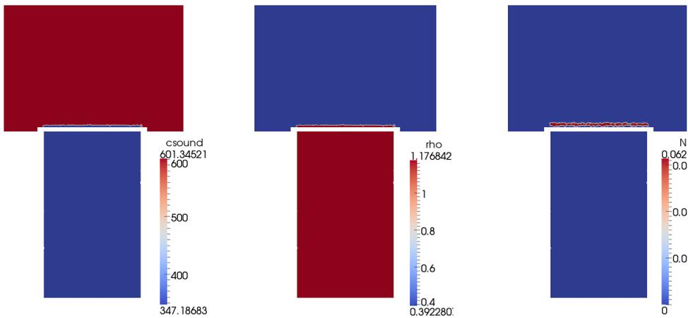
**Figure 8.3:** **Left:** Field of the speed of sound modeling effects of steady combustion (in  $m.s^{-1}$ ). **Middle:** Corresponding field of density (in  $g.m^{-3}$ ). **Right:** Field of magnitude of the source term appearing in the right-hand side of the Eq. (7.17) corresponding to a compact flame location above the perforated plate.
