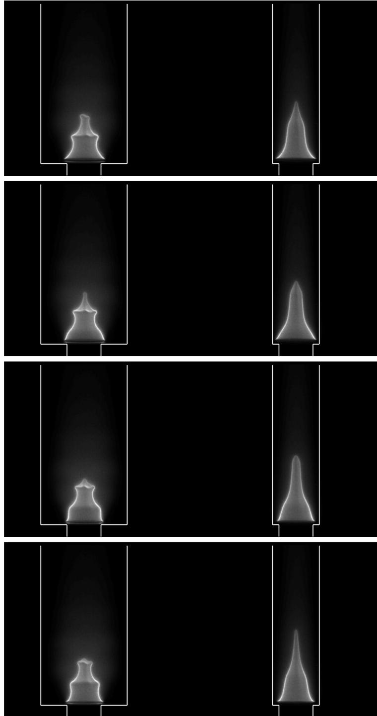
**Figure 6.11:** Images of acoustically perturbed confined conical flames for four equidistant phases during the forcing period. Left column:  $C_r = 0.44$ . Right column:  $C_r = 0.81$ .  $f = 80$  Hz.  $\dot{m} = 0.396$  g.s<sup>-1</sup>.  $|v_1/v_0| = 0.1$ .  $\phi = 0.86$ .
