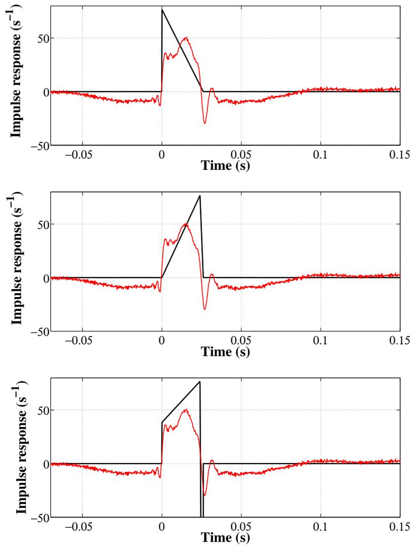
**Figure 4.11:** The experimentally determined impulse response (red curves) is plotted as a function of time and compared to predictions from different models (black curves): uniform model (top), convective model (center) and incompressible convective model (bottom).  $\tau_r = 0.261 \text{ s}^{-1}$ ,  $\tau_c = 0.240 \text{ s}^{-1}$ .
