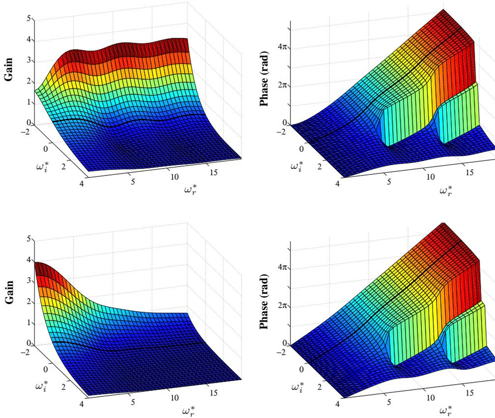
**Figure B.1:** Flame Transfer Function gain (left) and phase (right) as a function of the reduced real frequency  $\omega_r^*$  and the reduced growth rate  $\omega_i^*$ . The models used are derived from an incompressible convective model (top figures) and from a convective model [Schuller et al. (2003a)]. The FTF values derived for  $\omega_i^* = 0$  are highlighted as a thick black curve.  $\alpha = \pi/12$ .
