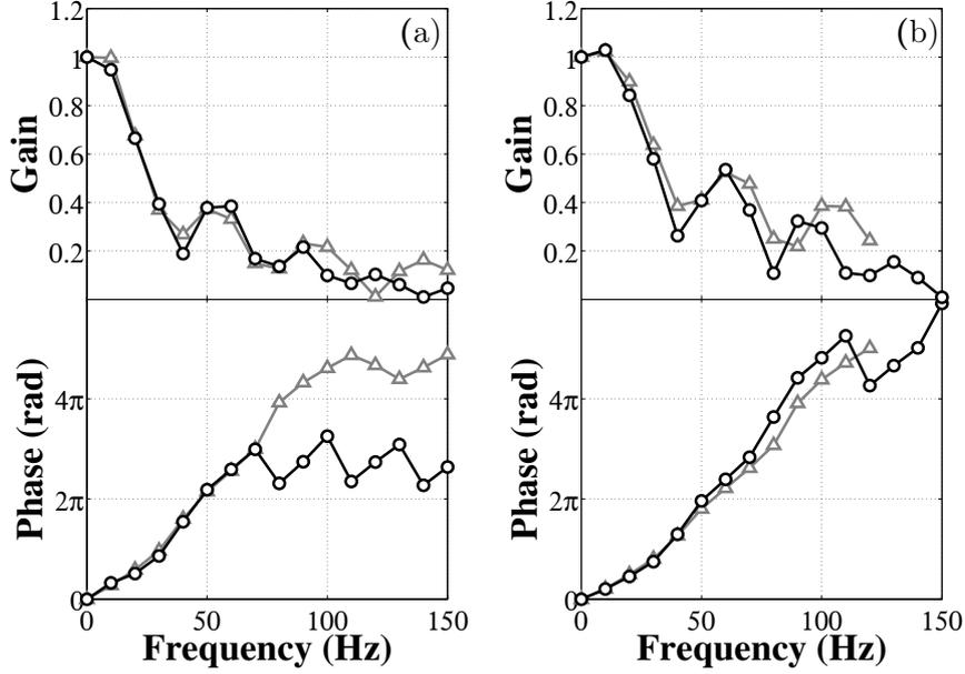
**Figure 3.3:** Flame Transfer Function gain (top) and phase (bottom) as a function of the acoustic perturbation frequency. (a) FTF measured on the 22mm-diameter burner exit with a 35 mm-diameter plateau.  $\phi = 1.1$ . Black line:  $v_0 = 1.3 \text{ m.s}^{-1}$  Grey line:  $v_0 = 2.5 \text{ m.s}^{-1}$  (b) FTF measured on the 22 mm-diameter burner exit with a 35mm-diameter confinement tube.  $\phi = 1.1$ . Black line:  $v_0 = 1.34 \text{ m.s}^{-1}$  Grey line:  $v_0 = 2.27 \text{ m.s}^{-1}$
