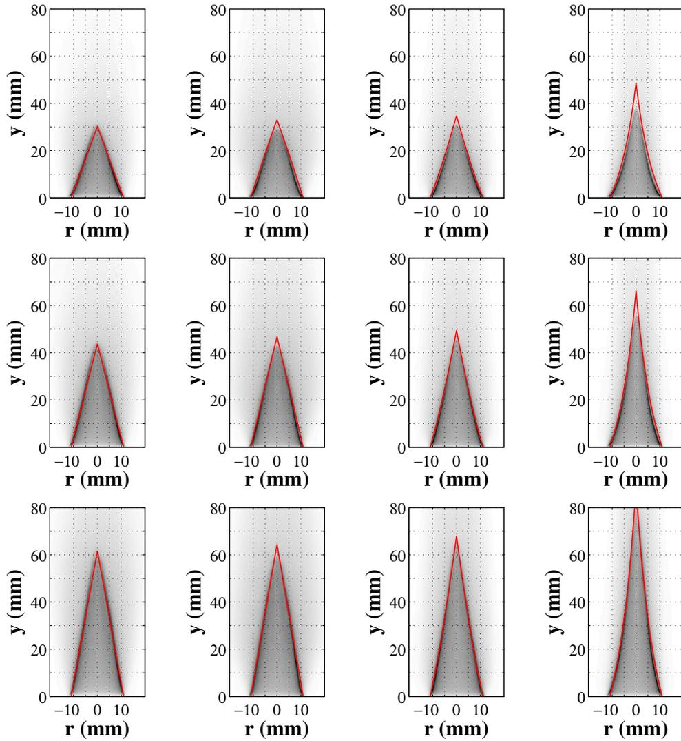
**Figure 6.8:** Flame images for different confinement tubes and flow conditions. From left to right :  $C_r = 0, 0.44, 0.60$  and  $0.81$ . Upper row:  $\dot{m} = 0.396 \text{ g.s}^{-1}$ . Middle row:  $\dot{m} = 0.566 \text{ g.s}^{-1}$ . Lower row:  $\dot{m} = 0.792 \text{ g.s}^{-1}$ . Predictions with Eq. (6.23) are plotted in red.
