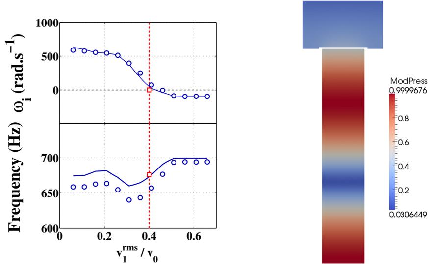
**Figure 8.9:** Left: Oscillation frequency  $f$  and growth rate  $\omega_i$  are plotted as a function of the perturbation level  $v_1^{\text{rms}}/v_0$ . Numerical results from AVSP ( $\circ$ ) and from LOM (-) are compared to experimental data ( $\square$ ) from [Boudy et al. (2011)]. Right: Pressure modulus distribution calculated by AVSP indicating the structure of the corresponding eigenmode at limit cycle.  $L_1 = 0.35$  m and  $l = 0.003$  m.
