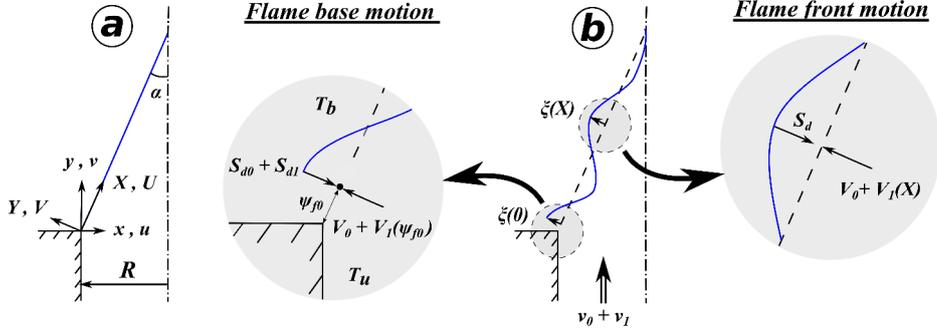
**Figure 4.1:** Schematic of the configuration investigated. (a) Steady conical flame along with the different frames used in this article. (b) Acoustically perturbed conical flame, with a focus on the flame base region and the flame front displacement far from the burner lip.
