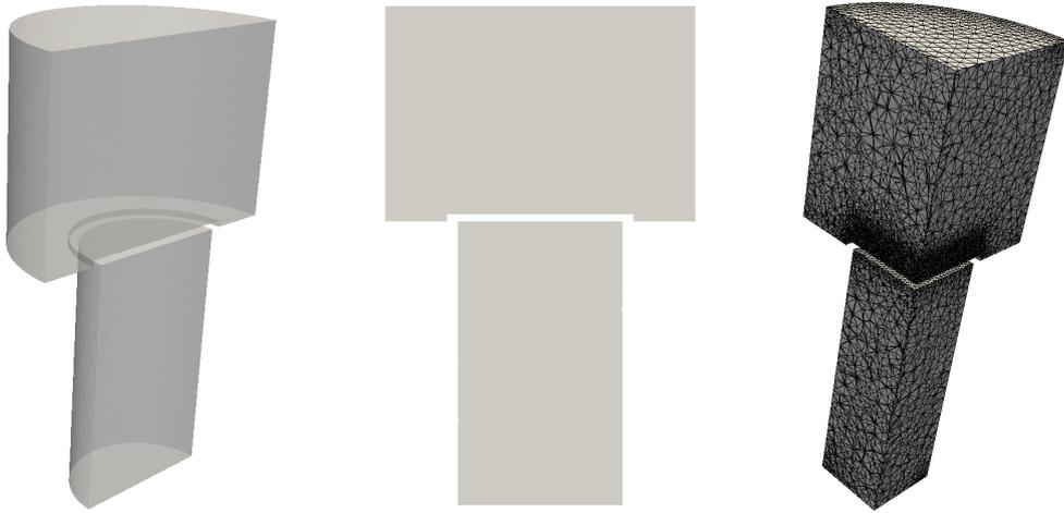
**Figure 8.2:** Numerical domain for  $L_1 = 0.12$  m,  $L_2 = 0.088$  m and  $l = 0.003$  m. **Left:** Half of the numerical domain. **Middle:** 2D vertical slice of the numerical domain. **Right:** The mesh is superimposed on a fourth of the numerical domain.
