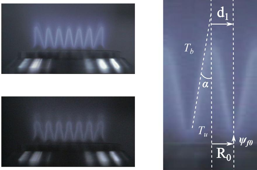
**Figure 6.17:** (left) Collection of conical flames anchored on a perforated plate: steady flames (top) and a snapshot of acoustically perturbed flames (bottom). (right) Zoomed image of the central flame used to determine some of the parameters used in the theoretical models.
