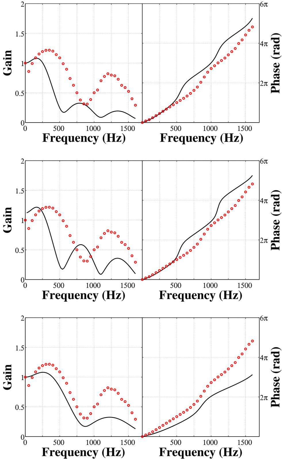
**Figure 6.18:** Comparisons between FTF measurements (red circles) and different FTF models (black lines). **(top)**  $F_A(\omega_*, \alpha)$ . **(center)**  $F_A(\omega_*, \alpha) + F_B(\omega_*, \alpha, \Psi_f, \delta_*, Ze)$ . **(bottom)**  $F_A(\omega_*^c, \alpha)$ .
