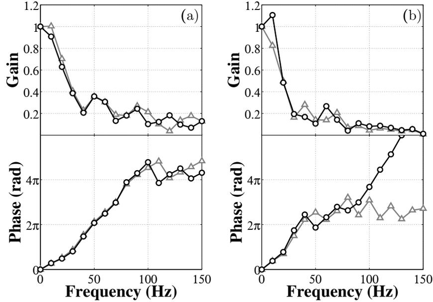
**Figure 3.2:** Flame Transfer Function gain (top) and phase (bottom) as a function of the acoustic perturbation frequency. (a) FTF measured on the 22 mm-diameter beveled burner exit.  $\phi = 1.1$ . Black line:  $v_0 = 1.3 \text{ m.s}^{-1}$  Grey line:  $v_0 = 2.5 \text{ m.s}^{-1}$  (b) FTF measured on the 30 mm-diameter beveled burner exit. Black line:  $v_0 = 1.27 \text{ m.s}^{-1}$ .  $\phi = 0.8$  Grey line:  $v_0 = 1.3 \text{ m.s}^{-1}$ .  $\phi = 1.1$ .
