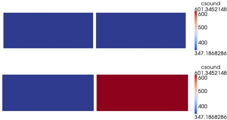
**Figure C.3:** Distribution of the speed of sound used for the calculations. Top figure:  $c_0 = 347\text{m.s}^{-1}$ . Bottom figure:  $c_0 = 347\text{m.s}^{-1}$  in the upstream cavity corresponding to  $T_1 = 300\text{ K}$  and  $c_0 = 601\text{m.s}^{-1}$  in the downstream cavity, corresponding to  $T_2 = 900\text{ K}$ .
