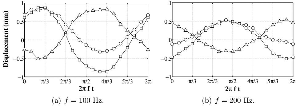
**Figure 5.5:** Flame base displacement as a function of the phase in the excitation cycle for a modulation amplitude of  $v_1^{\text{rms}}/v_0 = 0.1$ . The horizontal ( $\Delta$ ) and vertical displacements ( $\circ$ ) with respect to the steady flame location are represented, as well as the displacement in the normal direction with respect to the flame front ( $\square$ ).
