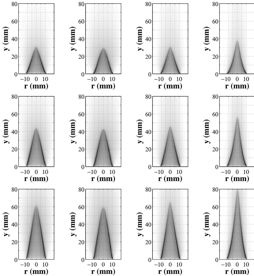
**Figure 6.3:** Flame images for different confinement tubes and flow conditions. From left to right :  $C_r = 0, 0.44, 0.60$  and  $0.81$ . Upper row:  $\dot{m} = 0.396 \text{ g.s}^{-1}$ . Middle row:  $\dot{m} = 0.566 \text{ g.s}^{-1}$ . Lower row:  $\dot{m} = 0.792 \text{ g.s}^{-1}$ .
