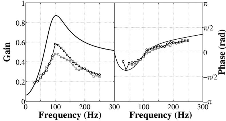
**Figure 5.8:** Transfer function  $\Xi(\omega)$  gain (left) and phase (right) as a function of the forcing frequency. The theoretical transfer function (black curve) is compared to measurements for two input levels  $v_1^{\text{rms}}/v_0 = 0.05$  (grey curve with square symbols) and  $v_1^{\text{rms}}/v_0 = 0.1$  (black curve with circle symbols).
