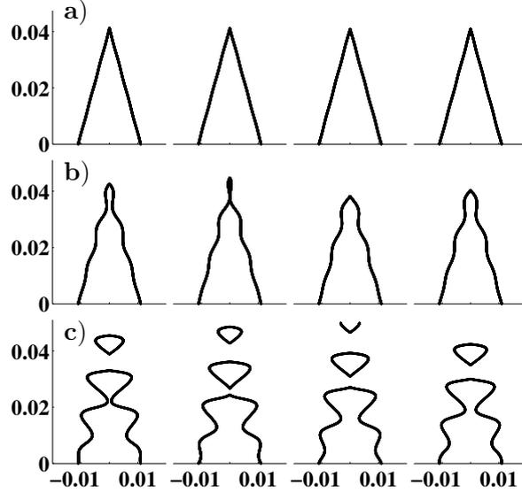
**Figure 4.4:** Flame shapes predicted with (a) a uniform velocity perturbation [Ducruix et al. (2000)]; (b) a convected velocity disturbance [Schuller et al. (2003a)]; (c) the model derived in the present chapter. The flame is presented for four different phases of the acoustic period, namely  $0$ ,  $\pi/2$ ,  $\pi$  and  $3\pi/2$ . Flame motions are calculated for  $\alpha = \pi/12$ ,  $|v_1/v_0| = 0.1$  and  $\omega_* = 20$ .
