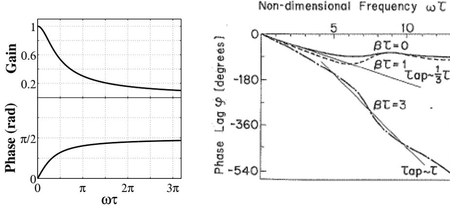
**Figure 1.2:** (left) FTF gain and phase lag from Eq. (1.4) as a function of the dimensionless frequency  $\omega\tau$ . (right) Phase of the FTF as a function of the dimensionless frequency  $\omega\tau$ , plotted for different values of  $\beta\tau$  (see Eq. (1.7)) [Sugimoto and Matsui (1982)]. The FTF phase lag decreases because the “exp( $i\omega t$ )” convention was adopted in this article.
