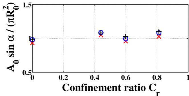
**Figure 6.6:** Evolution of the flame surface area  $A_0$  as a function of the confinement ratio. Measurements for three different mass flow rates:  $\dot{m} = 0.396 \text{ g.s}^{-1}$  (red cross);  $0.566 \text{ g.s}^{-1}$  (blue circles);  $0.792 \text{ g.s}^{-1}$  (black cross). The flame surface area is made dimensionless with the theoretical unconfined steady flame surface area  $A_0 = \pi R_0^2 / \sin \alpha$ .
