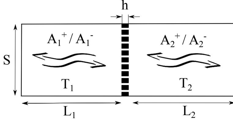
**Figure C.1:** Scheme of the theoretical validation case investigated. It comprise two cavities separated by a perforated plate of thickness  $h$ . The first (resp. the second) cavity is of temperature  $T_1$  (resp.  $T_2$ ) and of length  $L_1$  (resp.  $L_2$ ). Both cavities are of cross-section area  $S$ .
