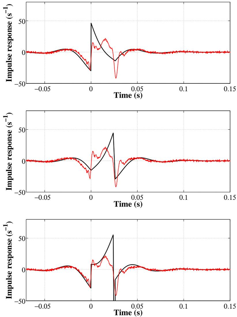
**Figure 4.13:** The filtered experimental impulse response (red curves) is plotted as a function of time and compared to predictions from different filtered models (black curves): uniform model (top), convective model (center) and incompressible convective model (bottom).  $\tau_r = 0.261 \text{ s}^{-1}$ .  $\tau_c = 0.240 \text{ s}^{-1}$ . Cut-off frequency of the high-pass filter:  $f_c = 20 \text{ Hz}$ .
