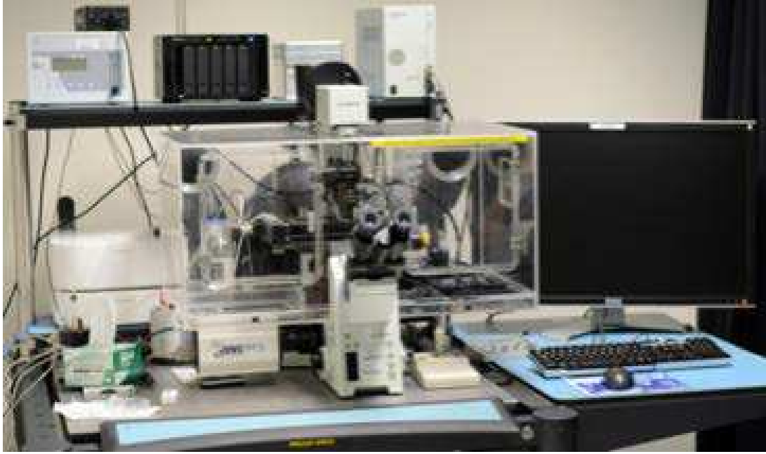
Figure 1-8: A*STAR IMB Phase-contrast microscope installation with incubator for living cells observation.
