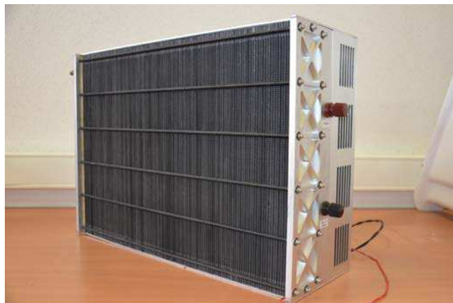
Fig. 2. A 5 kW commercial fuel cell stack consisting of 90 cells.
