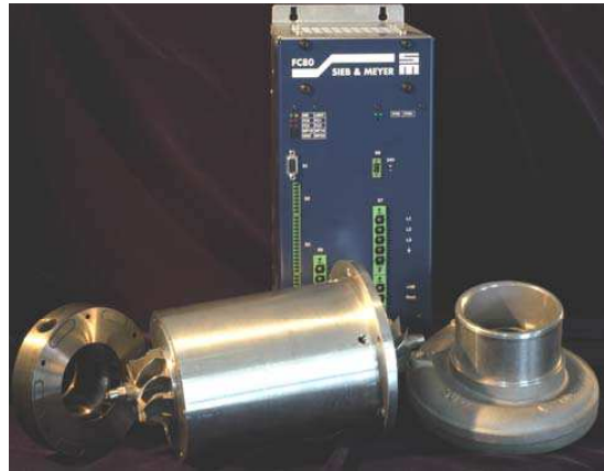
Fig. 14. A 12 kW centrifugal compressor with maximum speed of 120,000 rpm [30].
