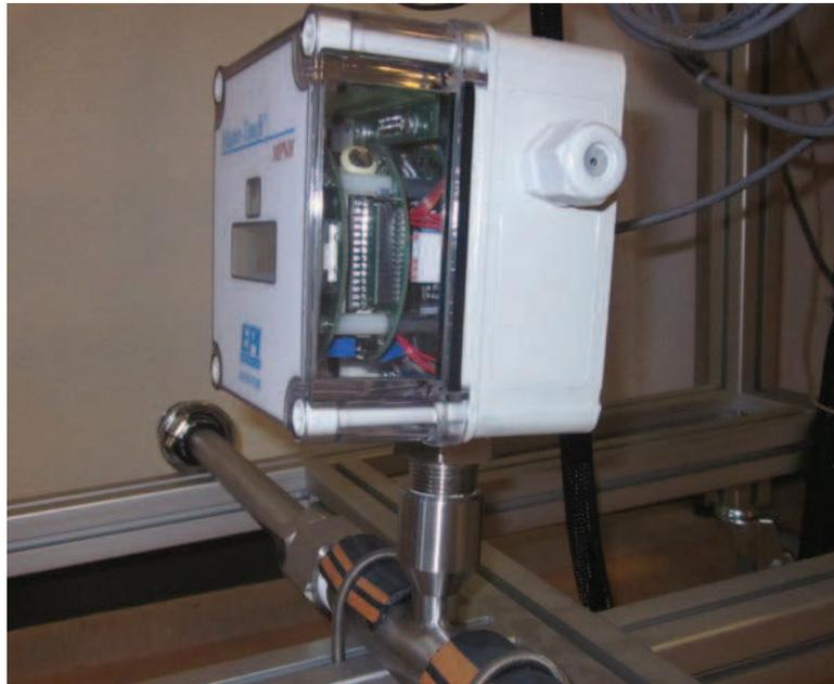
**Fig. 67.** Mass flow sensor.
