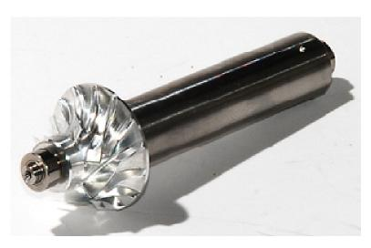
Fig. 17. Assembled rotor including impeller and high-speed ball bearings.
