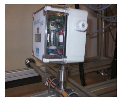
Fig. 67. Mass flow sensor.
