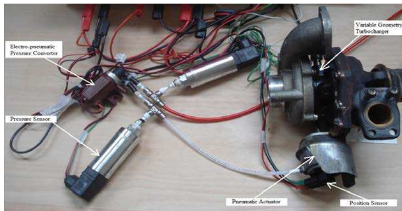
Figure 0.4. VGT with an electro-pneumatic actuator system
