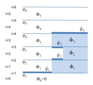
Figure 3.3: Side view of a section of the 1-D column showing the interpretation of porosity by CIM
