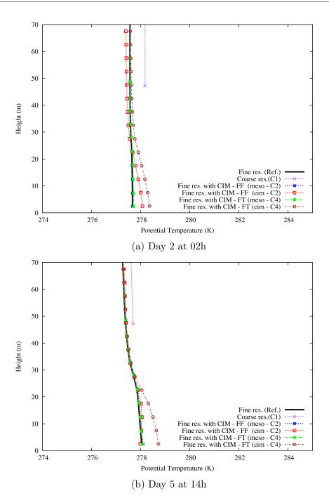
Figure 5.4: Profile of the potential temperature (K) using a fine resolution (Ref. bold black curve), coarse resolution (C1 - purple curve), fine resolution with CIM (meso - C2 - blue curve ; cim - C2 - red curve) and fine resolution with CIM - with no horizontal fluxes (meso - C4 - green curve ; cim - C4 - brown curve)
