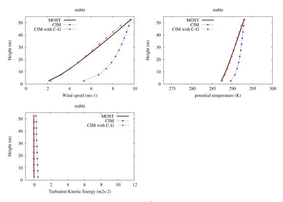
Figure 4.3: Comparison of wind (in  $ms^{-1}$ ), potential temperature (in K) and T.K.E (in  $m^2s^{-2}$ ) vertical profiles obtained with the MOST over a plane surface and with CIM (without and with the  $C_G$  correction in the T.K.E.) under stable conditions. Altitude is in meter.
