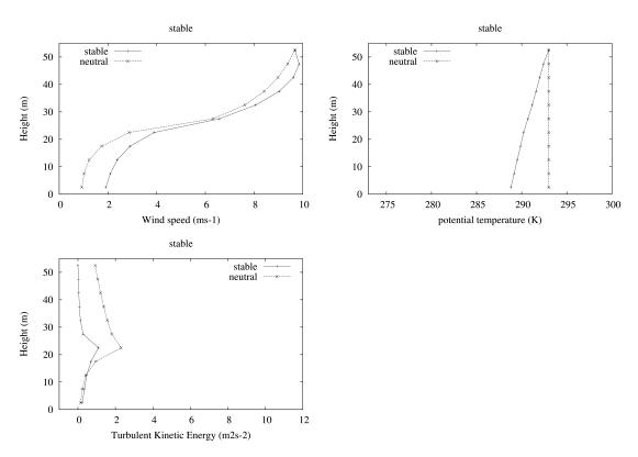
Figure 4.5: Comparison of wind (in  $ms^{-1}$ ), potential temperature (in K) and T.K.E (in  $m^2s^{-2}$ ) vertical profiles computed with CIM applied on a surface with obstacles under neutral and stable case atmospheric conditions
