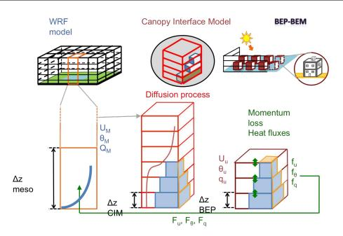
Figure 5.1: WRF scheme with the implementation of CIM (all in blue corresponds to WRF, in red variables corresponding to CIM and the fluxes are represented in green)
