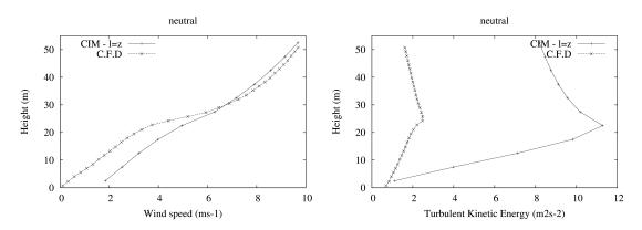
Figure 3.8: Comparison of the wind (in  $ms^{-1}$ ) and T.K.E (in  $m^2s^{-2}$ ) profiles obtained with obstacles from CIM and the C.F.D experiment with the mixing length equal to the height. Altitude is in meter.
