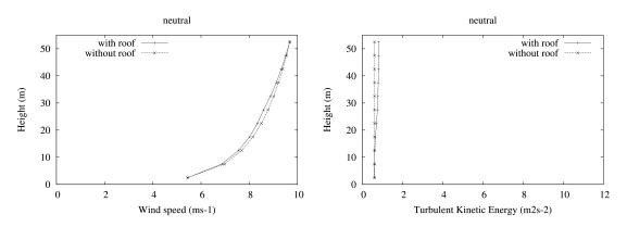
Figure 3.6: Comparison of the wind (in  $ms^{-1}$ ) and T.K.E (in  $m^2s^{-2}$ ) profiles computed to evaluate the impact of obstacles roof surfaces. Altitude is in meter.
