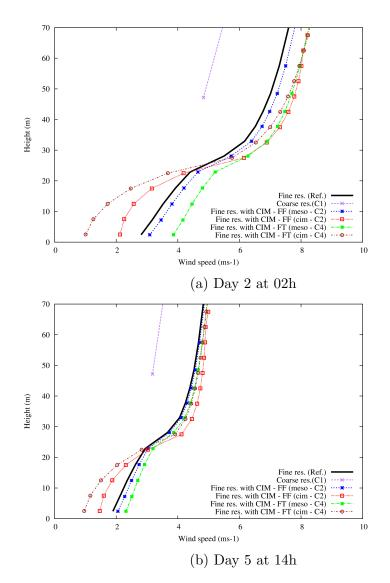
Figure 5.5: Profile of the wind speed  $(ms^{-1})$  using a fine resolution with WRF (Ref. - bold black curve), coarse resolution (C1 - purple curve), fine resolution with CIM (meso - C2 - blue curve ; cim - C2 - red curve) and fine resolution with CIM - with no horizontal fluxes (meso - C4 - green curve ; cim - C4 - brown curve)
