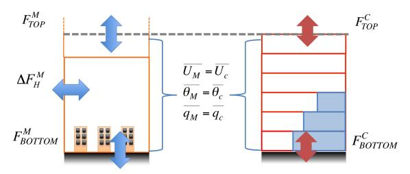
Figure 5.2: Representation of fluxes calculated on the vertical column in CIM (right) before correction and in the corresponding volume in WRF (left)
