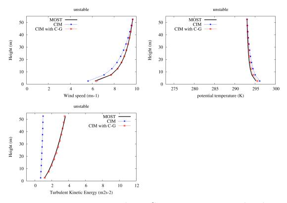
Figure 4.4: Comparison of wind (in  $ms^{-1}$ ), potential temperature (in K) and T.K.E (in  $m^2s^{-2}$ ) vertical profiles obtained with the MOST over a plane surface and with CIM (without and with the  $C_G$  correction in the T.K.E.) under unstable conditions. Altitude is in meter.
