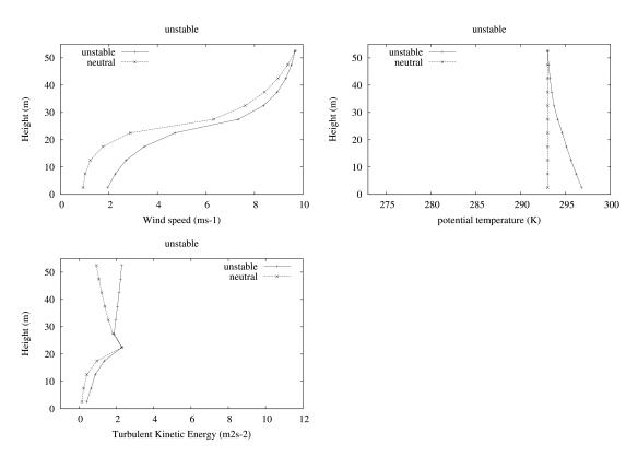
Figure 4.6: Comparison of wind (in  $ms^{-1}$ ), potential temperature (in K) and T.K.E (in  $m^2s^{-2}$ ) vertical profiles computed with CIM applied on a surface with obstacles under neutral and unstable case atmospheric conditions
