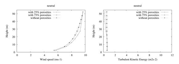
Figure 3.5: Comparison of the wind (in  $ms^{-1}$ ) and T.K.E (in  $m^2s^{-2}$ ) profiles computed to evaluate the impact of the obstacle porosities (with 25% and 75% of empty space in a grid cell). Altitude is in meter.
