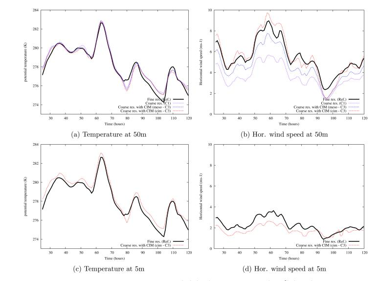
Figure 5.3: Comparison of the potential temperature (K) (left) and wind speed  $(ms^{-1})$  (right) computed using WRF without and with the coupling of CIM at 50m (top) and at 5m (bottom). Black lines refer to reference simulation (Ref.), purple refer to C1, blue line refer to meso-scale values from C3 (meso - C3) and red line refer to CIM values from C3 (cim - C3). Horizontal axis represents the time, in hours, after the start of the simulation
