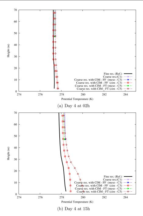
Figure 5.6: Profile of the potential temperature (K) using a fine resolution with WRF (Ref. - bold black curve), coarse resolution (C1 - purple curve), coarse resolution with CIM (meso - C2 - blue curve ; cim - C2 - red curve) and coarse resolution with CIM - with no horizontal fluxes (meso - C4 - green curve ; cim - C4 - brown curve)
