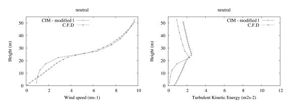
Figure 3.9: Comparison of the wind (in  $ms^{-1}$ ) and T.K.E (in  $m^2s^{-2}$ ) profiles obtained with obstacles from CIM and the C.F.D using the mixing length as given by Eq. (3.39) from Santiago and Martilli [2010]. Altitude is in meter.
