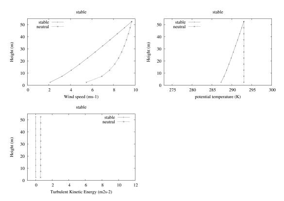
Figure 4.1: Comparison of wind (in  $ms^{-1}$ ), potential temperature (in K) and T.K.E (in  $m^2s^{-2}$ ) vertical profiles obtained with the MOST over a plane surface in neutral and stable cases. Altitude is in meter.
