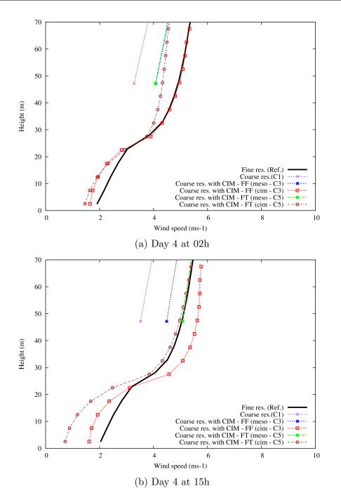
Figure 5.7: Profile of the wind speed  $(ms^{-1})$  using a fine resolution with WRF (Ref. - bold black curve), coarse resolution (C1 - purple curve), coarse resolution with CIM (meso - C2 - blue curve ; cim - C2 - red curve) and coarse resolution with CIM - with no horizontal fluxes (meso - C4 - green curve ; cim - C4 - brown curve)
