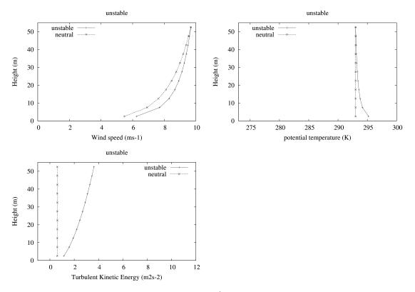
Figure 4.2: Comparison of wind (in  $ms^{-1}$ ), potential temperature (in K) and T.K.E (in  $m^2s^{-2}$ ) vertical profiles obtained with the MOST over a plane surface in neutral and unstable cases. Altitude is in meter.
