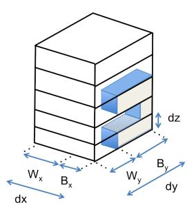
Figure 3.2: Integration of obstacles inside CIM ( $B_x$  and  $B_y$  are the building length and  $W_x$  and  $W_y$  are the street width in the x and y-directions respectively. dx and dy are the horizontal grid resolution while dz is the vertical resolution)
