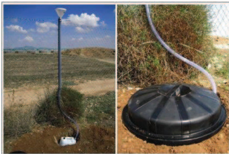
Figure 9 : Details of the sampling device for the analysis of stable isotopes in precipitation. The black tap was finally painted in white.
