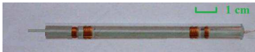
Fig. 34 shows the detail of as-prepared sample holder containing thin capillary and series of four pick-up coils wound around it.
