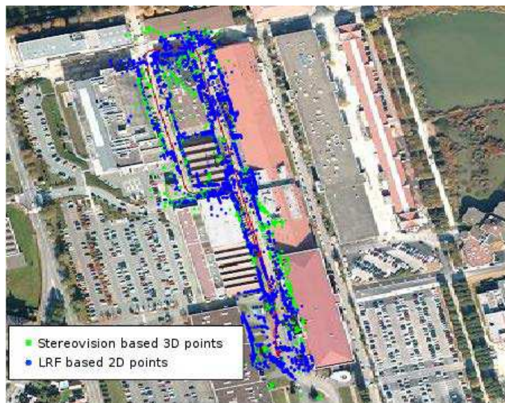
FIGURE 3.21 – Landmarks from the stereoscopic system and from the LRF are overlapped on Google aerial image
