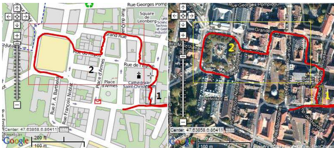
FIGURE 5.37 – Vehicle trajectory overlapped on the OpenStreetMap and Google aerial image
