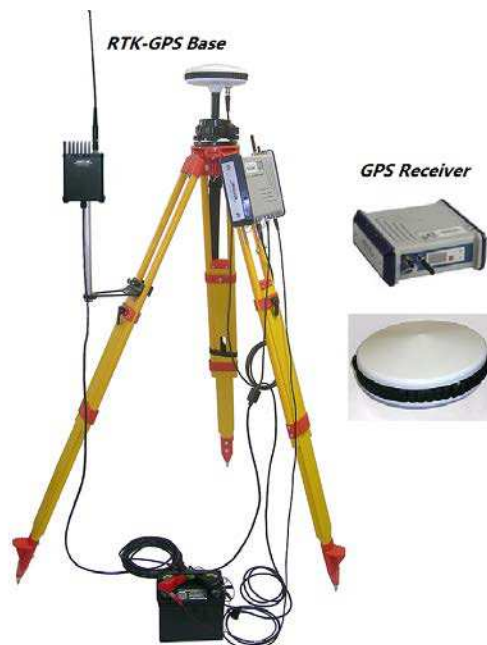
FIGURE 3.20 – Fixed GPS base used for sending corrections to the mobile GPS receiver
