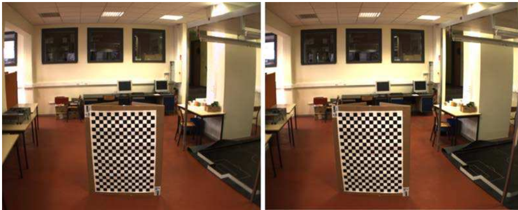
FIGURE 3.2 – Chessboard images used for camera calibration
