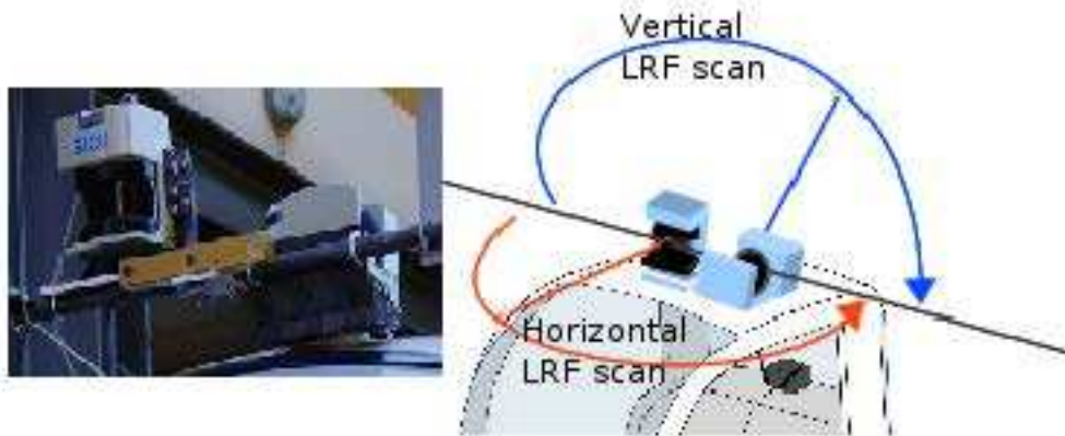
FIGURE 5.3 – Two LRF systems are mounted on the roof of the vehicle : the vertical LRF scan is in blue and the horizontal LRF scan is in red
