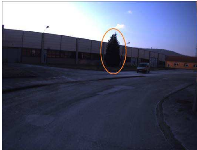
FIGURE 5.47 – One tree in front of the building is treated as an independent object by the LRF-V (corresponding to the object in the yellow circle of Fig. 5.46)
