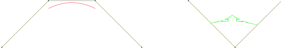
Figure 3.13: Left: a cubic spline with 4 control points. Right: a fractal curve with 3 control points.
