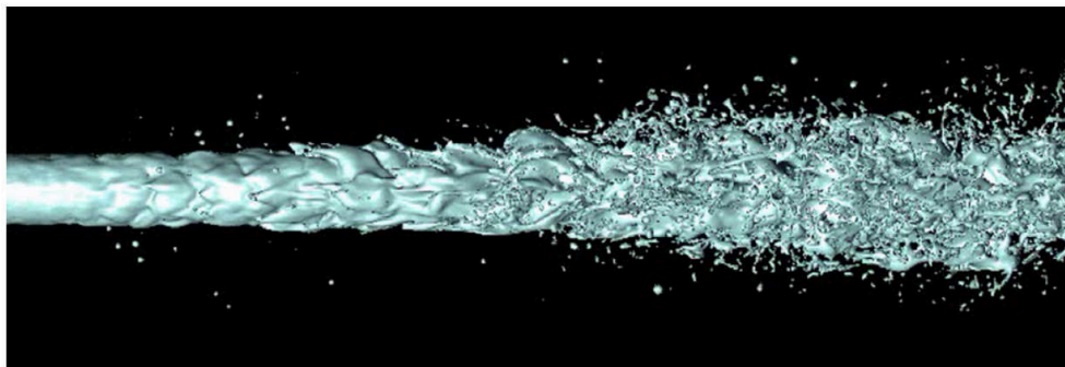
Figure 4.20 : DNS of the primary breakup of a turbulent jet, from [231]
