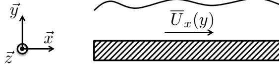
Figure 4.3 : Unidirectional mean film flow configuration
