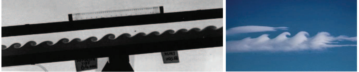
Figure 4.2 : Illustration of Kelvin-Helmholtz instability at different length scales. Left: Kelvin-Helmholtz instability located at two different fluids interface, from [340] (scale \approx 1 cm). Right: instability between different atmospheric layers, illustrated by clouds (scale \approx 1 km).
