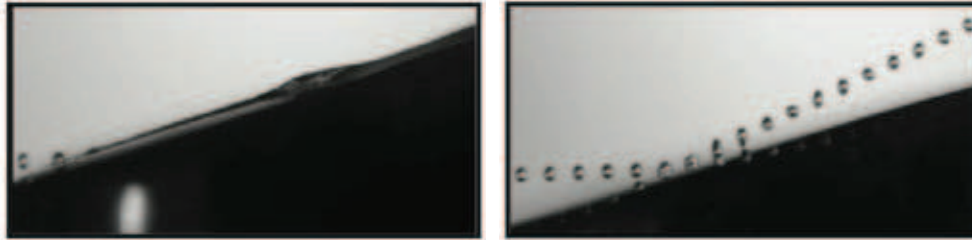
Figure 2.1 : Photograph of isolated droplet/wall interaction in filming (left) and rebound (right) regimes, from [6]
