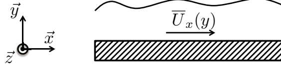
Figure 4.3 : Unidirectional mean film flow configuration
