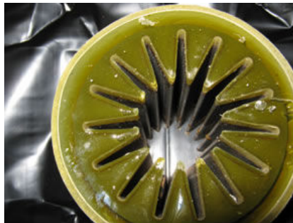
Figure 1.5: Star-shaped grain of a P230 1/35 sub-scale test motor named LP10 (source: ONERA).
