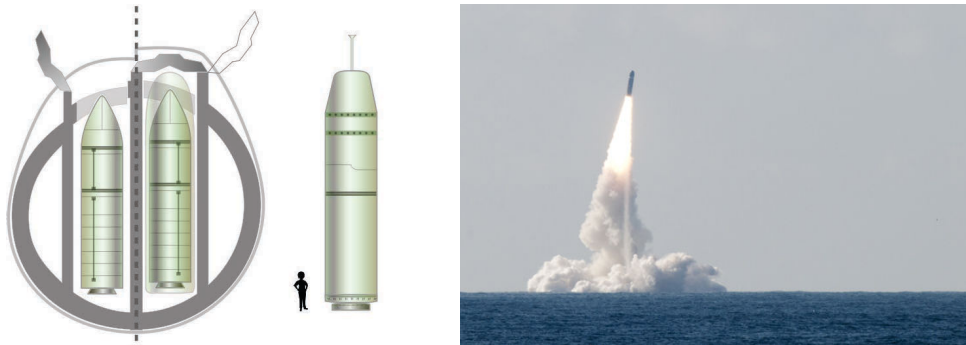
Figure 1.8: Left: M_4 in a submarine; Middle: M51 (source: Wikipedia) – Right: M51 test firing (source: DGA).
