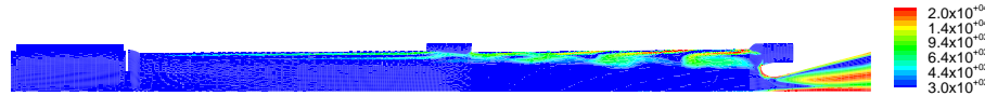
Figure 15.11: Gaseous phase vorticity module ( s^{-1} ) with monodisperse solid particles at t = 0.514 s.
