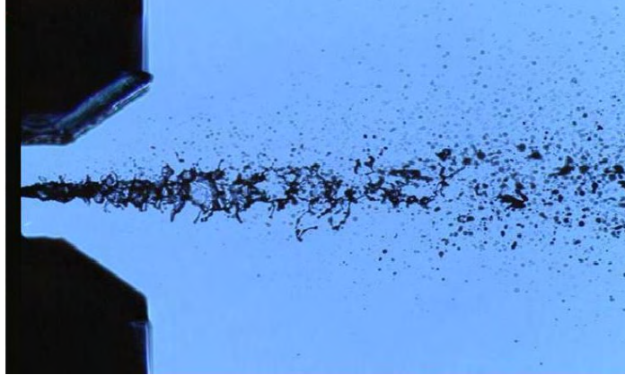
Figure 3.3: Generation of a polydisperse spray from the primary atomization of a jet – Experiment by C. Dumouchel (CORIA).
