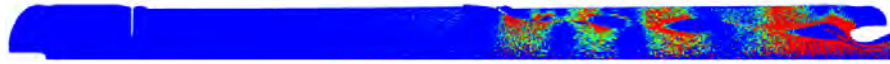
Figure 1.19: Collision rate in the P230 SRM– 2D Lagrangian computation from Estivalezes (2010) with the CEDRE code (ONERA).
