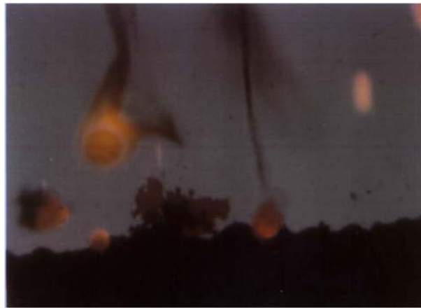
Figure 1.22: Ignited aluminum droplets ejected from the propellant surface. (source: ONERA).
