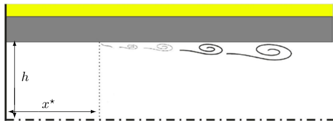
Figure 1.34: Illustration of the parietal vortex shedding (VSP).
