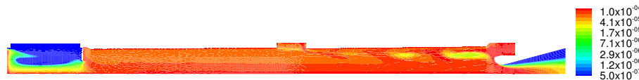
Figure 15.12: Volume fraction for solid monodisperse particles with d_{30} = 6.5 \mu\text{m} at t = 0.514 s.
