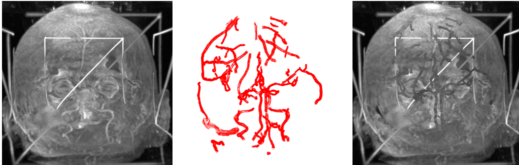
Figure 3.23: Our RBT algorithm applied to MRA data (left). The dense sampling produced on 37 vessels (middle) and the tracked vessels superimposed upon the original data (right).
