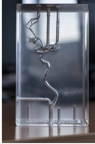
Figure 5.5: The silicon vascular network used for validation.
