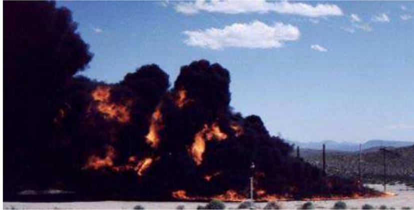
Figure IV.18 Instantaneous view of the experiment flame and smoke from a video camera for medium wind ( $U_0=5.4$  m/s)
