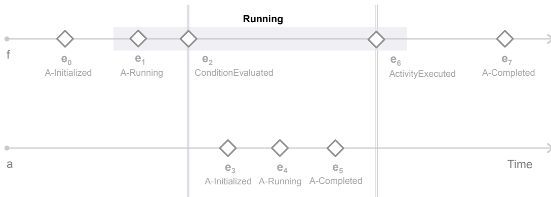
Figure 4.13 Event trace produced by the normal execution of an IF activity instance
