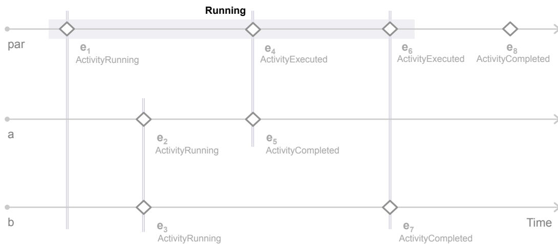
Figure 4.20 Event trace produced by a normal execution of a Parallel activity instance
