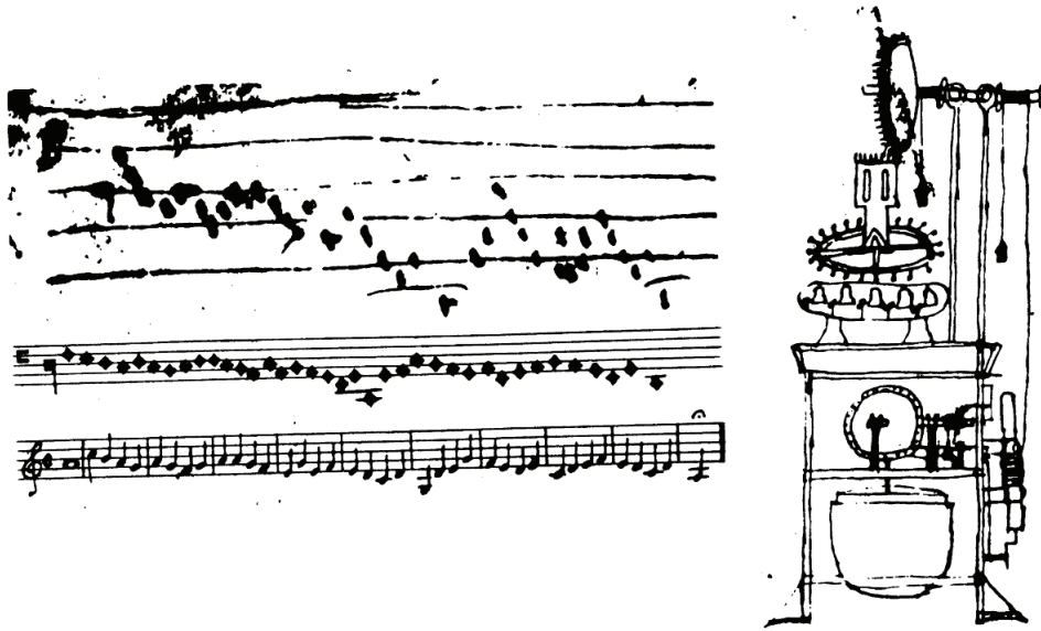
Figure 1.3: The Flute Player schema of the Musa brothers, reconstructed by [Farmer, 1931] (From [Koetsier, 2001])
