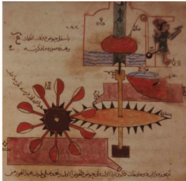
Figure 1.4: A schema showing a part of the Arbiter for a Drinking Session. (From al-Jazari book).
