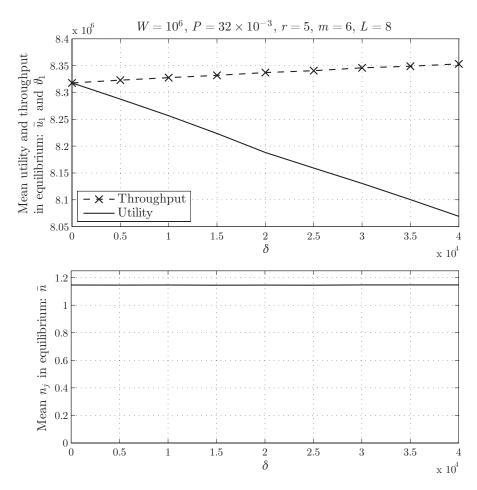
Figure 8.3: Mean utility, throughput and number of mobiles sharing the same BS with respect to pricing in case of Rayleigh and path loss model.
