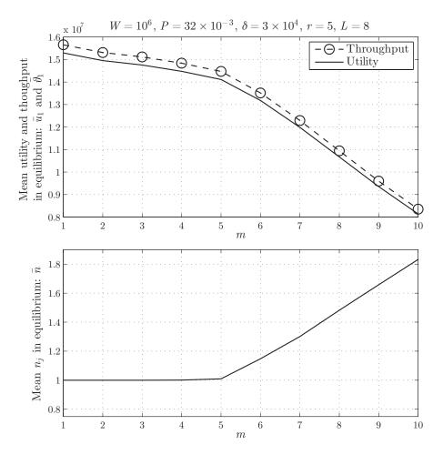
Figure 8.4: Mean utility, throughput and number of mobiles sharing the same BS with respect to *m* in case of Rayleigh and path loss model.
