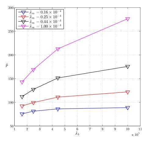
Figure 4.5: The DCC Algorithm: Change of the average total power  $\bar{p}$  with respect to intensity of BSs  $\lambda_b$  for increasing values of intensity of mobiles  $\lambda_m = (0.16, 0.25, 0.44, 1.00) \times 10^{-4} \, \frac{points}{m^2}, A = 4 \, km^2, P_0 = 12 \, W.$
