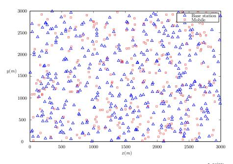
Figure 4.2: Distribution of BSs and mobiles in Euclidean plane.  $\lambda_b=44.4\times 10^{-5}~\frac{points}{m^2}$ ,  $\lambda_m=2.5\times 10^{-5}~\frac{points}{m^2}$ .
