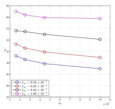
Figure 4.4: The CC Algorithm: Change of the average total power  $\bar{p}$  with respect to intensity of BSs  $\lambda_b$  for increasing values of intensity of mobiles  $\lambda_m = (0.16, 0.25, 0.44, 1.00) \times 10^{-4} \frac{points}{m^2}, A = 4 \ km^2, P_0 = 12 \ W.$
