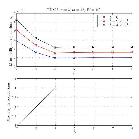
Figure 8.6: Mean utility, throughput and number of mobiles sharing the same BS with respect to  $\mathcal L$  in case of TDMA for Scenario 2.
