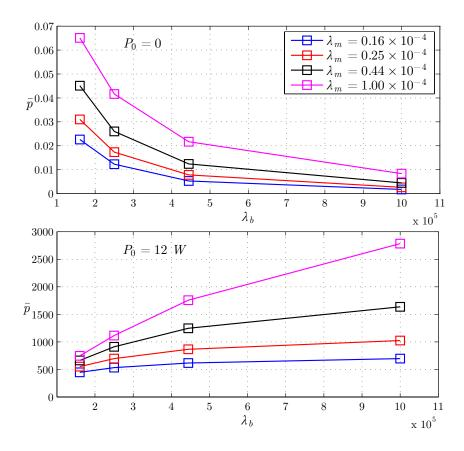
Figure 4.3: The NBS Algorithm: Change of the average total power  $\bar{p}$  with respect to intensity of BSs  $\lambda_b$  for increasing values of intensity of mobiles  $\lambda_m = (0.16, 0.25, 0.44, 1.00) \times 10^{-4} \frac{points}{m^2}, A = 4 \ km^2$ .
