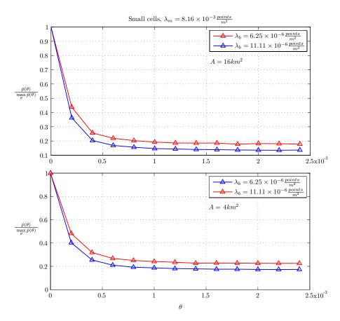
Figure 4.8: Small cells: Change of the normalized average total power with respect to  $\boldsymbol{\theta}$
