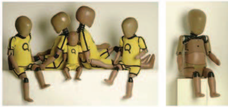
Figure 1.2: Q set child dummy family, from left to right: Q1.5, Q3, Q0, Q6, Q1 and Q1 without suit (de Jager et al., 2005).
