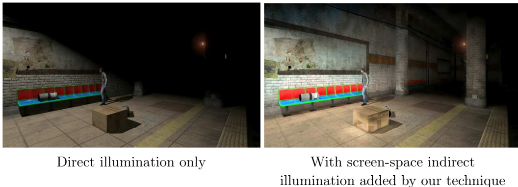
Figure 3.12: Our method to compute screen-space indirect illumination was successfully used in the pipeline of the game Alone In The Dark , developed by Eden Games.
