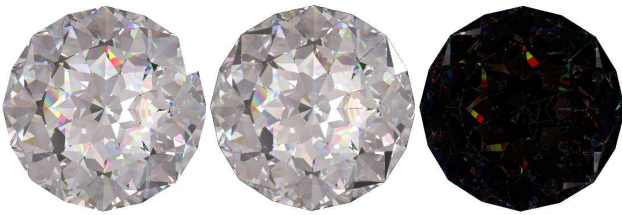
Figure 8: Image of a highly dispersive stone, computed using exact refraction with our ray tracer ( top left ) and with our hardware algorithm with one facet tree ( top right ). Left : a difference image shows that some—but not all, as explained in the text—rainbow effects are missed by our algorithm in this case.
