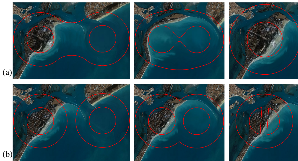
FIGURE 4.2: Two fisheye merging. (a) flat-tops with the same magnification factor merge, requiring similar magnification factor; (b) flat-tops with distinct magnification factors are cropped.
