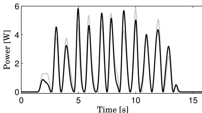
Figure 5.46: Power input into the gripper on the vertical axis (black) with no intended trajectory. In grey is the power dissipated by the damping part, i.e.  $bv_z^2$ . The stiffness part does not reduce the power input at all.
