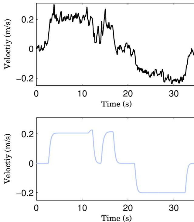
Figure 3.15: Velocities of the object on the robot's frontal axis: the admittance controller output  $\dot{\mathbf{X}}$  in black (top), robot desired velocity  $\dot{\mathbf{X}}_d$  in light blue (bottom). The role switching occurs at around  $t = 20s$ .
