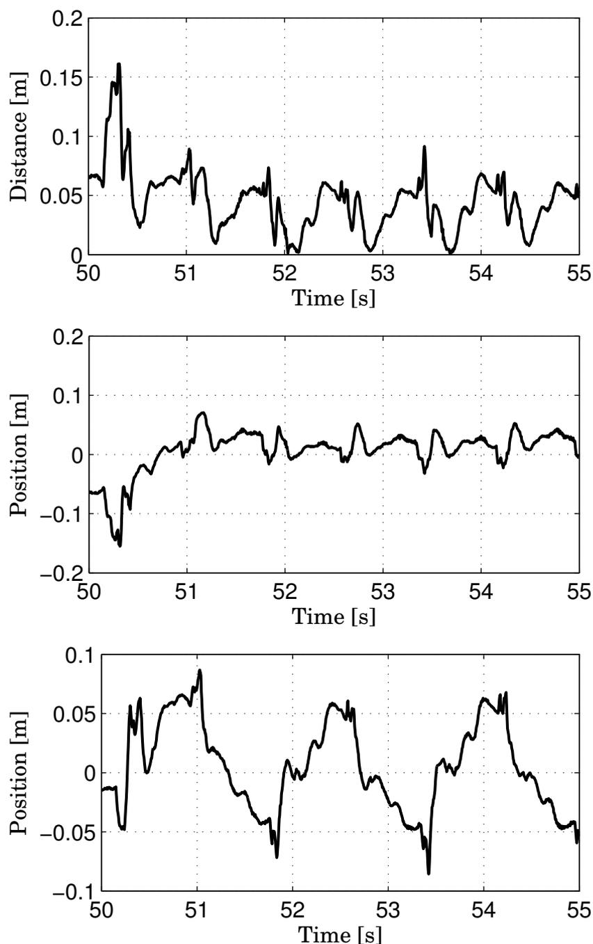
Figure 5.18: Distance to weighted middle point (top) and vector ZMP-weighted middle point ( $x$  and  $y$  components: middle and bottom respectively), between  $t = 50s$  and  $t = 55s$ . The total experiment goes from  $t = 45s$  to  $t = 80s$ . These values are less discontinuous than the two previous sets of data.
