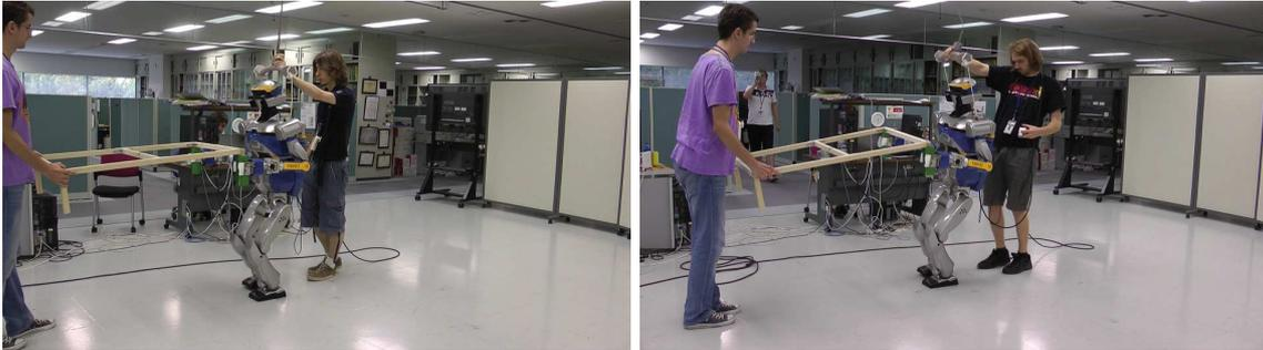
Figure 5.26: Test scenario with the stabilizer on (left) and off (right). The robot remains straight with the stabilizer on while it is leaning dangerously without it. The operator behind the robot has to assist in stabilizing the robot by stretching the ropes that are holding the robot in case it is falling.
