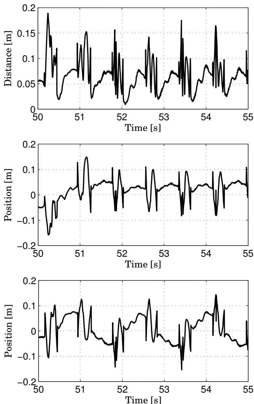
Figure 5.16: Distance to geometric middle point (top) and vector ZMP-geometric middle point ( $x$  and  $y$  components: middle and bottom respectively), between  $t = 50\text{s}$  and  $t = 55\text{s}$ . The total experiment goes from  $t = 45\text{s}$  to  $t = 80\text{s}$ . These values are highly discontinuous, too.
