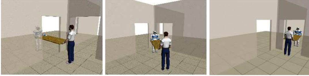
Figure 3.1: Example of scenario. The human-robot dyad has to carry the table through two doors that form a  $90^\circ$  angle. The dimensions of the table are too big to perform the task with a single bend, so that the human has to pass backward through the first door and forward through the second one. The human assumes the leadership of the task as he is walking backward through the first door, and then is guided by the robot through the second door.
