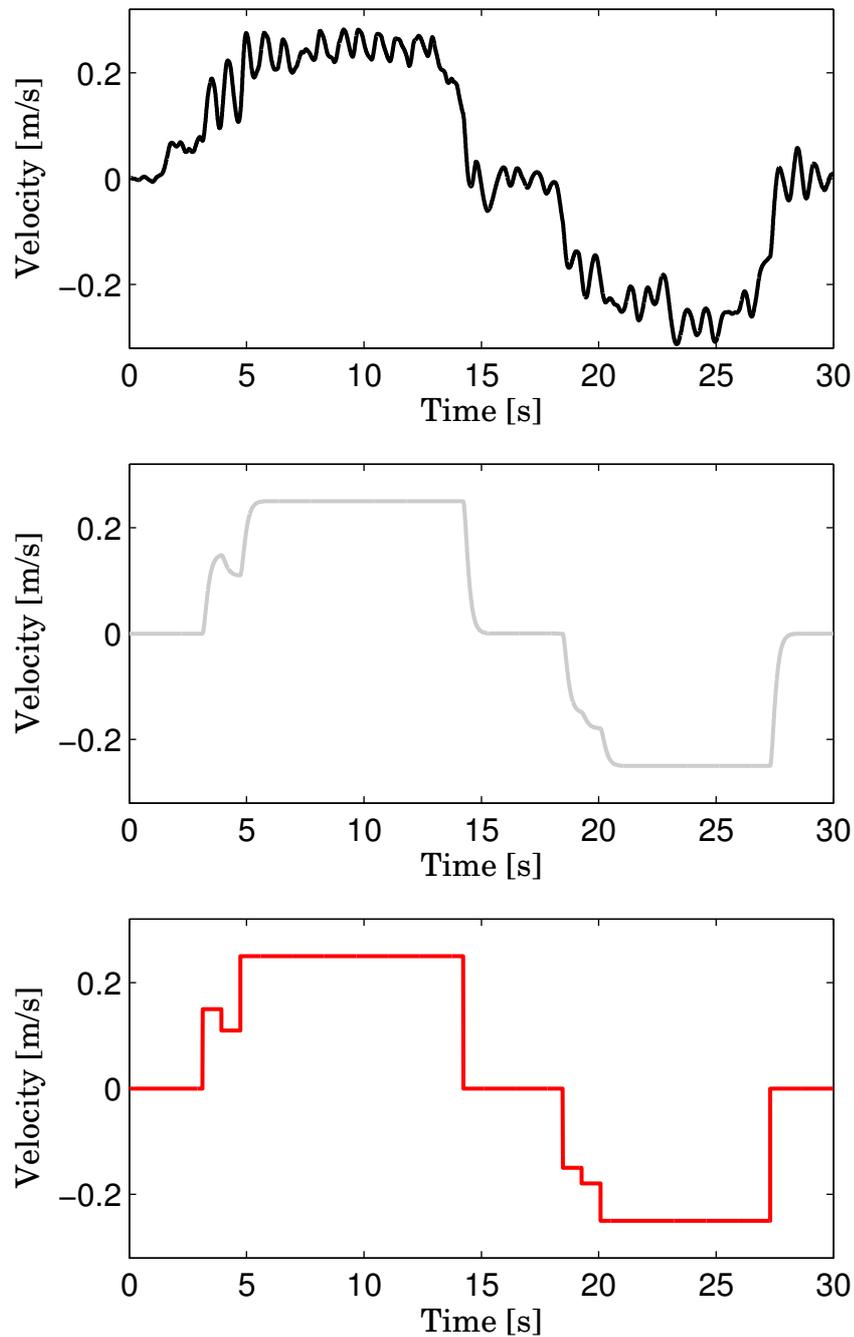
Figure 3.8: Velocities of the object: the admittance controller output  $\dot{\mathbf{X}}$  in black (top), follower desired velocity  $\dot{\mathbf{X}}_d$  in gray (middle), motion primitives  $\mathcal{V}$  in red (bottom).
