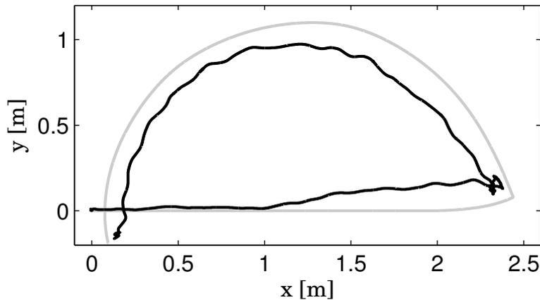
Figure 5.37: Trajectories of the robot's gripper in the XY plan: the admittance controller output  $\mathbf{X}$  in black, follower desired trajectory  $\mathbf{X}_d$  in grey. The motion starts at  $(0,0)$  towards the positive  $x$ . In a second time, the human guides the robot in a half-circular trajectory back to  $(0,0)$ .
