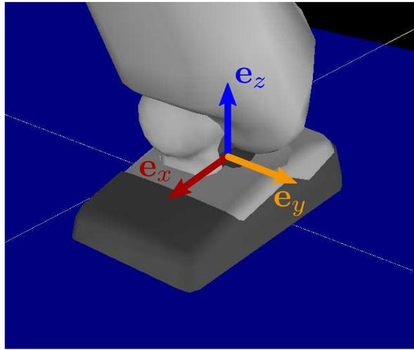
Figure 5.12: Foot local frame. It is chosen so that the  $z$ -axis is confounded with the gravity axis when walking on a horizontal floor. Besides the  $x$ -axis is the forward direction, thus making the  $y$ -axis the lateral direction.
