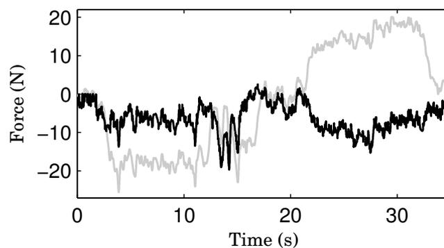
Figure 3.16: Force applied by the robot on the object (black) on the robot's frontal axis. The gray curve represents the damping part of the interaction force  $\mathbf{F} = -B\dot{\mathbf{X}}$ : it is the force that would be applied by the robot with a passive behavior. The role switching occurs at around  $t = 20s$ .
