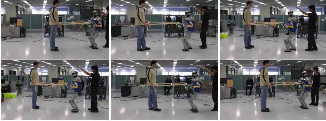
Figure 3.6: HRP-2 realizing the 1D transportation task as a proactive follower with a human partner, walking forwards (first line) and then backwards (last line).
