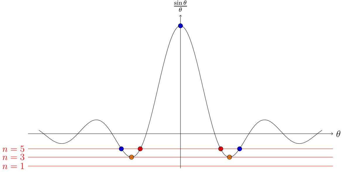
Figure A.1: Number of equilibrium positions  $n$  depending on the value of  $\frac{k_a}{kl^2}$ . The equilibrium position  $\theta_{eq} = 0$  is counted in  $n$ . Stable equilibrium positions are picture by a blue dot, while metastable and unstable equilibrium positions are pictured with orange and red dots respectively.
