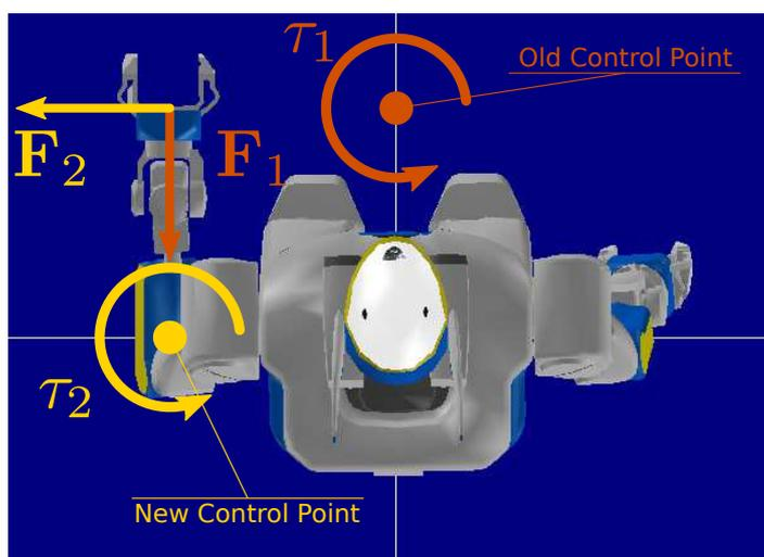
Figure 5.35: Old and new control points. With the old control point, a frontal force  $F_1$  applied on the left gripper results in a torque  $\tau_1$  at the control point. With the new control point, a lateral force  $F_2$  applied on the left gripper results in a torque  $\tau_2$  at the control point
