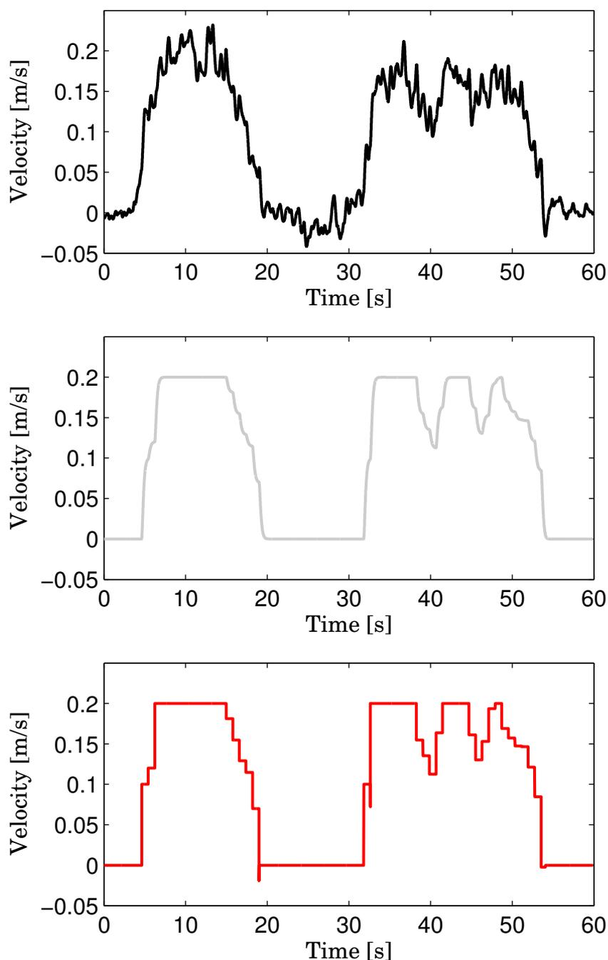
Figure 5.38: Velocities of the gripper on the robot's frontal axis: the admittance controller output  $\dot{\mathbf{X}}$  in black (top), robot desired velocity  $\dot{\mathbf{X}}_d$  in grey (middle) and velocity plan  $\mathcal{V}$  (bottom).
