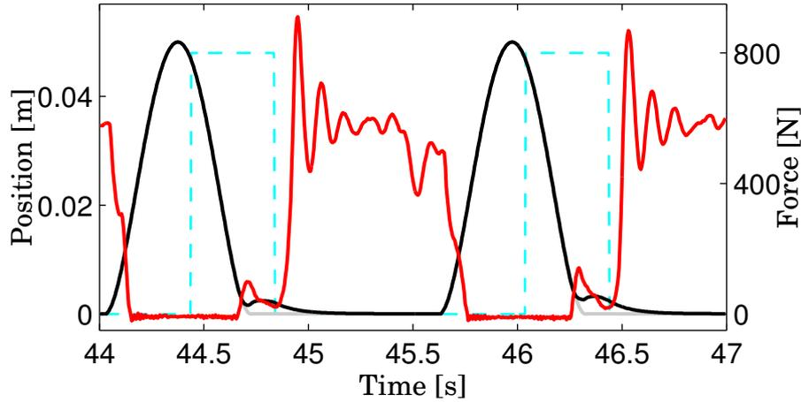
Figure 5.27: Example of inputs and outputs of the right foot impedance control. The vertical force  $f_z$  applied on the foot is in red (right scale), the desired trajectory  $z_d$  generated by WPG is in grey (left scale). The output trajectory  $z$  of the impedance controller is in black (left scale). The dotted light blue line is a multiple of the gain  $g$ . When it is positive, impedance control is active, when it is zero, impedance control is inactive and  $z$  converges towards  $z_d$ .
