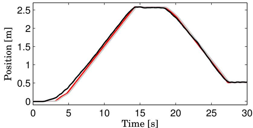
Figure 3.7: Trajectories of the object: the admittance controller output  $X$  in black, follower desired trajectory  $X_d$  in gray, motion primitives  $\mathcal{X}$  in red (integral of  $\mathcal{V}$ ).
