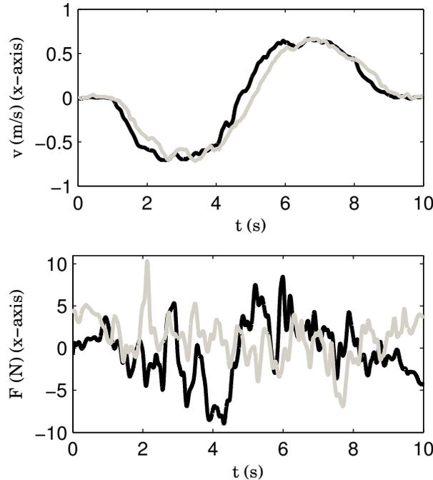
Figure 2.15: The top figure shows the velocity of the object on the  $x$ -axis in two consecutive trials with the same dyad (black, then gray curve). The curves are almost identical. The bottom figure shows the force applied on the object on the  $x$ -axis by the same subject in the same two consecutive trials. No evident force pattern can be identified.
