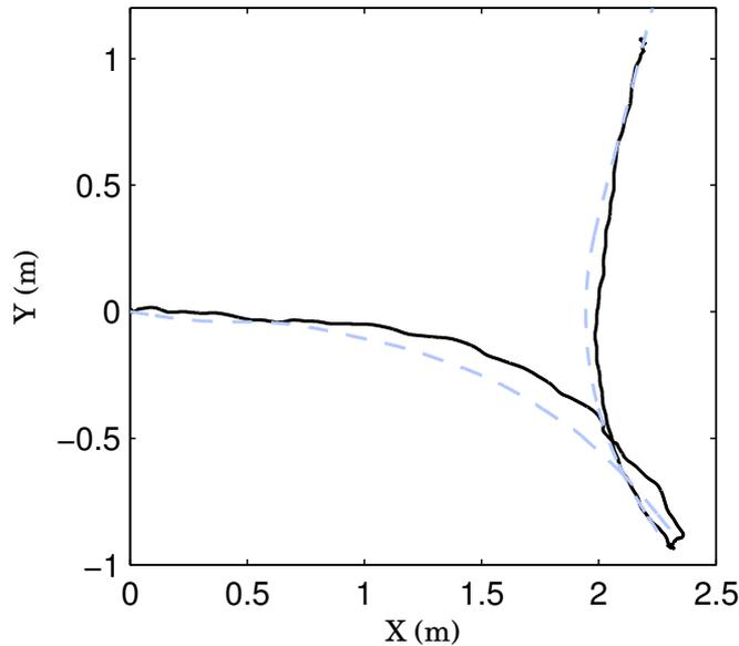
Figure 3.14: Trajectories of the object in the XY plan: the admittance controller output  $\mathbf{X}$  in black, follower desired trajectory  $\mathbf{X}_d$  in dotted light blue. The transportation starts at  $(0, 0)$  and ends around  $(2, 1)$ . The role switching occurs when the object is around  $(2.3, -1)$ .
