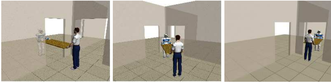
Figure 1.8: Example of pHRI task. The human-robot dyad has to carry the beam through two doors that form a 90^\circ angle. The dimensions of the beam are too big to perform the task with a single bend, so that the human has to pass backward through the first door and forward through the second one.
