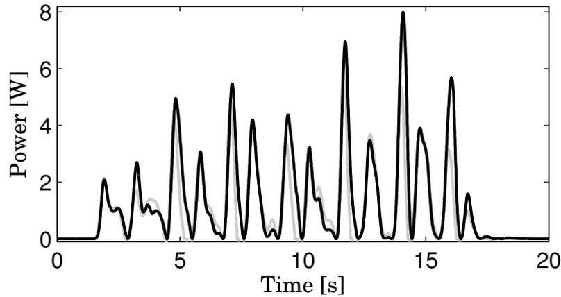
Figure 5.43: Power input into the gripper on the vertical axis (black) with the proactive control scheme. In grey is the power dissipated by the damping part, i.e.  $bv_z^2$ . The proactive control does not reduce the power input at all.
