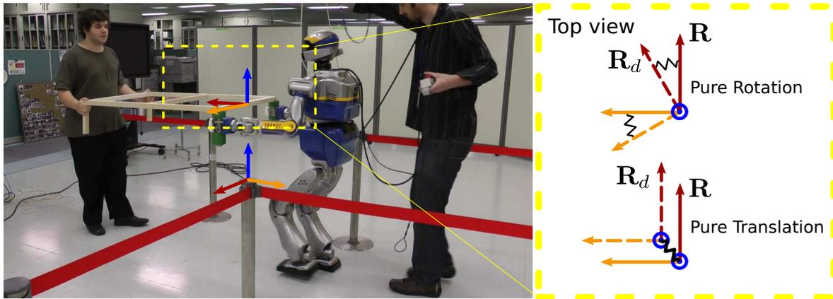
Figure 3.12: Important frames used in our 3D control scheme ( $x$  in red,  $y$  in orange,  $z$  in blue). The first one is the fixed global world frame that is visible in the foreground of the picture. The two other ones are attached to the object and are pictured within the yellow rectangle. The frame  $\mathbf{R}$  is rigidly linked to the object while the frame  $\mathbf{R}_d$  is linked to the object by the impedance. The latter one is the impedance nodic reference.
