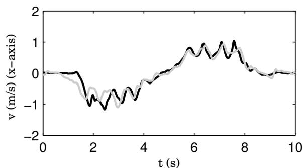
Figure 2.12: Velocities of hip markers in the motion direction ( $x$ -axis) for subject 1 (black, RASl) and subject 2 (gray, LASl). The oscillations in the velocities are caused by the gait. The oscillations in both subjects' hip velocities synchronize after a few steps.
