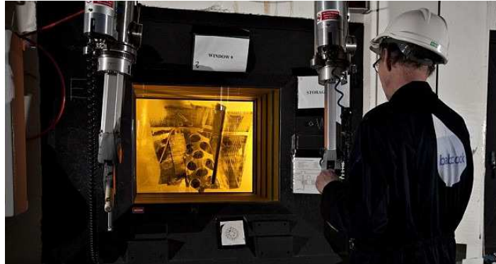
Figure 1.1: Example of telerobotics in hazardous environments. Employees at the Dounreay's Prototype Fast Reactor site in Caithness, Scotland, are forced to use robotic arms because of the high levels of radiation on the glass.
