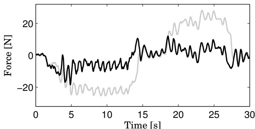
Figure 3.9: Force applied by the robot on the object (black). The gray curve represents the damping part of the interaction force  $\mathbf{F} = -B\dot{\mathbf{X}}$ : it is the force that would be applied by the robot with a passive behavior to obtain the same velocity.
