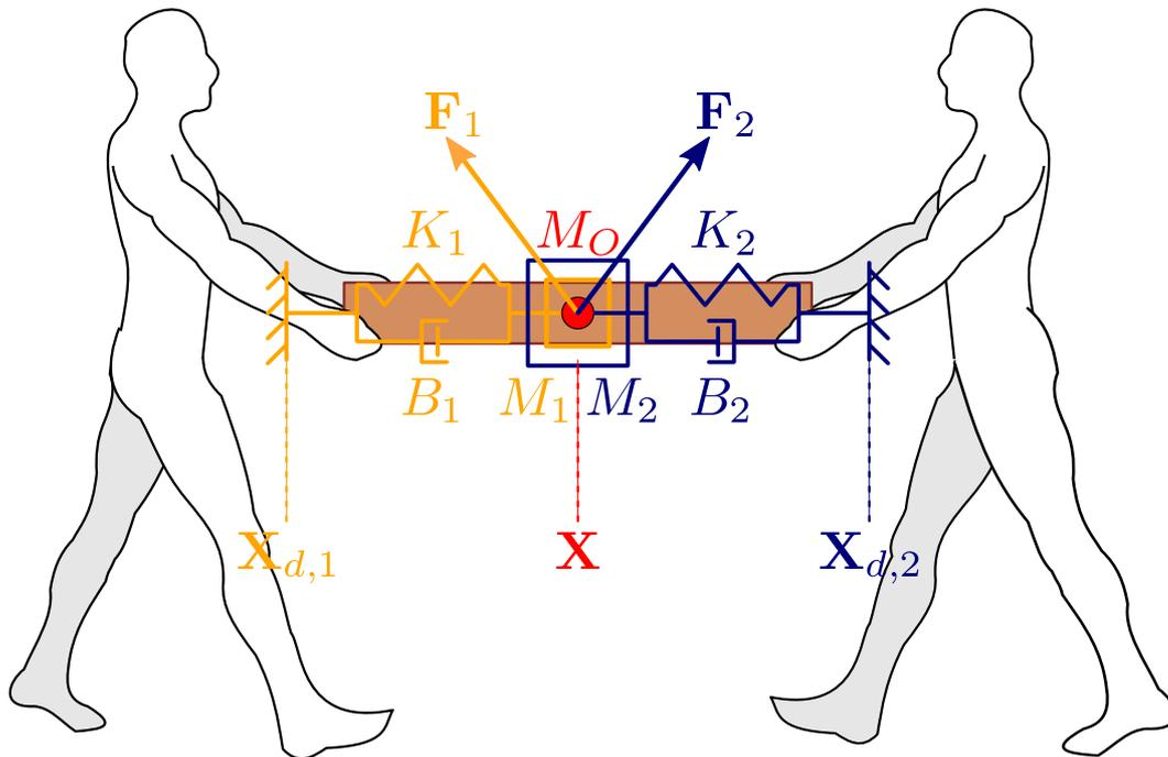
Figure 1.10: Impedance constraint example for collaborative object manipulation.
