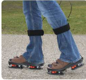
Figure 2.3: ForceShoe™ system. Each shoe is composed of two force sensors and two motion sensors.
