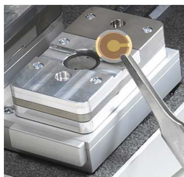
Figure 11: AT-cut quartz (source http://www.q-sense.com )
