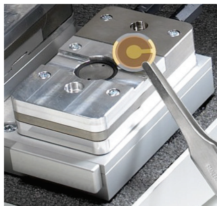
Figure I-4: AT-cut quartz crystal for QCM, electrode side, above a sample chamber (source http://www.q-sense.com )
