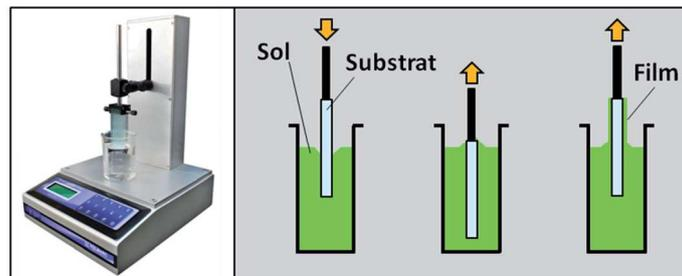
Fig. I.15 - Montage de dip-coating.
