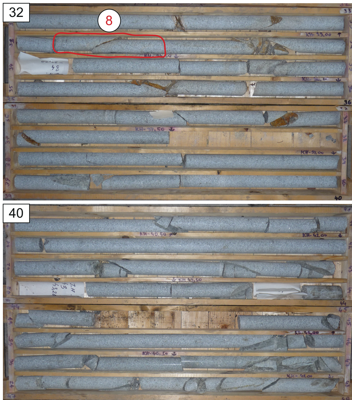
Figure A2 (continued). Position of the borehole core samples within the borehole core. The core with diameter 4.45 cm is stocked by meters. The numbers in top left corner of the photographs indicate the upper borehole level (m) of the sequence.
