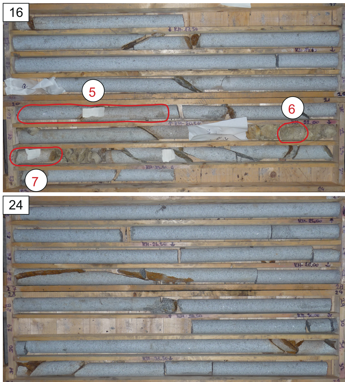
Figure A2 (continued). Position of the borehole core samples within the borehole core. The core with diameter 4.45 cm is stocked by meters. The numbers in top left corner of the photographs indicate the upper borehole level (m) of the sequence.
