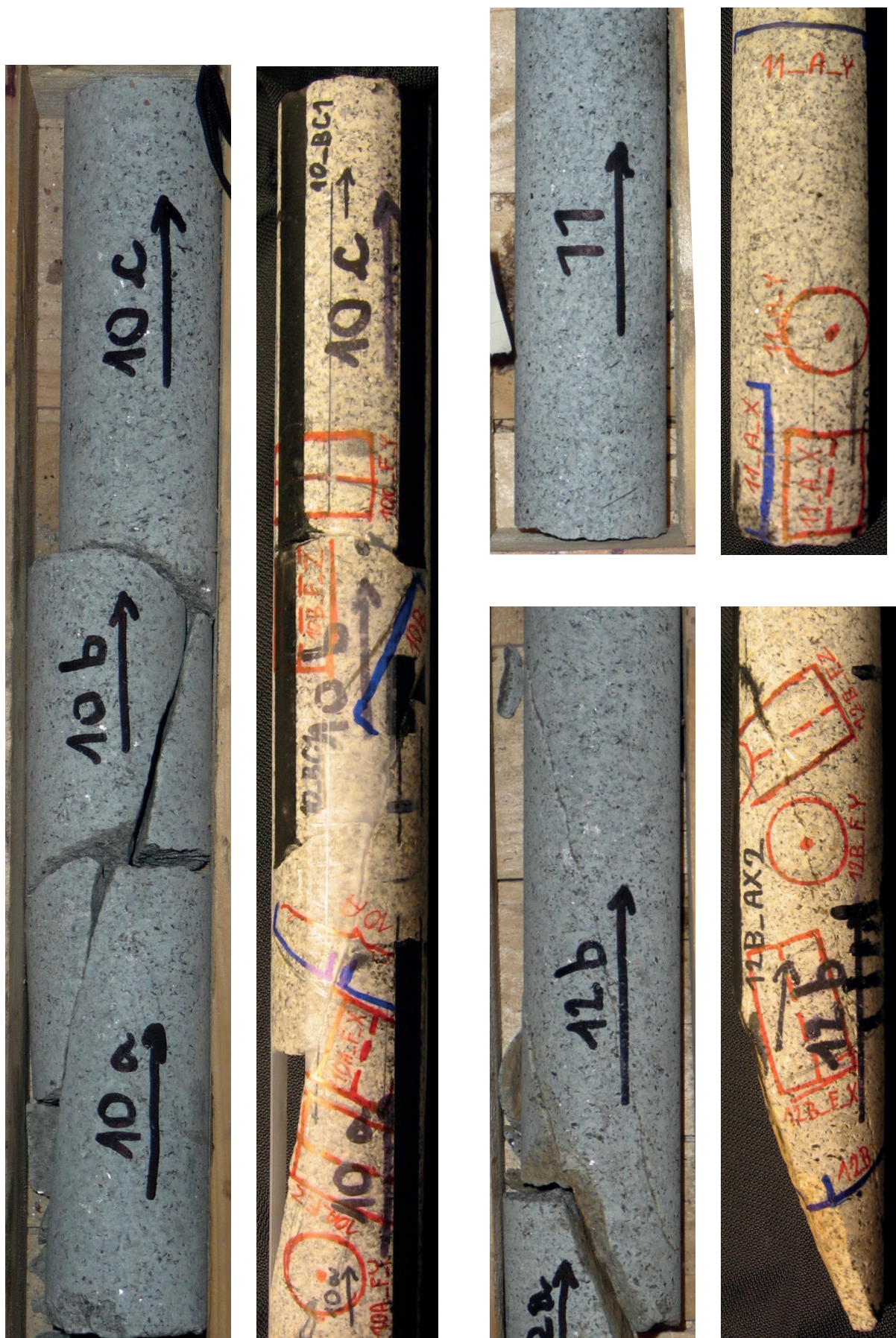
Figure A1 (continued). Borehole core samples shown on photographs taken prior to extraction from the core boxes (left) and after marking of position of the TC scanning profiles and of the plugs for permeability and V_p measurements (right).
