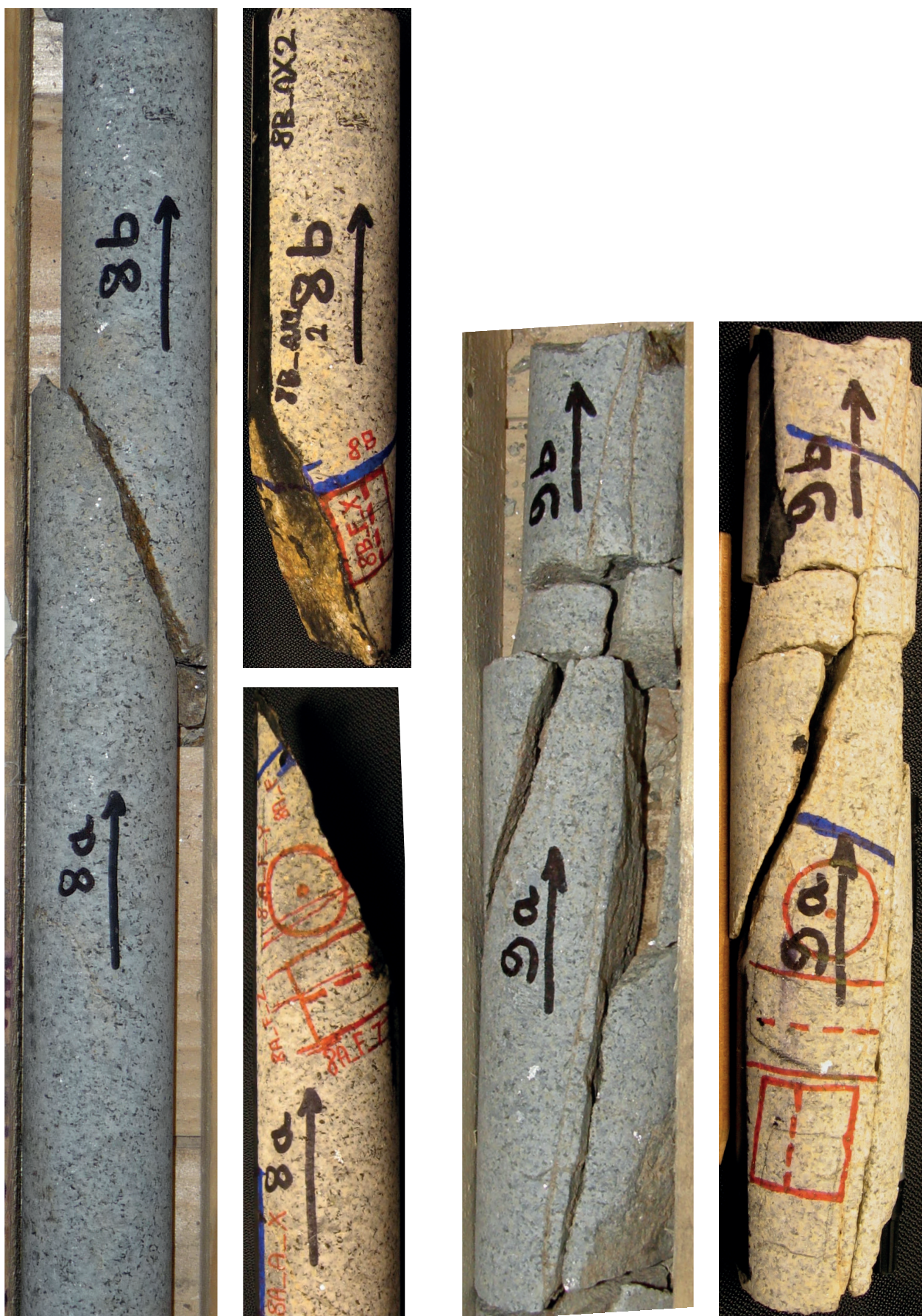
Figure A1 (continued). Borehole core samples shown on photographs taken prior to extraction from the core boxes (left) and after marking of position of the TC scanning profiles and of the plugs for permeability and V_p measurements (right).
