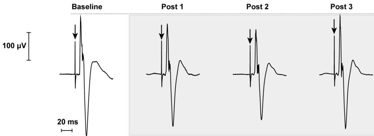
Figure 2. Average waveform of diaphragm motor-evoked potentials (DiMEPs) for a single subject evoked by single-pulse TMS over the motor cortex at baseline and at 3 time-points following the inhibitory protocol (cTBS) over the SMA. Arrows indicate the time of stimulation.
