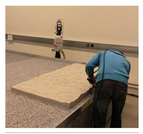
Figure 5.14 – Mock-up lying on the granit table and being scanned for DEM at DLR
