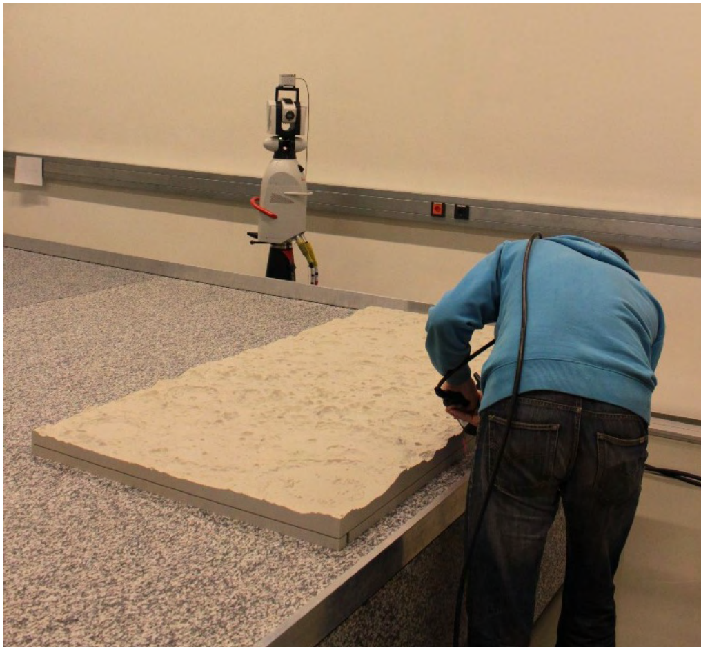
Figure 5.14 – Mock-up lying on the granit table and being scanned for DEM at DLR
