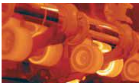
Figure 3.2: Thermal image of suspected roller [Flir, 2011]
