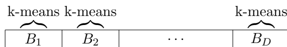
Figure 4.5: Illustration of the PQ procedure on one vector. The vector is considered as a product of D subvectors of equal length, and each subvector is quantized separately using a k -means algorithm on the database \mathcal{X} .
