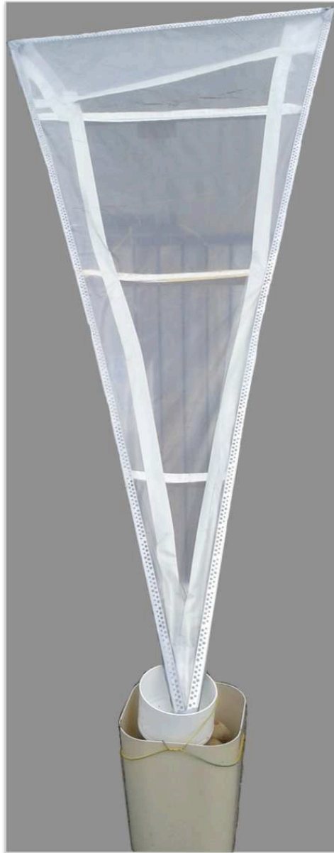
Figure 1: Rain collector constituted a conic polyan canvas cover (about 1.875 m 2 in surface area), allowing rainwater to flow through a 0.5 mm nylon filter in a 150 mL Büchner funnel to be collected in a 2 L polyethylene sterile container.
