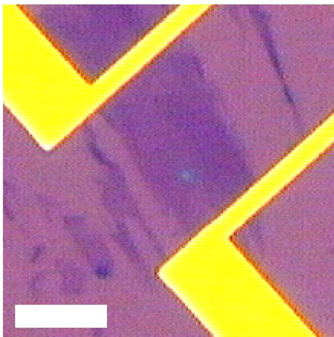
**Figure 5.2.** Optical image of a FLG deposited on a Si/SiO<sub>2</sub> substrate and Contacted with Ti/Pd (5/50 nm). Scale bar: 10 μm.
