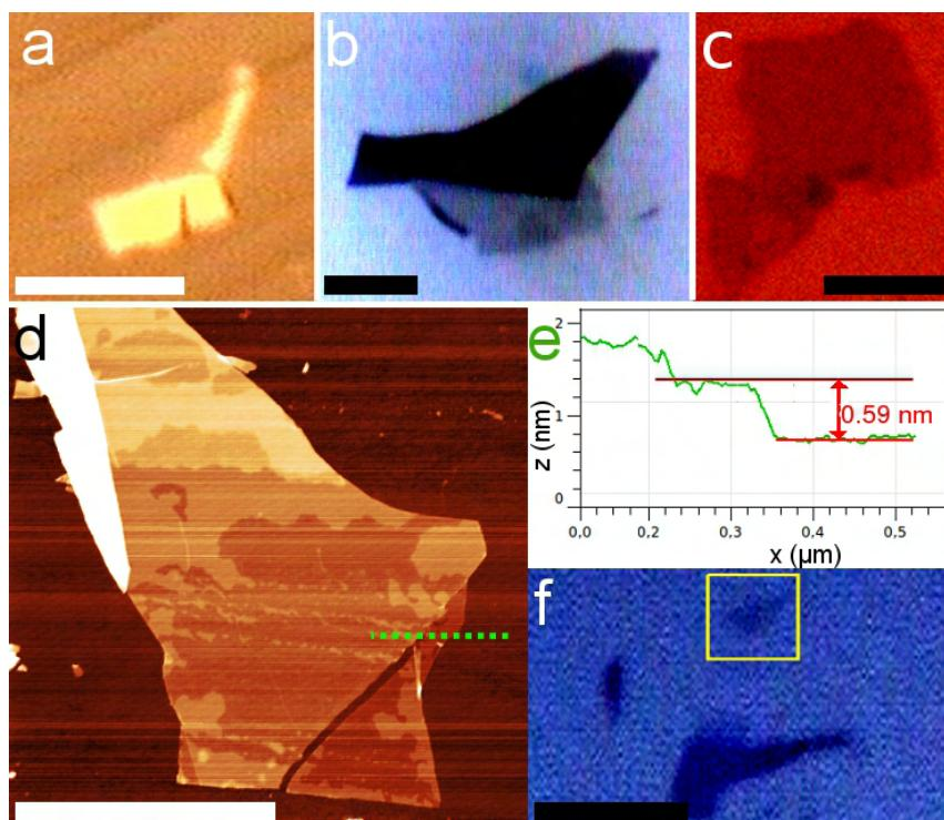
**Figure 3.12.** Optical images of micromechanically exfoliated graphene deposited on (a) KBr, (b) mica and (c) alumina. (d) AFM image of a mono or bi layer graphene on mica. Vertical color scale is 10 nm (e) cross section along the green dashed line in (d). (f) optical image of the flake shown in (d). Scale bars are (a)(b)(c)(f), 10 μm and (d) 1 μm.
