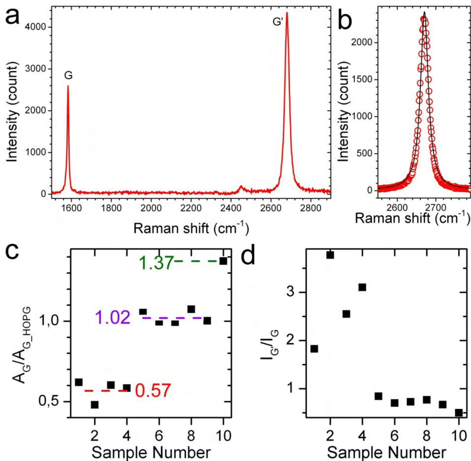
**Figure 3.5.** (a) Raman spectrum of a graphene monolayer supported by a silicon/silicon oxide substrate. The two main peaks of graphene (G and G') are labeled. (b) is a Raman spectrum of a graphene monolayer G'-peak (red circles) and its Lorentzian fit (solid black line). (c) is a plot of the G-peak integrated intensity of graphene flakes normalized by the G-peak integrated intensity of a freshly cleaved HOPG. (d) is the  $I_{G'}/I_G$  ratio for several graphene flakes.
