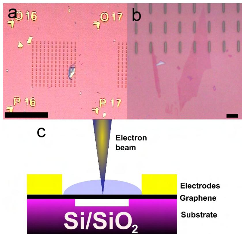
**Figure 5.9.** (a) and (b) Optical image of a  $\text{Si}/\text{SiO}_2$  substrates with pools, graphene has been deposited by micromechanical exfoliation. (b) Schematic view of a  $\text{Si}/\text{SiO}_2$  substrate with pools. A locally suspended graphene flake connected with metallic electrodes is cut by water assisted EBIE. Scale bar are (a)  $100 \mu\text{m}$  and (b)  $5 \mu\text{m}$ .
