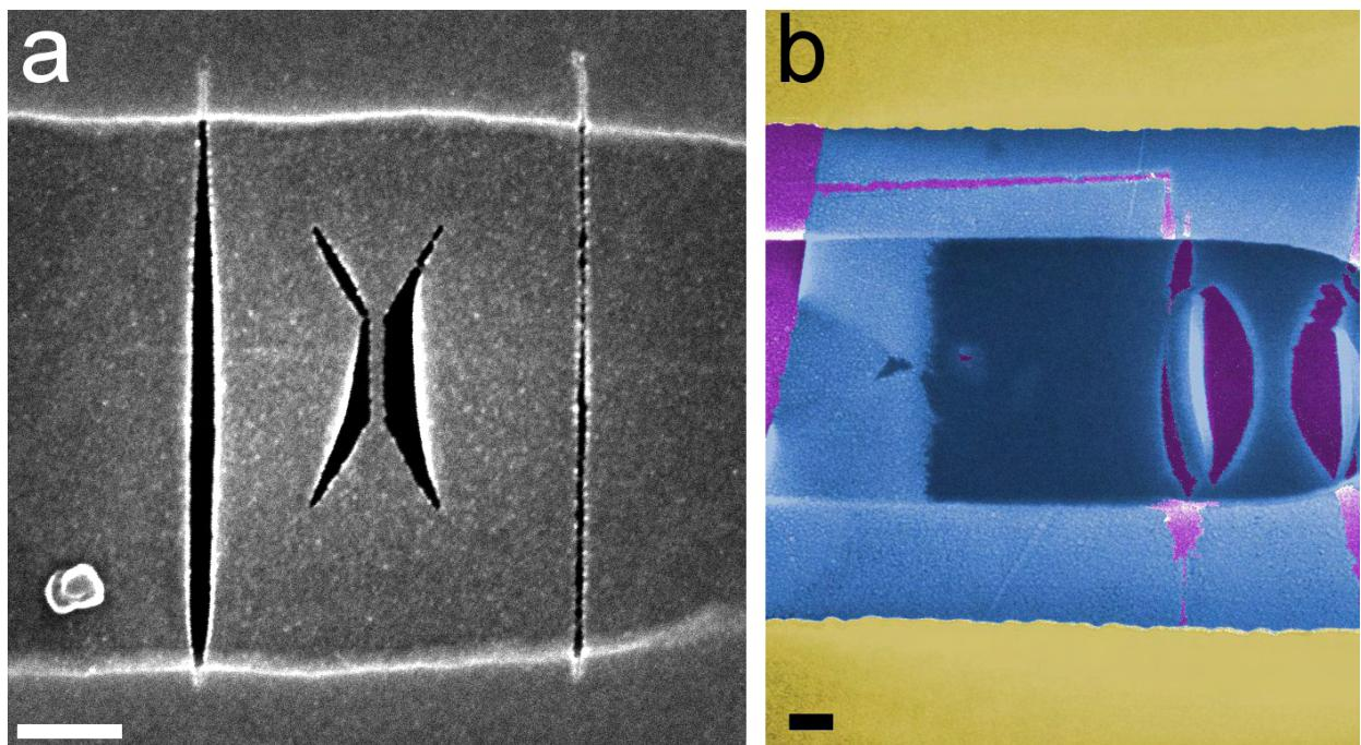
**Figure 5.18.** (a) SEM image of a 30x200 nm graphene ribbon etched by water assisted EBIE on a locally suspended graphene. Electronic dose was  $2 \times 10^{-2} \text{ C.m}^{-1}$  (b) Graphene nano-ribbon etched by EBIE and contacted by metallic electrodes. Colorized SEM image of metallic leads (yellow-brown), supported (blue), suspended graphene (dark blue) and silica surface (violet). Acceleration tension 20 kV. Scale bars are 200 nm.
