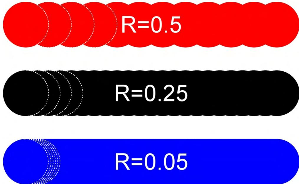
**Figure 4.9.** Comparison between several pitch factor values. The disks represent holes created by a spot mode EBIE. The disks are then spaced by 1/2, 1/4 and 1/20 of the diameter. This simulates an EBIE etch following a line with a pitch factor of  $R=0.5$  (red disks); 0.25 (black disks) and 0.05 (blue disks).
