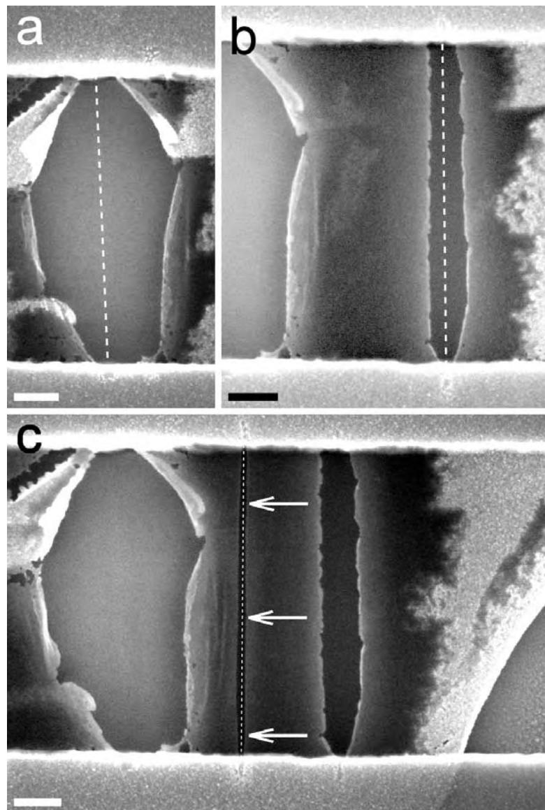
**Figure 5.15.** SEM images of a series of EBIE cuts on locally suspended graphene. All the cuts are made by water assisted EBIE with an electronic dose of  $9 \times 10^{-2} \text{ C.m}^{-1}$  and a voltage acceleration of 20 kV. The first cut is shown in (a). The second cut is done at the right of the first cut, visible in (b). White arrows show the third cut, visible in (c) which has been done between the two previous cuts. Scale bar are 200 nm.
