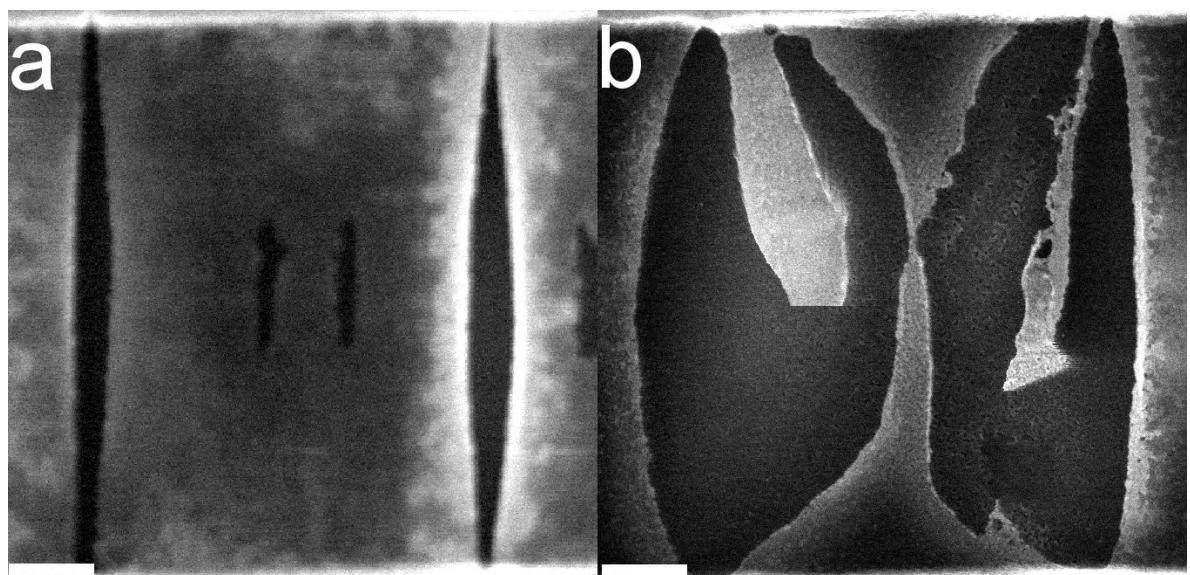
**Figure 5.13.** Suspended graphene nanoribbon. (a): a 150 nm wide ribbon. Finishing the ribbon shown in (a) by water and xenon difluoride assisted EBIE, (b) is a SEM image of a ribbon with two funnels. The ribbon is 60 to 80 nm in width. There is a constriction of 60 nm long and 15 nm wide. Scale bars are 200 nm.
