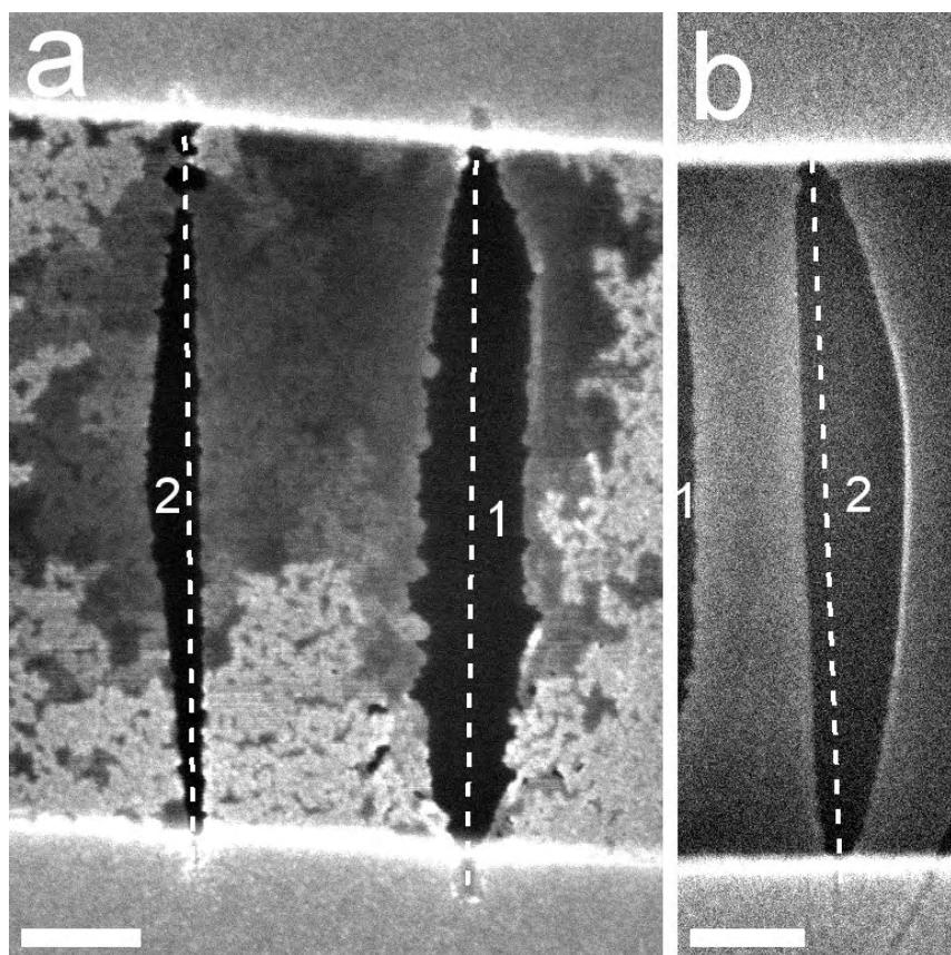
**Figure 5.16.** Asymmetric EBIE cut. SEM images of water assisted EBIE cuts on locally suspended graphene. The numbers on images indicates the order of etching. Electronic doses were (a)  $6 \times 10^2 \text{ C.m}^{-2}$  and (b)  $3 \times 10^2 \text{ C.m}^{-2}$ . In both images acceleration tension was 20 kV. Scale bars are 200 nm.
