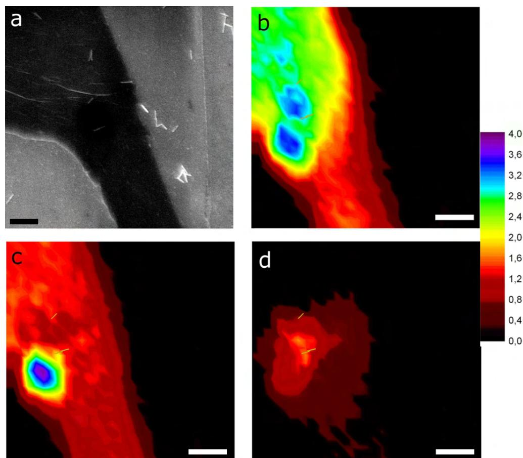
**Figure 3.7.** Raman signal of graphene enhanced by gold nanorods.. (a) A SEM image of a graphene flake deposited on gold nanorods. Raman map of the intensity of the (b)G peak, (c) G'-peak and (d) D peak at 532 nm of excitation wavelength of the same graphene flake.. Color scale bar is normalized by the second order Raman peak of the Si [100]. Scale bars are 1  $\mu$ m
