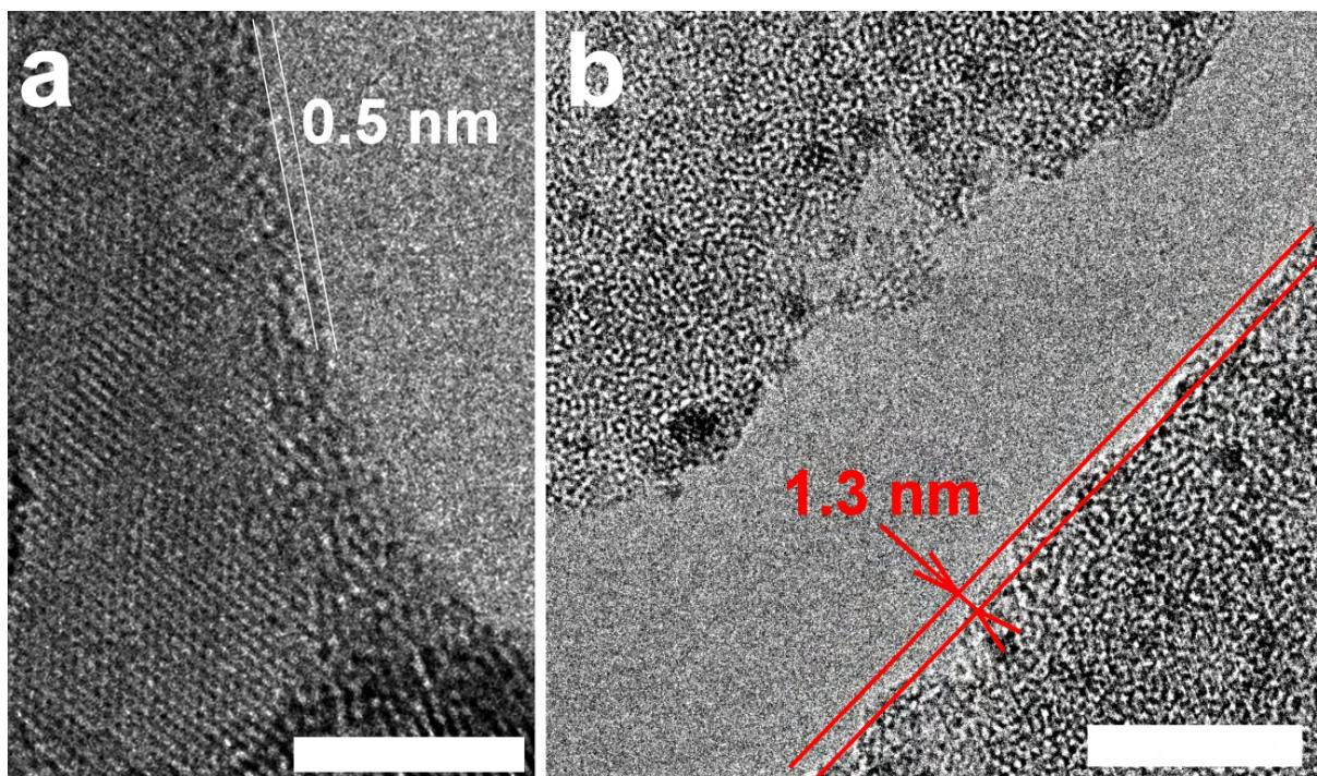
**Figure 4.16.** Edge roughness. The maximum edge roughness defined as the distance between two parallel lines (red) in which fit the edge. TEM operated at 100 kV. Scale bars are 10 nm.
