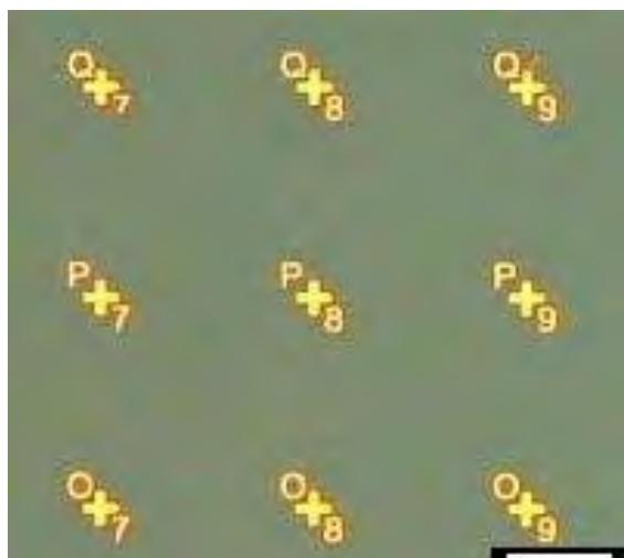
**Figure 2.1:** Optical image of a Si/SiO<sub>2</sub> substrate with photolithography pre-patterned numbered metal crosses. Scale bar is 100 µm.
