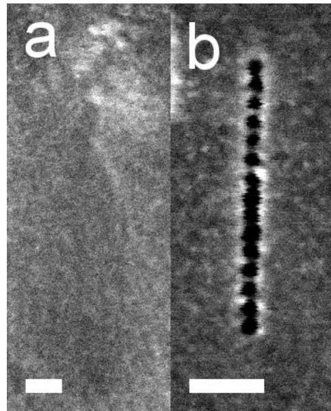
**Figure 4.6.** Evidence for gas assisted EBIE on graphene. SEM images of two series of irradiations (a) without water vapor and (b) with water vapor. Electronic doses per holes are  $20 \text{ C.mm}^2$  for (a) and  $4 \text{ C.mm}^2$  for (b). The width of the cut is 12 nm. Scale bar: 50 nm.
