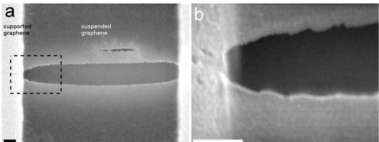
**Figure 5.14.** (a) SEM image of graphene suspended over a pool of a Si/SiO<sub>2</sub> substrate. It has been etched by water assisted EBIE. The acceleration tension was 20 kV and the electronic dose  $9 \times 10^{-2} \text{ C.m}^{-1}$ . (b) is a zoom of the black dashed square in (a). Scale bars: 100 nm.
