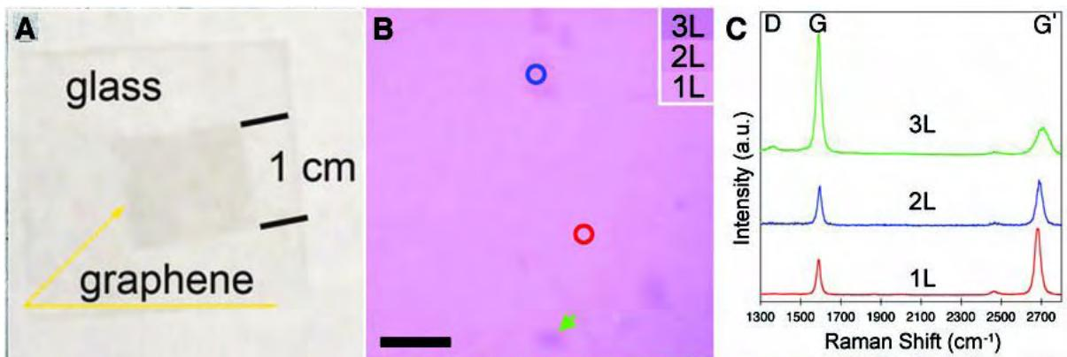
**Figure 1.6.** CVD graphene grown on copper foil and transferred on (a): a glass slide or (b): a Si/SiO<sub>2</sub> substrate. (c) Raman spectrum is taken on the blue and red circle and on the flake shown by green arrow. Scale bar is  $5 \mu\text{m}$ . adapted from [56].
