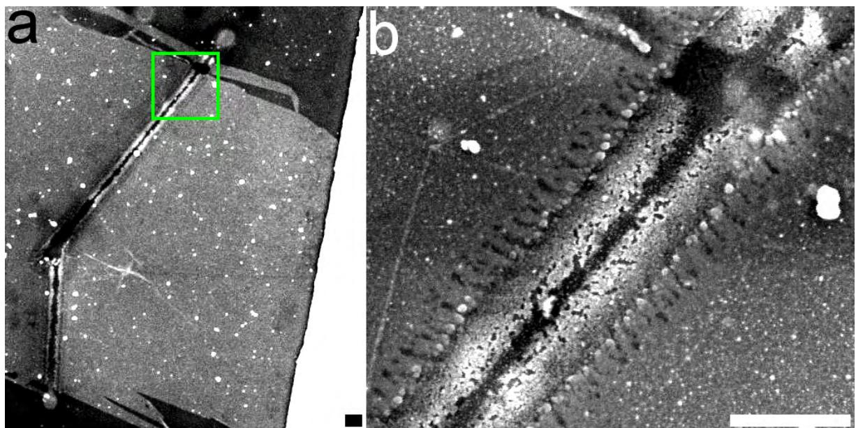
**Figure 5.8.** EBIE etching of graphene on  $\text{SiO}_2$ . (a) is a SEM image of a graphene flake supported on a  $\text{Si}/\text{SiO}_2$  substrate. An EBIE trench has been performed on it, the zoom of the green square is visible in the b) image. Water vapor was injected in the SEM chamber acceleration tension was 20 kV and dose,  $0.11 \text{ C.m}^{-2}$ . Scale bars are 500 nm.
