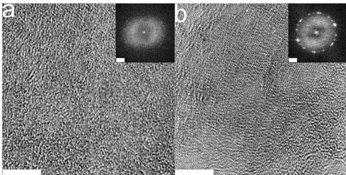
**Figure 4.21.** SACTEM images of a FLG on a copper TEM grid. Inset: FFT of the entire image. The graphene surface is imaged as received in (a) or after an annealing in forming gas ( $\text{Ar}/\text{H}_2$  300/75  $\text{cm}^3.\text{min}^{-1}$ ) at 400°C during 4h in (b). Scale bars: 5 nm for mains images and 2 nm $^{-1}$  for insets.
