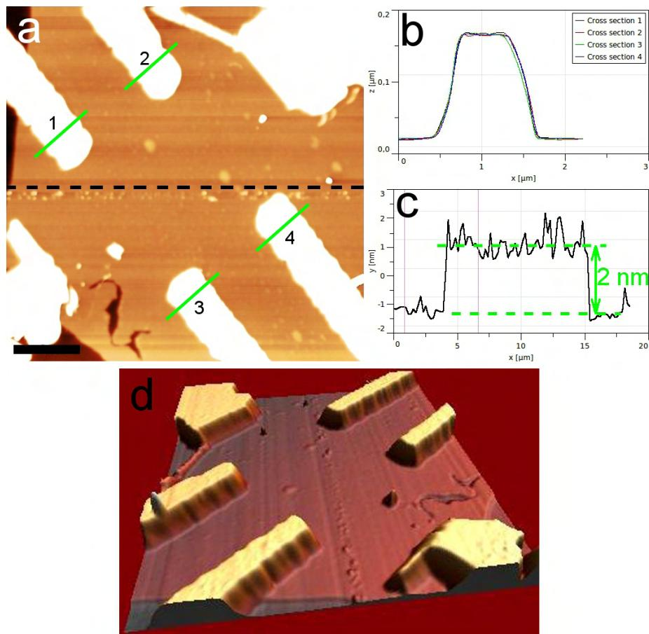
**Figure 5.4.** Electrodes deposited on a graphene flake by the stencil technique. (a) AFM image of Al electrodes deposited on a FLG flake by the stencil technique. (b) AFM cross section of the electrodes along the green lines in image (a). (c) Cross section of the graphene flakes of an AFM image taken before electrodes deposition (not shown). (d) is a 3D view of (a). Scale bar: 2  $\mu\text{m}$ . vertical color scale: 40 nm.
