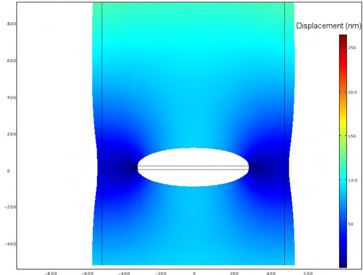
**Figure 5.17.** Simulated displacement of a cut in a strained film. X and Y axis are in nm, black solid line is the contour of the non strained film. Color scale represents the displacement of the loaded film.
