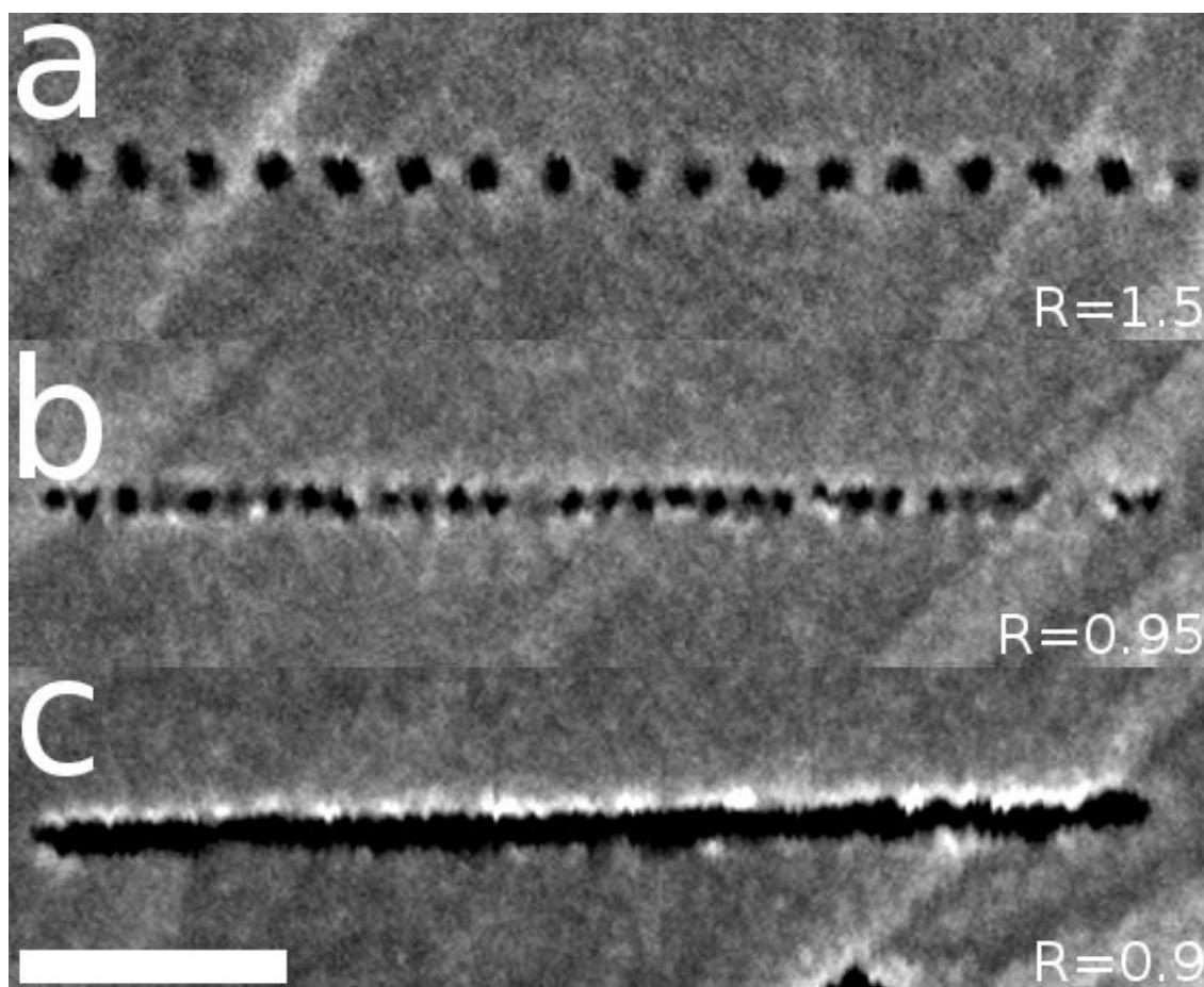
**Figure 4.8.** SEM images for EBIE patterns etched in a suspended graphene for pitch factor (a)  $R > 1$  lead to a series of separated spots with a diameter  $\phi = 15 \text{ nm}$ . (b)  $R \sim 1$  corresponds to tangent spots. (c) Continuous etched line is obtained for  $R < 1$ . Scale bars are 100 nm.
