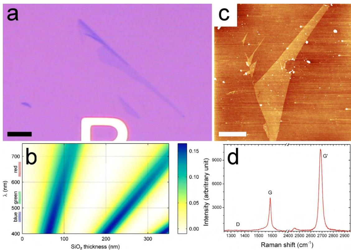
**Figure 1.5.** Identification of graphene (a) Optical image of a graphene flake deposited on a Si/SiO<sub>2</sub> substrate with an oxide thickness of 285 nm. (b) Graphene monolayer contrast with respect to the silica as a function of wavelength and SiO<sub>2</sub> thickness, adapted from [17]. (c) AFM image of a graphene flake. (d) Raman spectrum of a micromechanically exfoliated graphene monolayer. Vertical scale color: 15 nm. Scale bars: 10  $\mu\text{m}$ .
