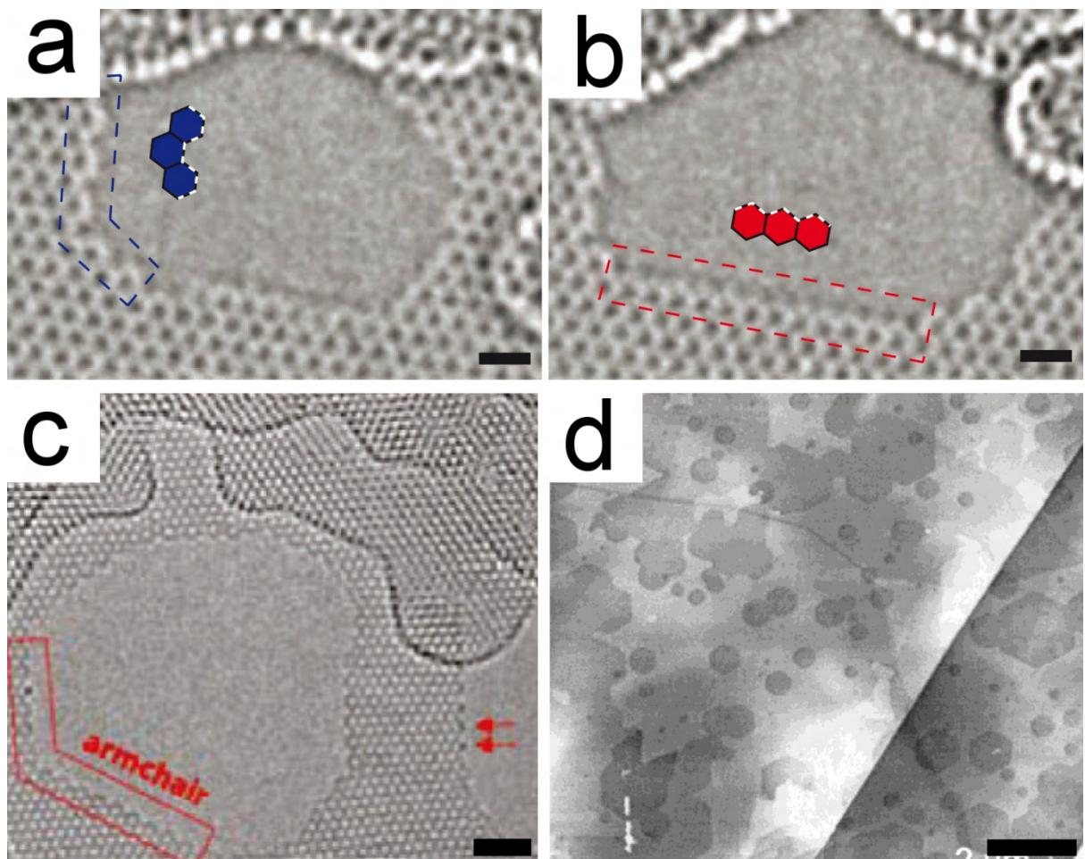
**Figure 1.10.** (a) Armchair and (b) zigzag configuration of carbon atoms at the edge of a hole in graphene. (c) AGNR made from a single layer of graphene. (d) STM image of geometrical flat bottomed microholes in HOPG after electron beam exposure. Adapted from: (a) and (b) [90]; (c) [91] (d) [92]. Scale bars: (a) and (b) 0.5 nm, (c) 1 nm and (d) 2  $\mu$ m.
