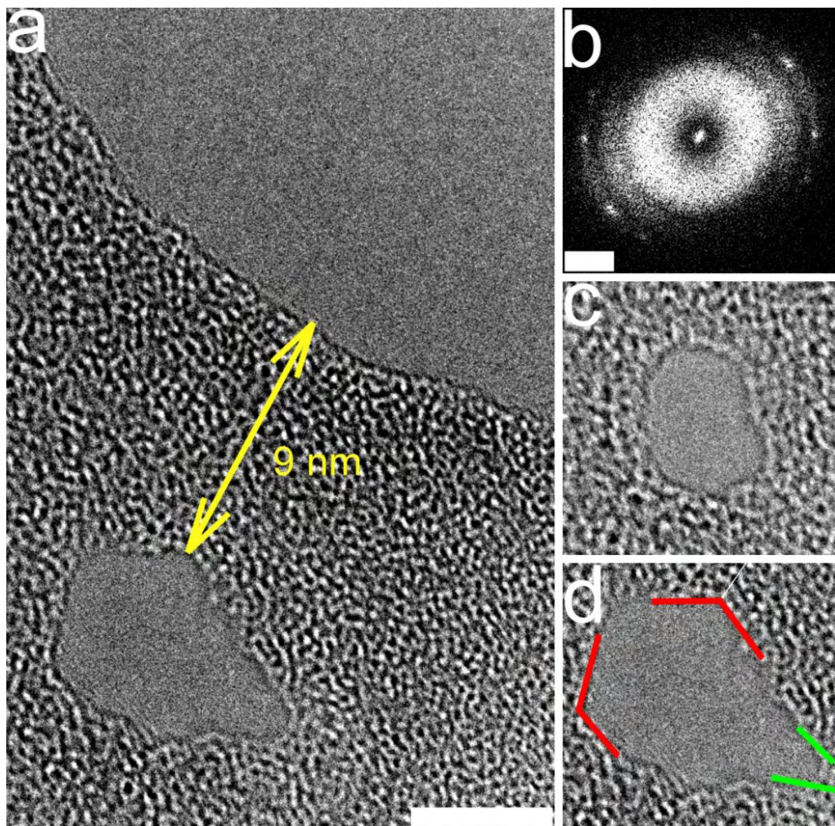
**Figure 4.18.** (a) is a SACTEM image of an EBIE cut. The EBIE cut is in the upper right corner of the image. A hole created near the EBIE cut by focusing the TEM beam and enlarged with a spread beam is visible at about 9 nm from the EBIE cut. (b) FFT of the image (a). (c) hole before it enlargement. (d) hole after enlargement  $120^\circ$  (red) and  $30^\circ$  (green) edges are shown. Scale bar are (a), (c) and (d) 5 nm; (b)  $2 \text{ nm}^{-1}$ .
