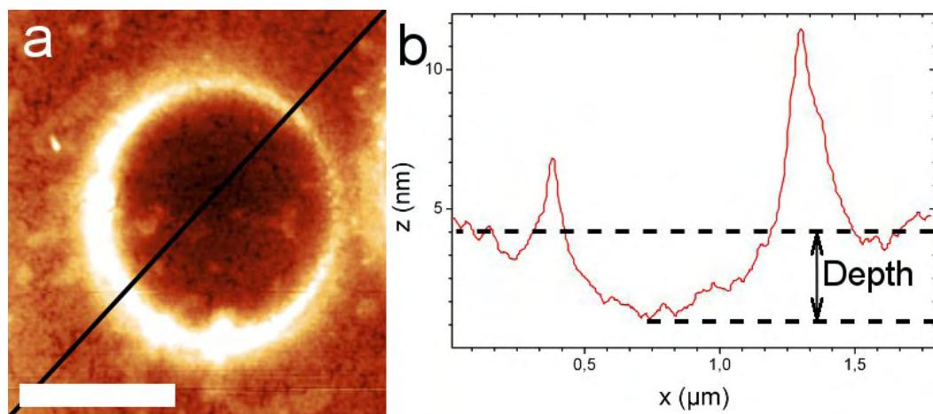
**Figure 5.5.** Electron irradiation in spot mode of a supported FLG on  $\text{SiO}_2$ . (a): AFM Image of a FLG deposited on a silica surface. The irradiation has been made in the center of the image with a dose of  $50 \text{ C.mm}^{-2}$  and an acceleration tension of 5 kV, no gas was injected. (b) is a cross section of the black line in (a), the depth of the hole is shown. Vertical color scale: 10 nm. Scale bar: 500 nm.
