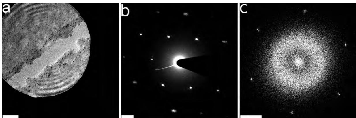
**Figure 4.17.** Diffraction and FFT of areas close to an EBIE cut. (a) TEM images of an EBIE cut. the central disk is the selected area for the electron diffraction of (b). (b) SAED of the EBIE cut shown in (a). (c) FFT of an image of the cut shown in (a). Scale bars are (a) 20 nm, (b) and (c) 2 nm<sup>-1</sup>.
