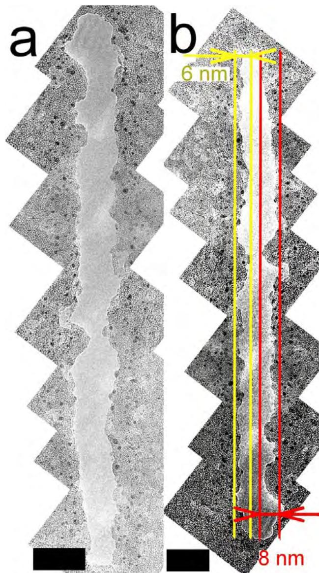
**Figure 4.20.** Roughness analysis. (a) Reconstructed SACTEM image of a long EBIE cut. (b) Is the reproduction of (a), two couples of parallel lines were added to highlight the left (yellow lines) and right (red lines) edges roughness. TEM operated at 100 kV. Scale bars are 20 nm.
