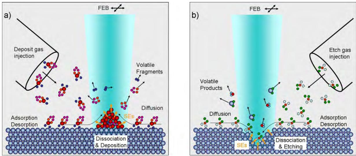
**Figure 4.5.** Schematics illustrating the processes involved in gas assisted electron beam induced deposition (a) and etching (b). Adapted from [27].
