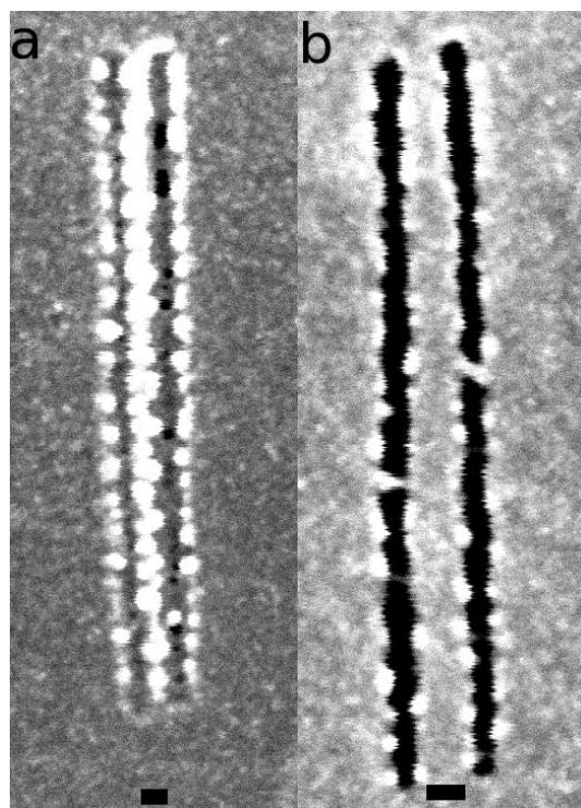
**Figure 4.14.** EBIE etching on thick and thin FLG. EBIE cut in Figure (a) has been done on a thick FLG, the electronic dose was  $1.1 \times 10^{-1} \text{ C.m}^{-1}$ . Figure (b) is an EBIE trench performed with a dose of  $4.5 \times 10^{-2} \text{ C.m}^{-1}$  on a thinner graphite than (a). Electron beam was 20 kV and water vapor was used. Scale bars are 20 nm.
