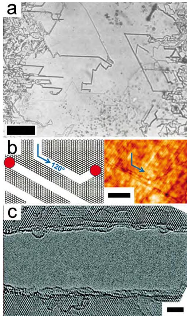
**Figure 1.11.** (a) Optical image of straight trenches formed by catalytic hydrogenation of graphite. adapted from [100]. (b) Drawing and AFM image of a ribbon created by a nanoparticle which turns twice, forming two angles of 120°. Adapted from [106]. (c) TEM image of a trench in FLG by a catalytic hydrogenation of graphene. Adapted from [108]. Scale bars: (a) 20  $\mu$ m, (b) 100 nm and (c) 2 nm.
