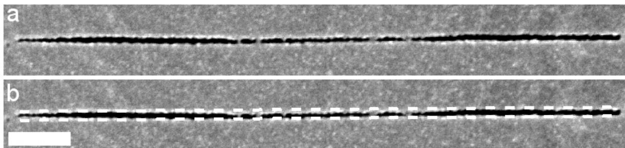
**Figure 4.12.** SEM image of EBIE long cut. (a) is a SEM image of a EBIE cut performed on graphite. (b) is the same image with two parallel dashed lines separated by 15 nm. Electronic dose was 5.4x10<sup>-2</sup> C.m<sup>-1</sup>, pitch factor was 0.8 and it took 4 min to be etched. Scale bar is 100 nm.
