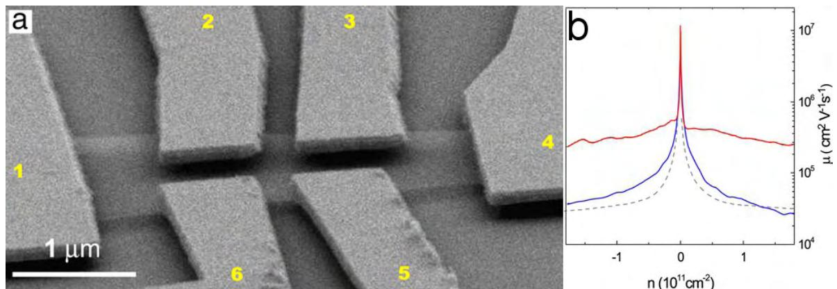
**Figure 1.3.** Suspended graphene device. (a) SEM image of a typical suspended six-probes graphene device taken at  $15^\circ$  with respect to the sample plane. (b) Mobility  $\mu$  as a function of carrier density  $n$  for a suspended graphene before (blue) and after (red) current annealing. Dotted line is the same measurement for the annealed supported sample. Adapted from [11].
