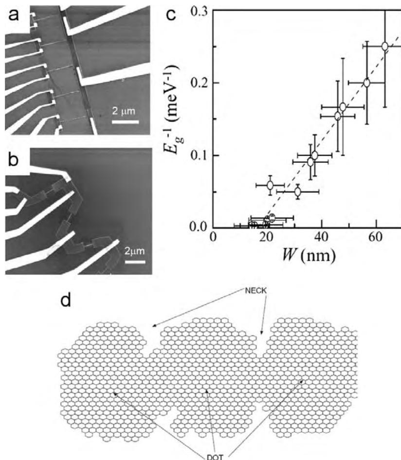
**Figure 1.7.** . (a) SEM image of parallel GNRs with varying width. (b) SEM image of GNR with varying orientations. (c) Inverse of band gap energy versus GNRs width. Dashed line is a linear fit. (a-c) Adapted from [62]. (d) Schematics of a graphene ribbon with a disordered edge leading to the formation of necks and dots along the ribbon.. Adapted from [67].
