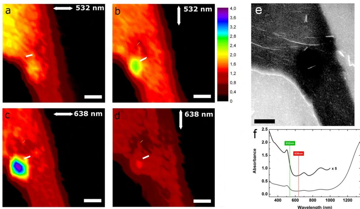
**Figure 3.8.** Polarization and wavelength dependence of the enhancement of the Raman G'-peak of graphene by gold nanorods. (a-d) Raman maps of the G'-peak intensity with (a, c) horizontal polarization and (b, d) vertical polarization. The excitation wavelength are (a, b) 532 nm and (c, d) 638 nm. (e) SEM image of the graphene and nanorods. (f) Absorbance spectrum of gold nanorods. Color scale bar is normalized by the second order Raman peak of the Si [100]. Scale bars are 1  $\mu$ m.
