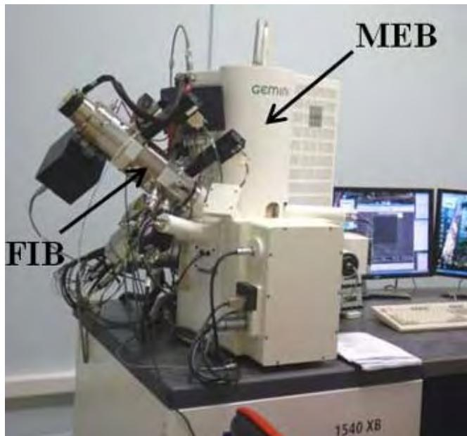
**Figure 2.3.** Zeiss 1540XB FIB-SEM equipped with a GIS.
