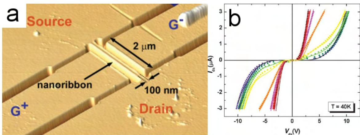
**Figure 1.8.** (a) 3D rendering of an AFM image of a side-gated sub-100 nm wide graphite nanoribbon. (b) I-V characteristics of a  $50 \times 2 \text{ mm}^2$ , FLG ribbon at  $T=40\text{ K}$ . Applied side-gate voltages are 0; 2; 4; 6; 8; 10; 15; 20; 25; and 30 V, displayed in a black-to-red rainbow color scheme. Open circles are experimental data and continuous lines are fits using a 1D quantum dot array model. Adapted from [44].
