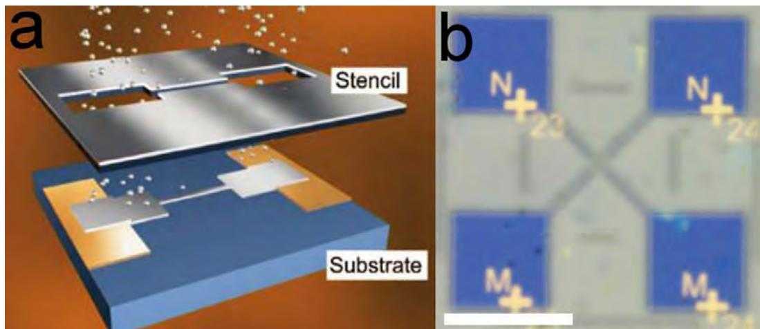
**Figure 5.3.** (a) Schematics illustrating the stencil deposition technique. Adapted from [8]. (b) Optical image of a  $\text{Si}_3\text{N}_4$  membrane positioned onto a substrate. In this case, the membrane is transparent, allowing to see the substrate too. Scale bar, 100  $\mu\text{m}$ .
