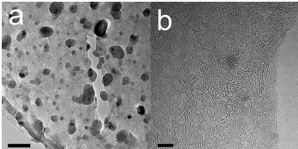
**Figure 4.22.** Metallic particles on annealed graphene. (a) is a TEM image of a graphene grown by CVD on a nickel surface transferred on a copper TEM grid. (b) is a TEM image of a graphene grown by CVD on a copper surface transferred on a gold TEM grid. The samples have been annealed in forming gas at 300°C for 2 h. Scale bars: (a) 30 nm, (b) 4 nm.
