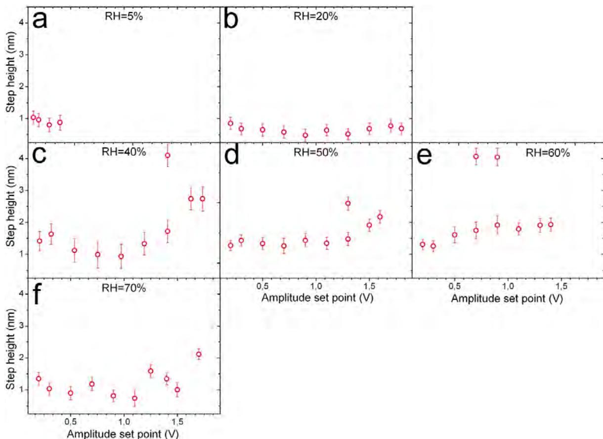
**Figure 3.4.** Apparent height of graphene under AFM imaging versus the amplitude set point for dry regime (a-b); medium humidity regime (c-e) and wet regime (f). RH are (a) 5%, (b) 20%, (c) 40%, (d) RH=50%, (e) RH=60% and (f) RH=70%.
