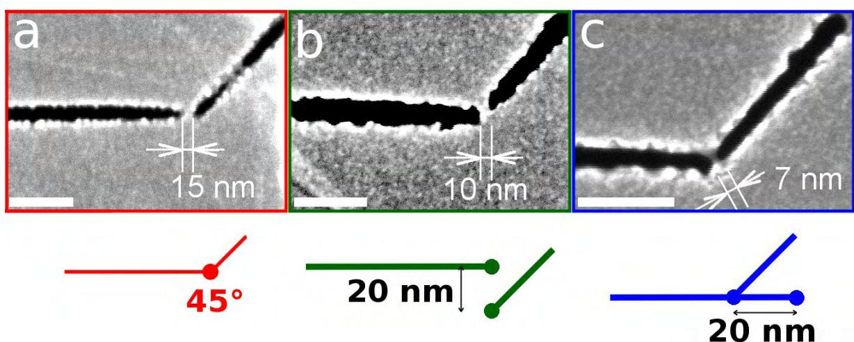
**Figure 4.13.** SEM images of ribbon with funnels. (a), (b) and (c): SEM images of two connected EBIE trench. Schematics of the etching ordered on the EBIE software is shown below each images. Pitch factor and doses are 0.5 and  $8.6 \times 10^{-2} \text{ C.m}^{-1}$ . Scale bars are 100 nm.
