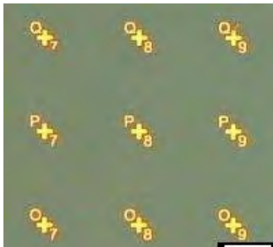
Figure 2.1: Optical image of a Si/SiO 2 substrate with photolithography pre-patterned numbered metal crosses. Scale bar is 100 \mu m.
