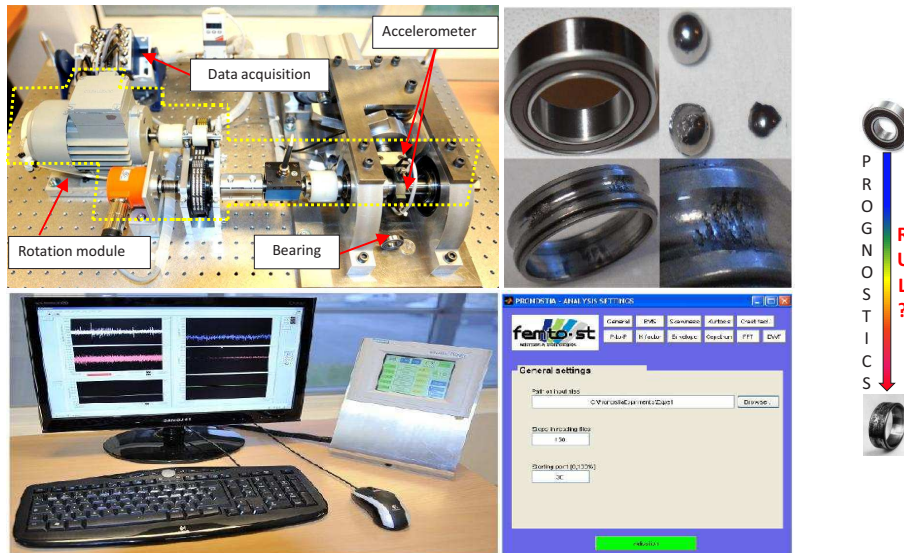
FIGURE 2.8: PRONOSTIA testbed - FEMTO-ST Institute, AS2M department
