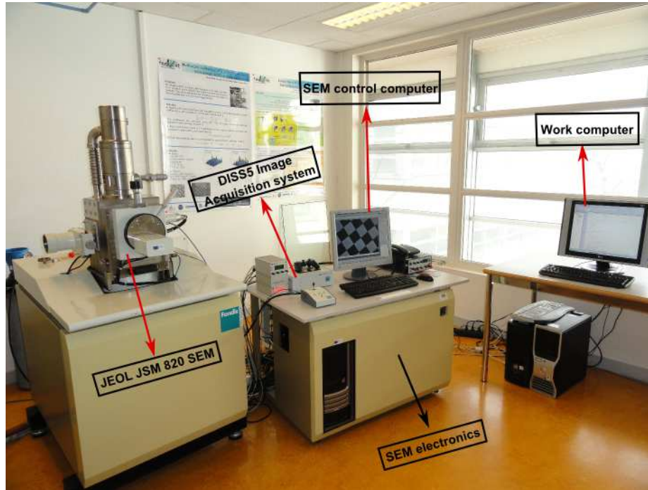
Figure 2.17: Experimental environment showing the hardware set-up.
